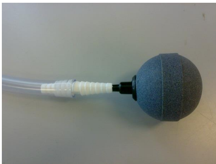
Figure 4-4 Gas diffuser applied in the experiment.
