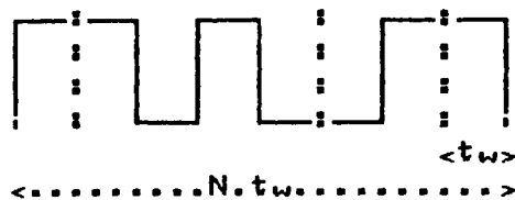
Fig. 3.6 An 8 bit Golay code showing code duration parameters.
