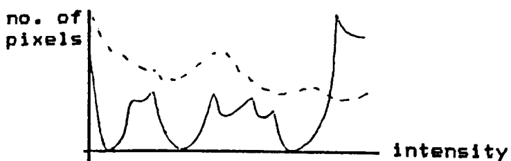
Fig. 6.18 Intensity histogram for threshold determination
