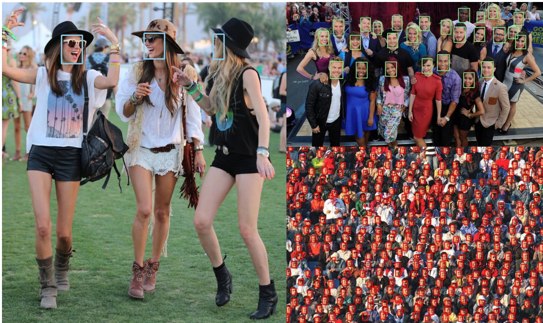
Figure 1.2: Examples of easy, medium and hard faces on WIDER FACE dataset, which are highlighted using blue, green and red boxes, respectively. According to the detection difficulty, which is measured by the average recall of EdgeBox detector [21] with 8,000 proposals per image, faces are split into three subsets: easy, medium and hard. For WIDER FACE dataset, the rates for these three subsets are 92%, 76%, and 34%, respectively.
