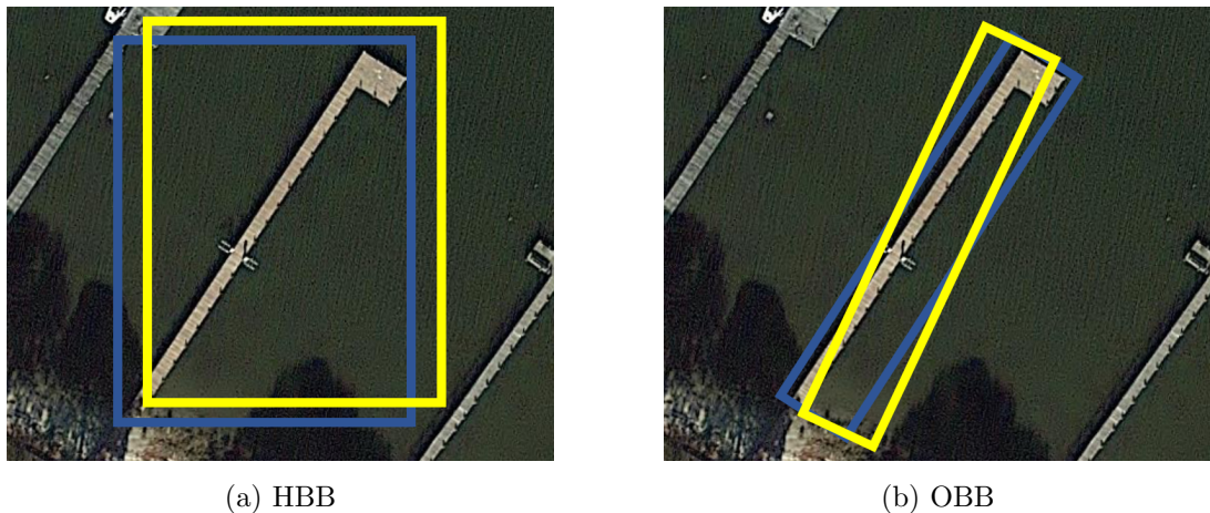
Figure 6.3: Examples of bounding box prediction on HBB (a) and OBB (b). Ground truth bounding boxes are denoted by blue, while predicted bounding boxes are colored by yellow. Only the centre target are labelled for clarity
