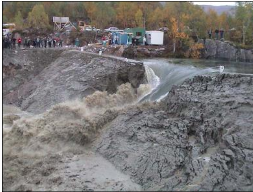
Figure 5-54: Headcut breaks through the crest causing the opening of the breach formation. Predicted embankment profile (a) and photos from the large-scale test (b) and (c)
