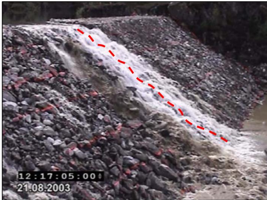
Figure 5-58: Interpretation of the embankment profile after 17 minutes the overflow process of the Test #3
