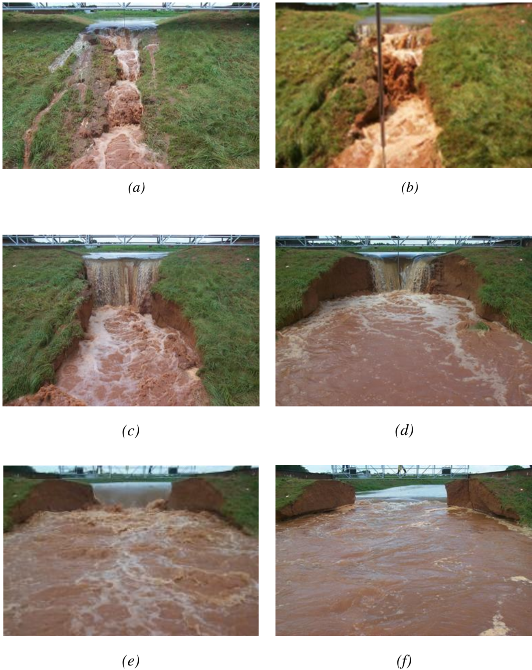
Figure 2-9: Different stages of breach formation observed during field-test experiments on fine-grained embankments. (a) formation of networks of rills and (b) evolution of the initial rills into a multi-stepped profiles in Stage I; (c) headcut backwards migration and transition to Stage II (d) headcut advancement to the crest and transition to Stage III; (e) crest lowering and transition to Stage III; (f) breach widening at Stage IV (G. J. Hanson, K. R. Cook and S. L. Hunt, 2005)
