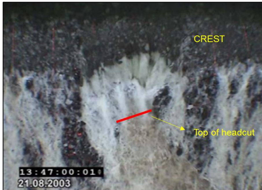
Figure 5-77: IMPACT field test #3 few minutes before breach formation (a) side view; (b) aerial view
