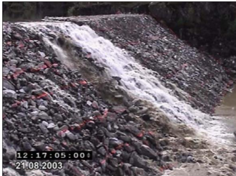
Figure 5-57: Initial phase of breach formation for coarse-grained embankment (a) predicted profile after 10 minutes of overflow; (b) Field test #2 after 7 min of test run; (c) Field test #3 after 17 min from the start of overflow
