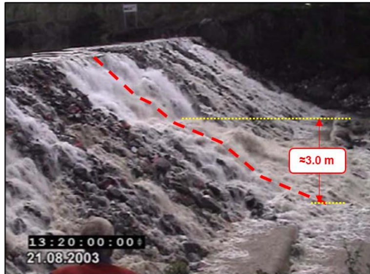
Figure 5-70: Interpretation of the embankment profile observed during the Field Test #3 after 95 min of overflow
