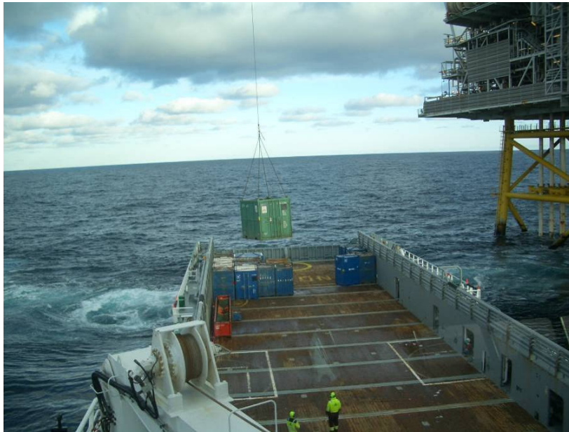
Figure 2.5: DP operation close to offshore installation (view from operator station)
