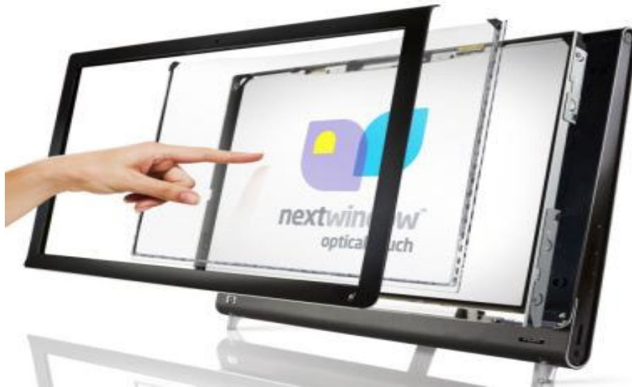
Figure 5.7: Illustrating the layers of NextWindow's 8 optical technology
