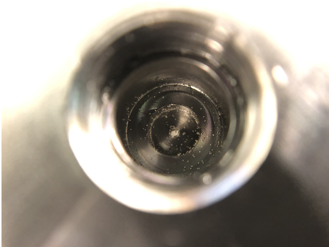
Figure A.3: Particles sitting at the entrance of the dummy filling cell
