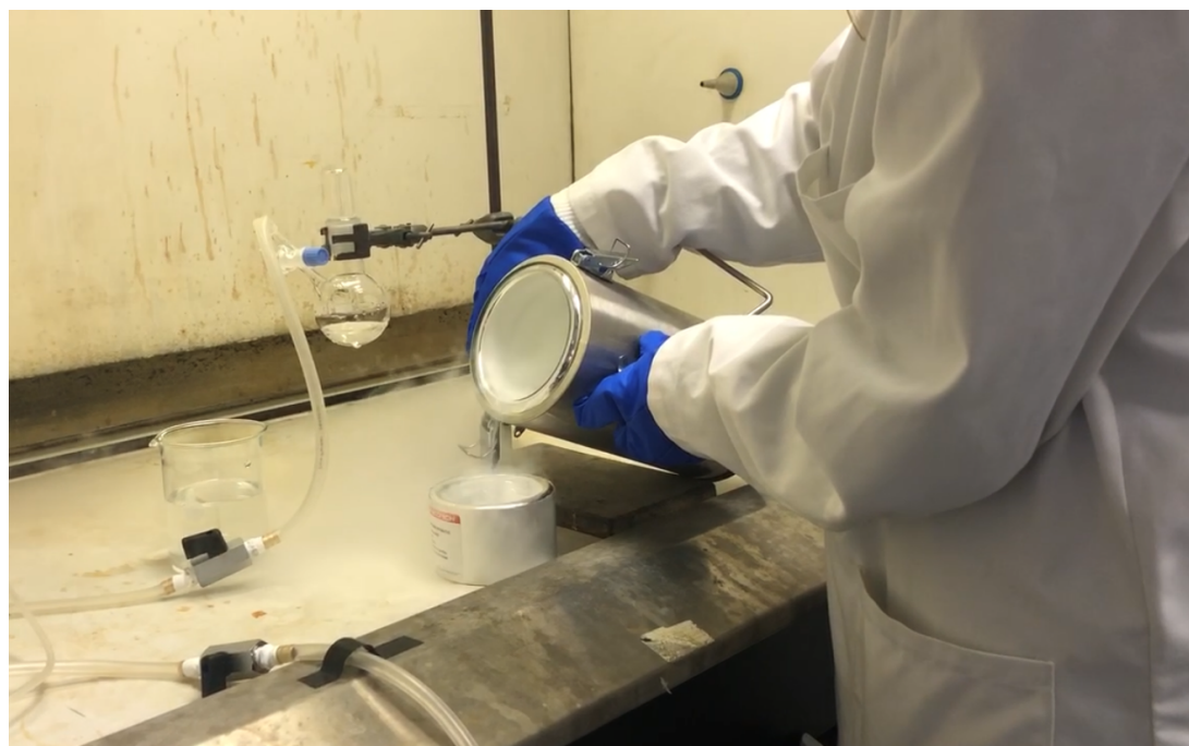
Figure A.9: Liquid nitrogen being poured into dewar for the freezing process
