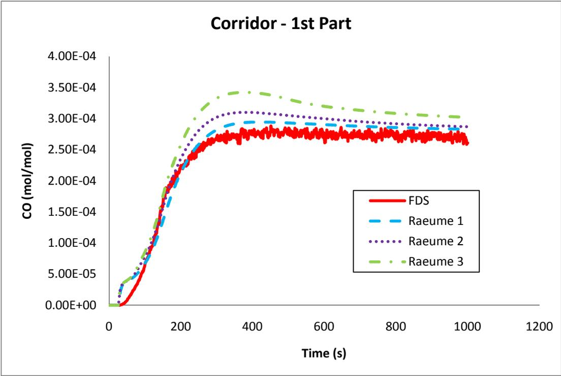
Figure B - 24: Carbon monoxide concentration (mol/mol) in the first part of the corridor.
