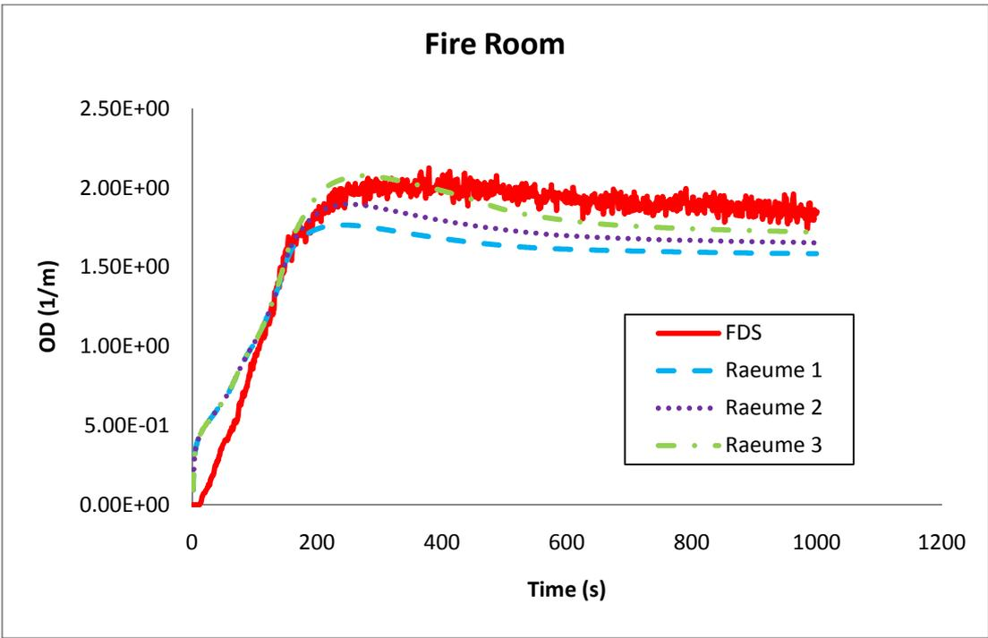
Figure B - 35: Optical density (1/m) in the fire room.
