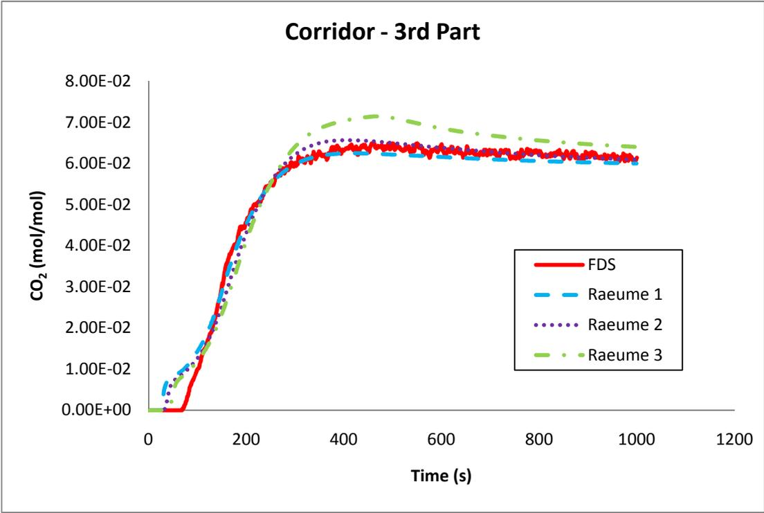
**Figure B - 30: Carbon dioxide concentration (mol/mol) in the third part of the corridor.**
