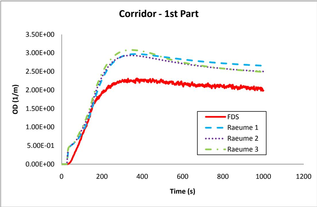
Figure B - 36: Optical density (1/m) in the first part of the corridor.
