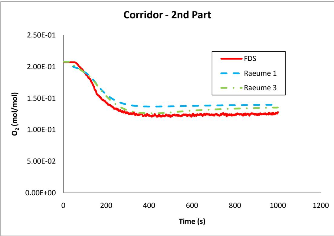
Figure B - 33: Oxygen concentration (mol/mol) in the second part of the corridor.
