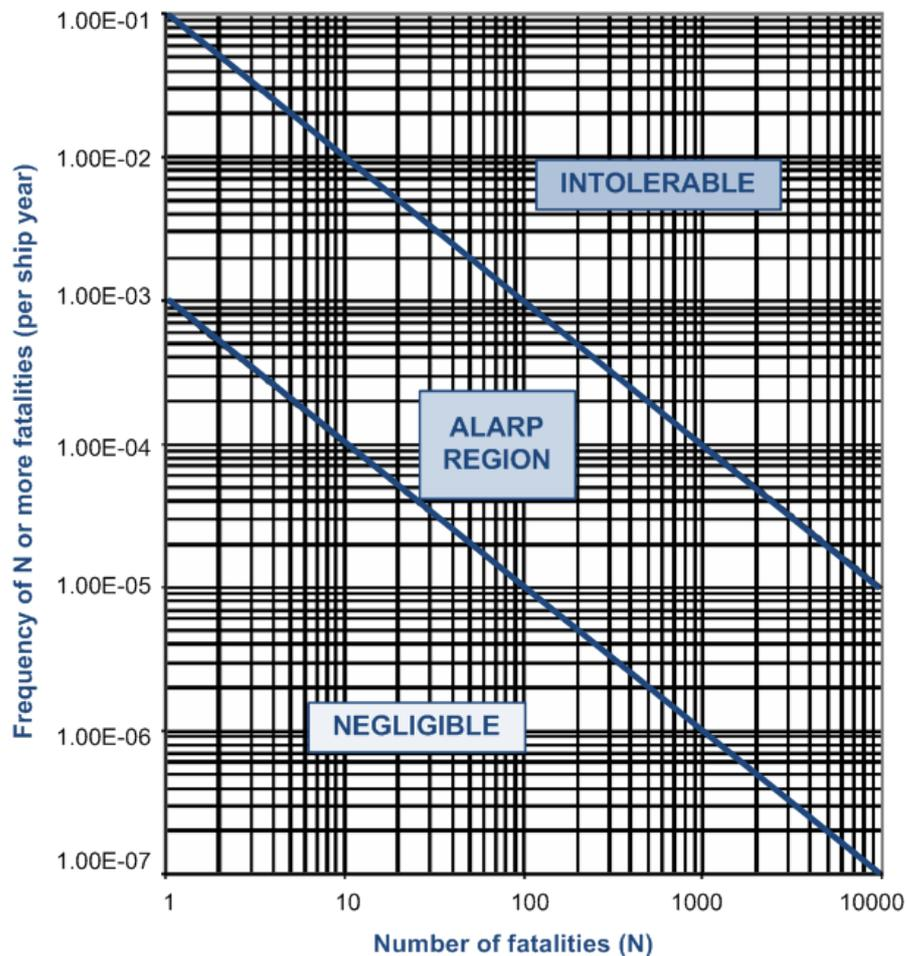
Figure 3-9: Suggested FN curve criteria for ro-ro/passenger ferries; [DNV, 2005]
