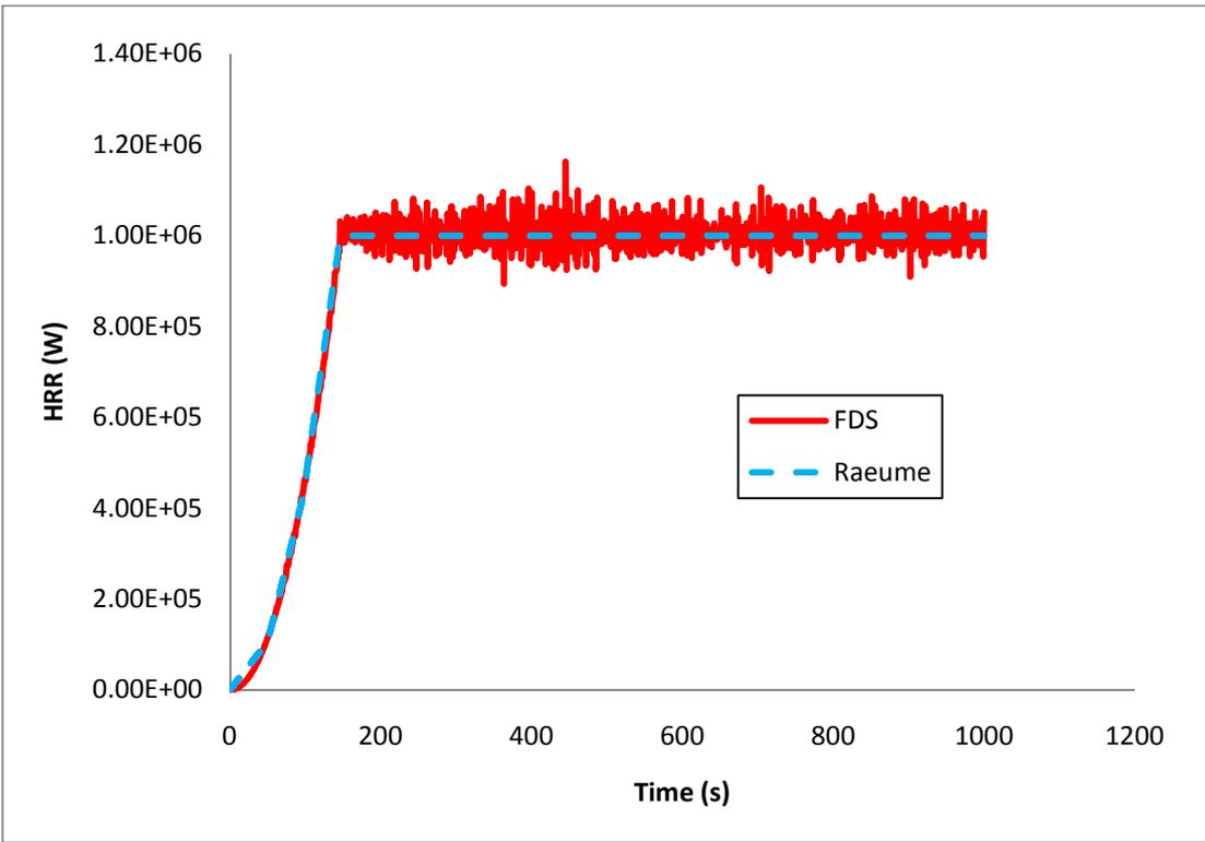
Figure B - 47: Output heat release rate (W) in the fire room.
