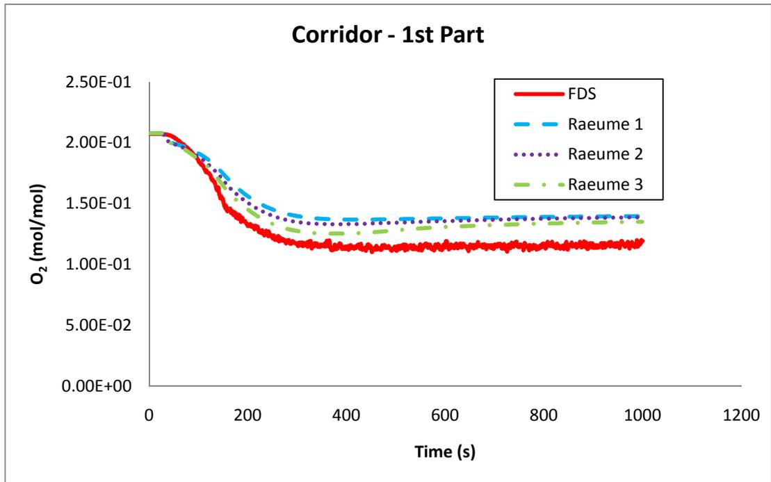
Figure B - 32: Oxygen concentration (mol/mol) in the first part of the corridor.
