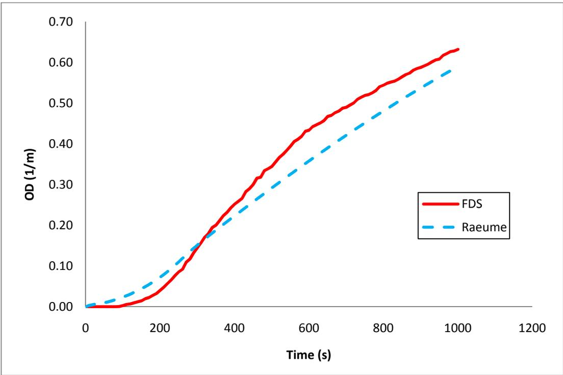
Figure B - 15: Optical density (1/m) in the atrium as predicted by FDS and Raeume.
