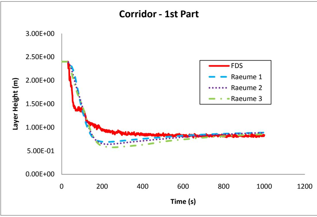
Figure B - 44: Smoke layer interface height (m) in the first part of the corridor.
