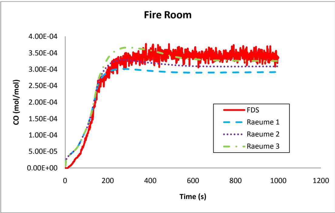
Figure B - 23: Carbon monoxide concentration (mol/mol) in the fire room.
