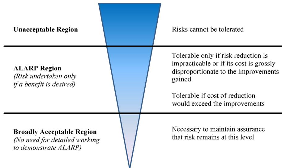
**Figure 3-8: The ALARP concept; [HSE, 1992]**
