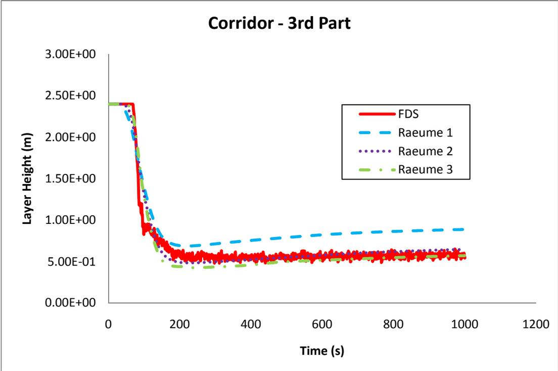
Figure B - 46: Smoke layer interface height (m) in the third part of the corridor.
