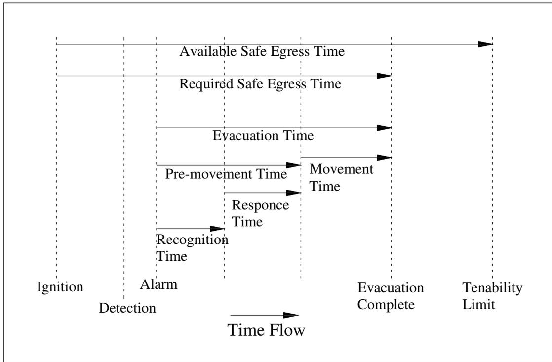
**Figure 4-1: Time lines sequence in fire incidents**
