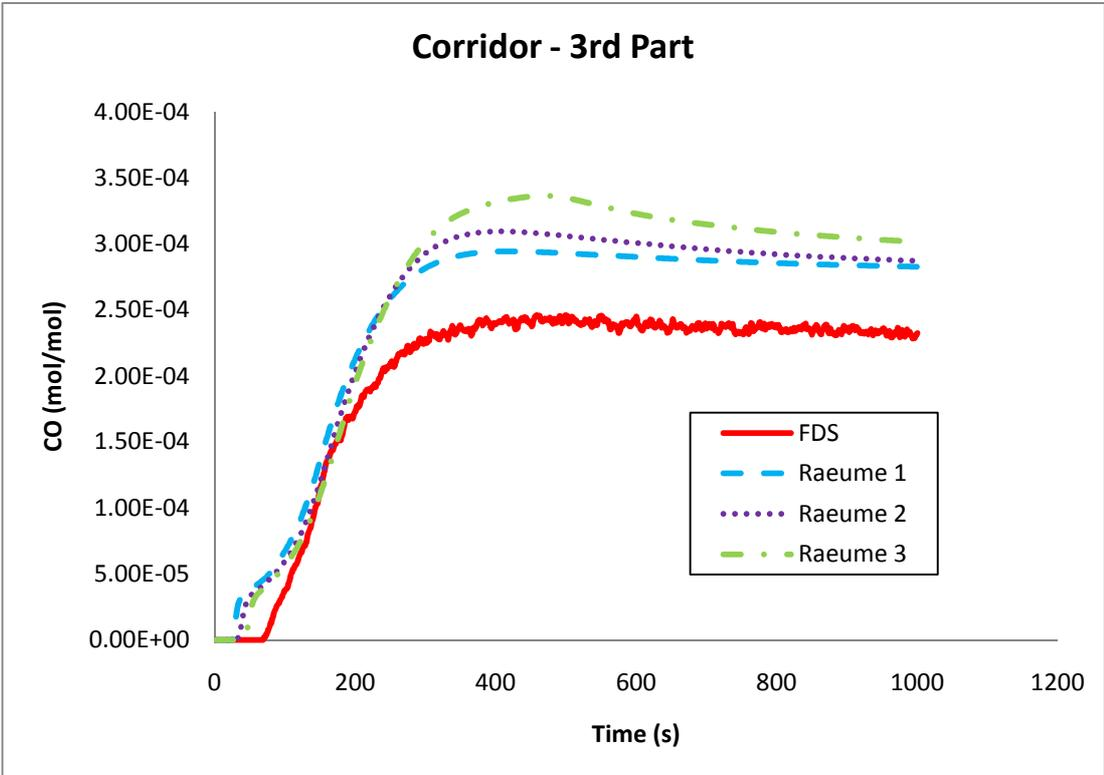
Figure B - 26: Carbon monoxide concentration (mol/mol) in the third part of the corridor.
