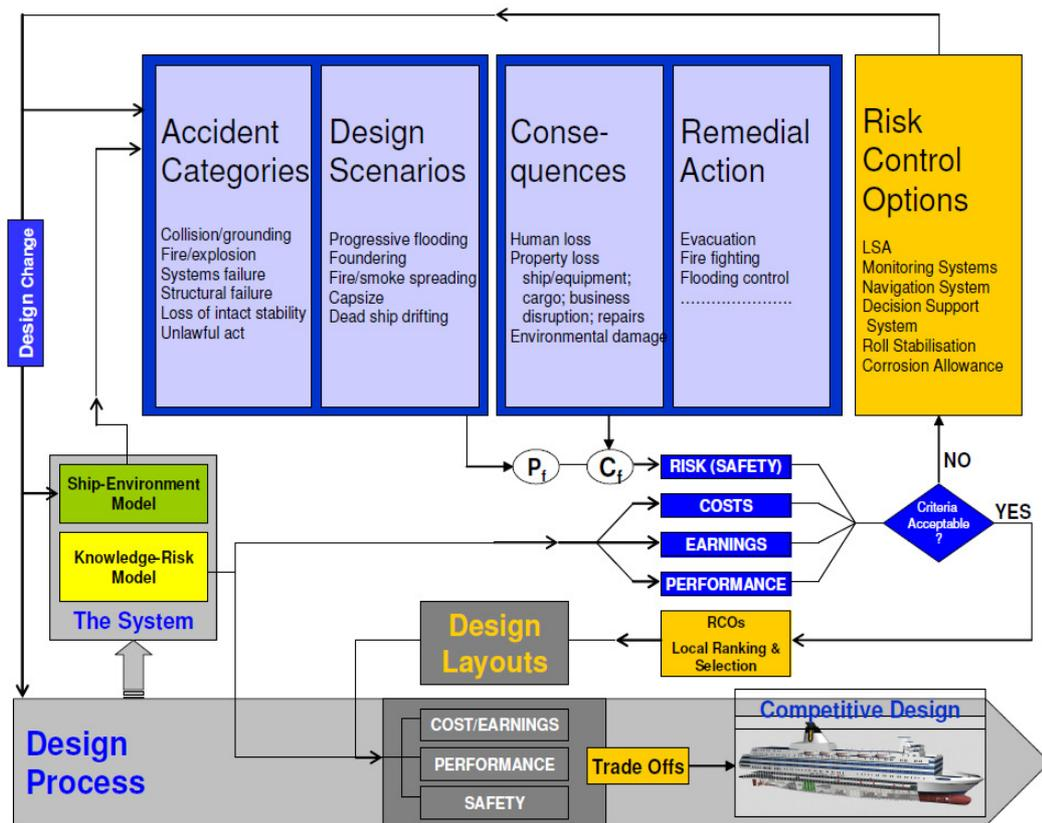
Figure 3-5: Overview of risk-based design (b); reproduced from [Vassalos et al., 2005]
