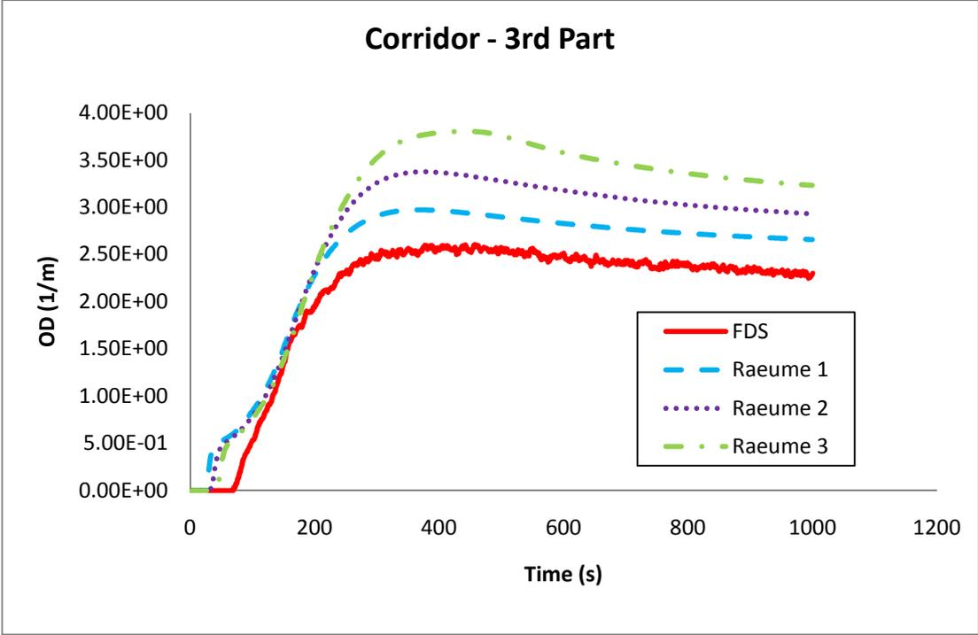
Figure B - 38: Optical density (1/m) in the third part of the corridor.
