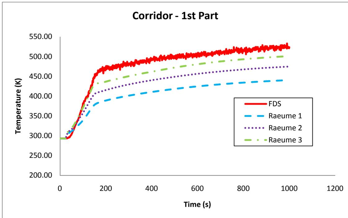
Figure B - 20: Temperature (K) in the first part of the corridor.
