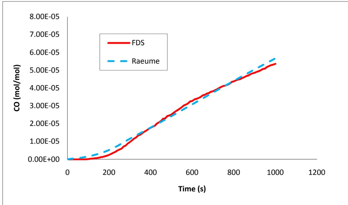
Figure B - 12: Carbon monoxide concentration (mol/mol) in the atrium as predicted by FDS and Raeume.
