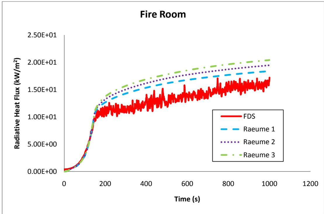
Figure B - 39: Radiative heat flux (kW/m<sup>2</sup>) in the fire room.
