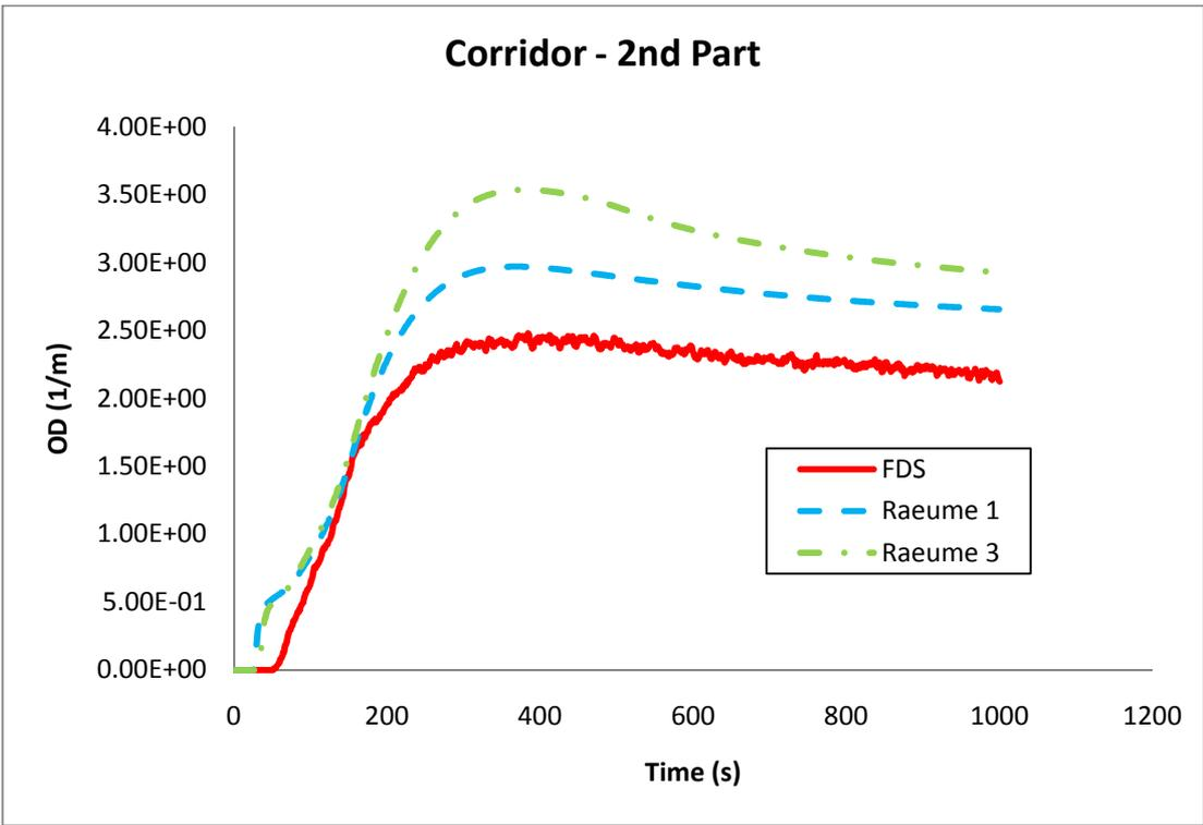
Figure B - 37: Optical density (1/m) in the second part of the corridor.
