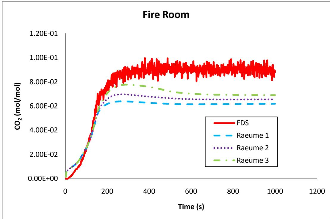
**Figure B - 27: Carbon dioxide concentration (mol/mol) in the fire room.**
