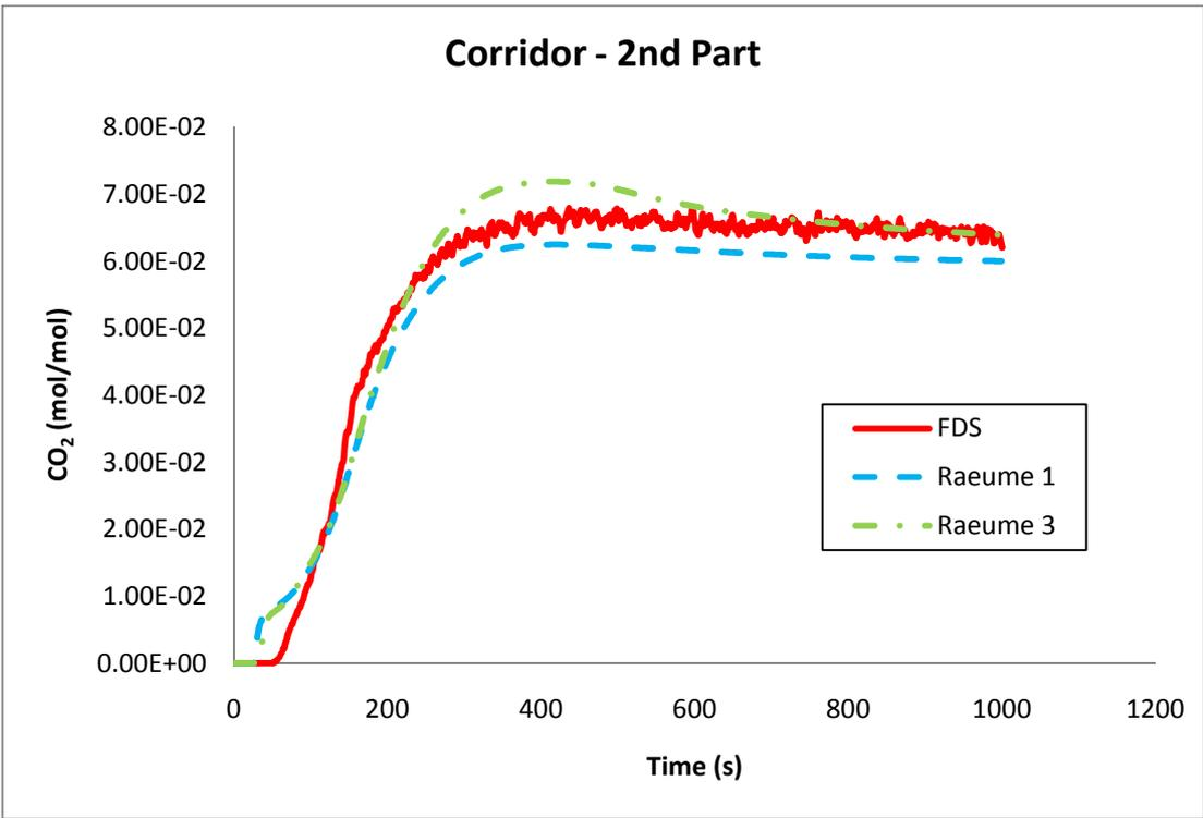
**Figure B - 29: Carbon dioxide concentration (mol/mol) in the second part of the corridor.**
