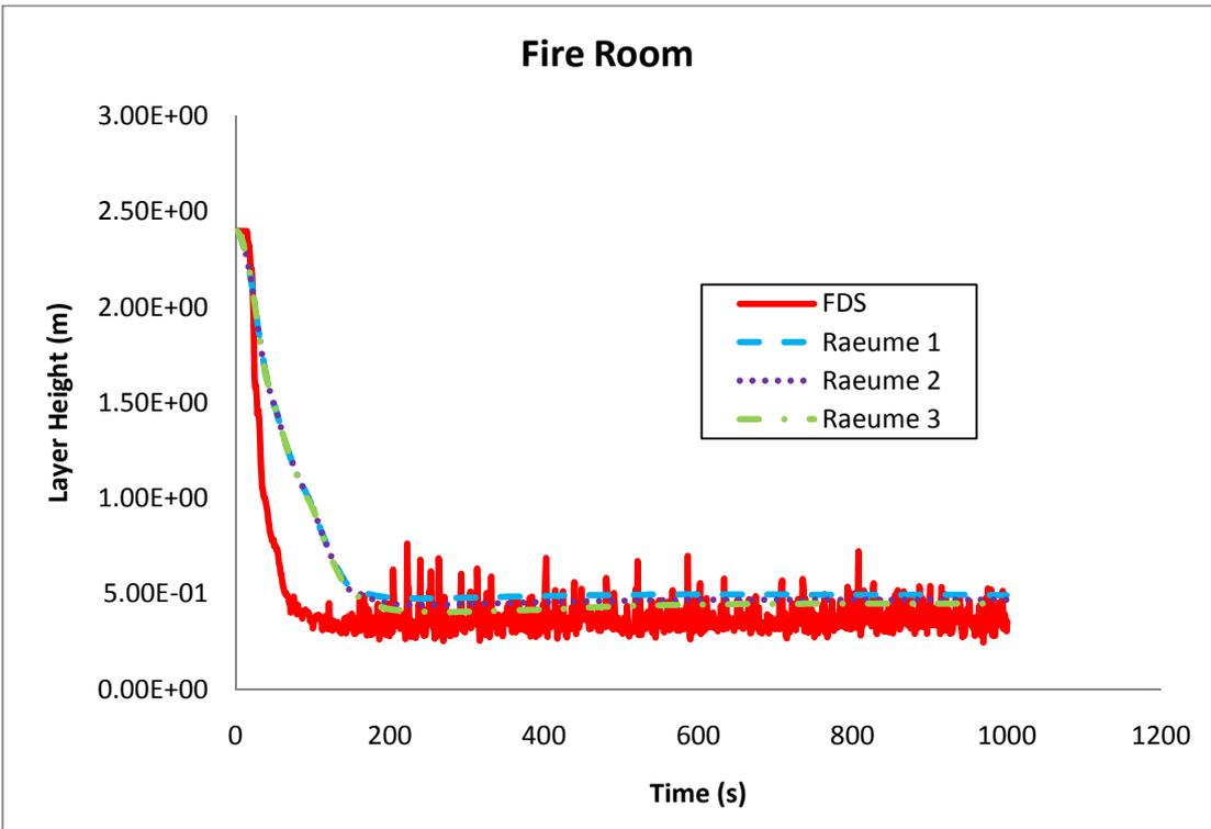
Figure B - 43: Smoke layer interface height (m) in the fire room.
