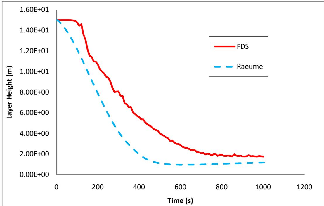
Figure B - 17: Smoke layer interface height (m) in the atrium as predicted by FDS and Raeume.
