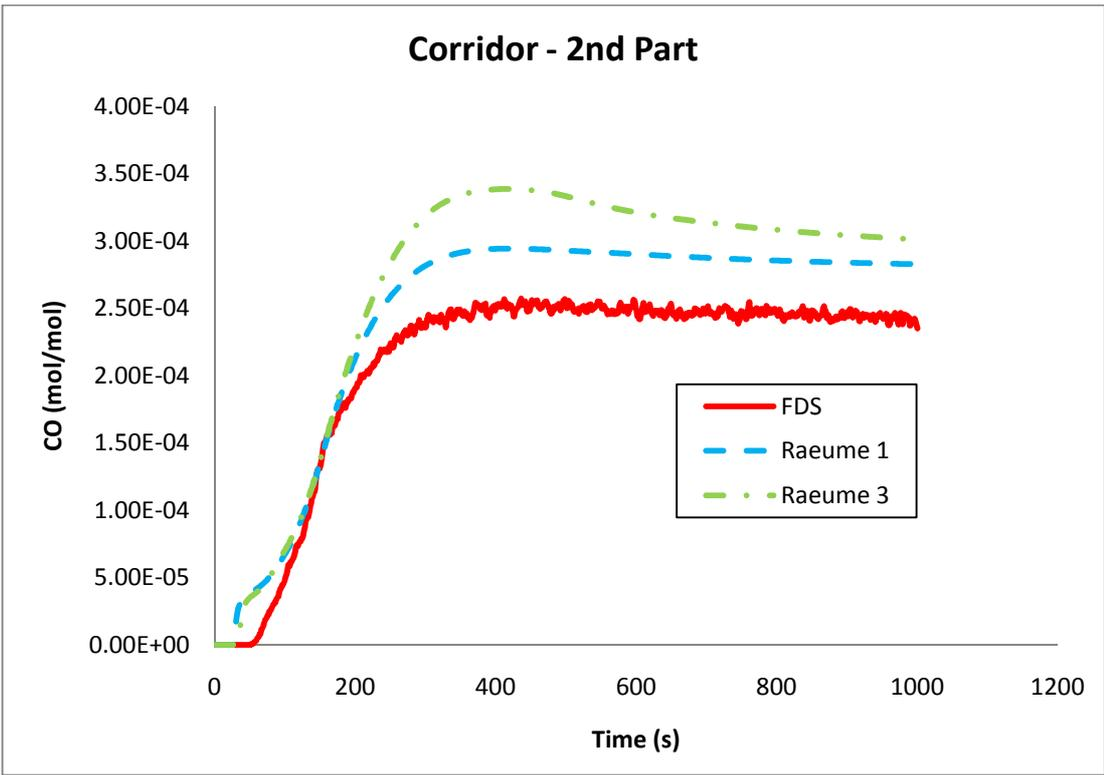
Figure B - 25: Carbon monoxide concentration (mol/mol) in the second part of the corridor.
