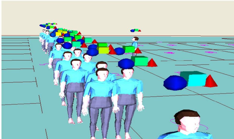
**Figure 7-4: Snapshot from the evacuation model Helios showing the indicators over the head of each evacuee (sphere for heat, cube for toxicity and cone for visibility).**
