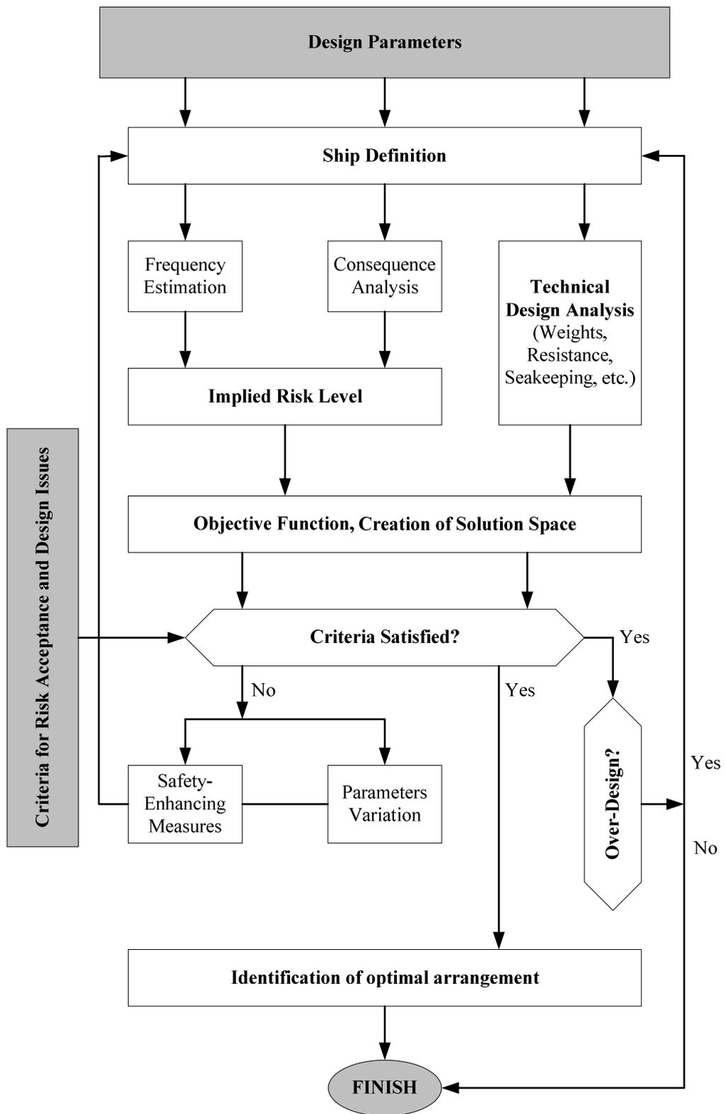
Figure 3-6: Risk-Based design framework; reproduced from [Konovessis, 2001]
