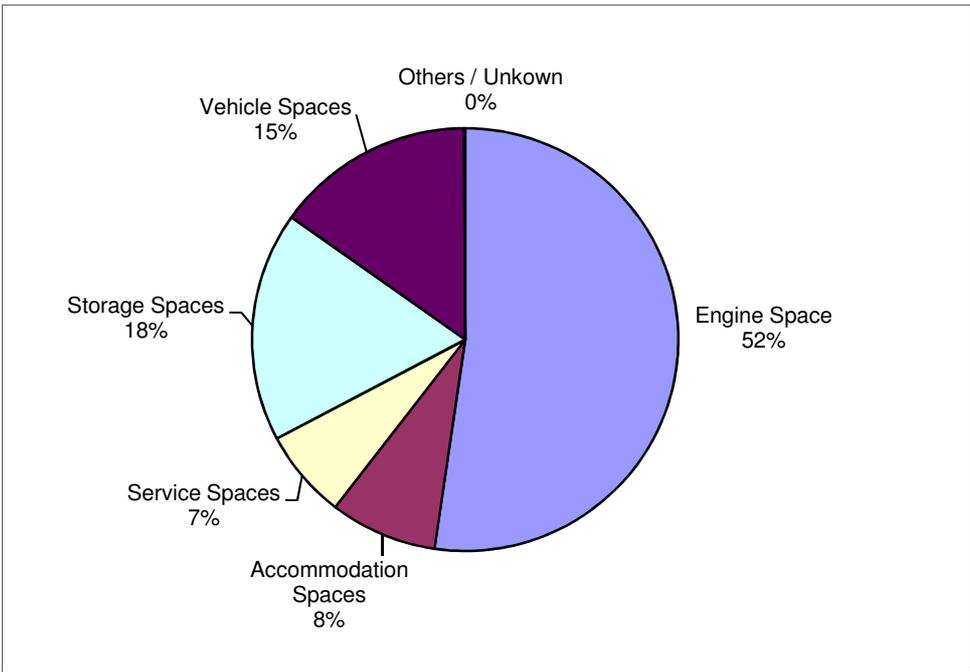
**Figure 5-4: Percentage of fatalities distributed according to location of fire origin including Al-Salam Boccaccio.**
