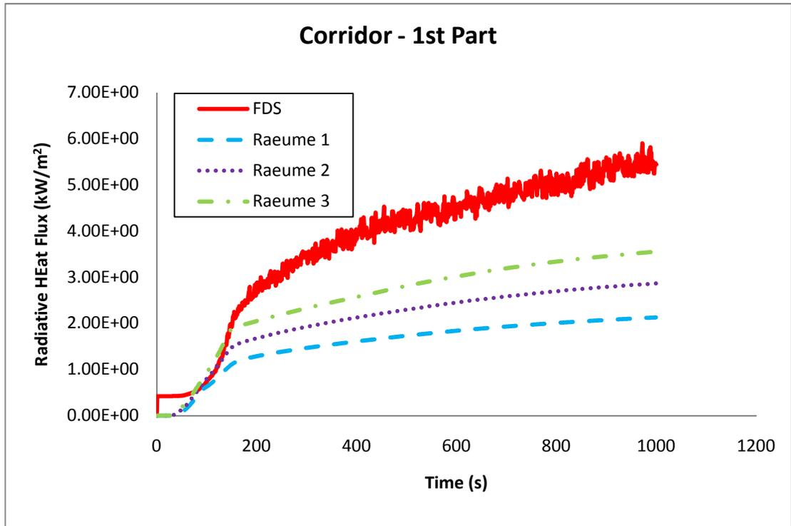
Figure B - 40: Radiative heat flux (kW/m<sup>2</sup>) in the first part of the corridor.
