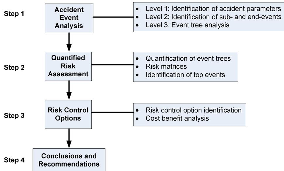
**Figure 3-4: Flow diagram of the risk assessment approach; [Bakker et al., 2000]**
