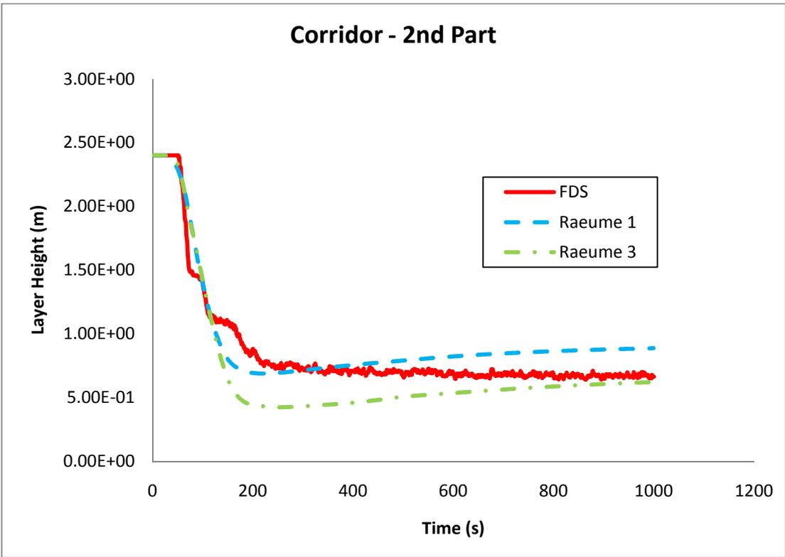
Figure B - 45: Smoke layer interface height (m) in the second part of the corridor.
