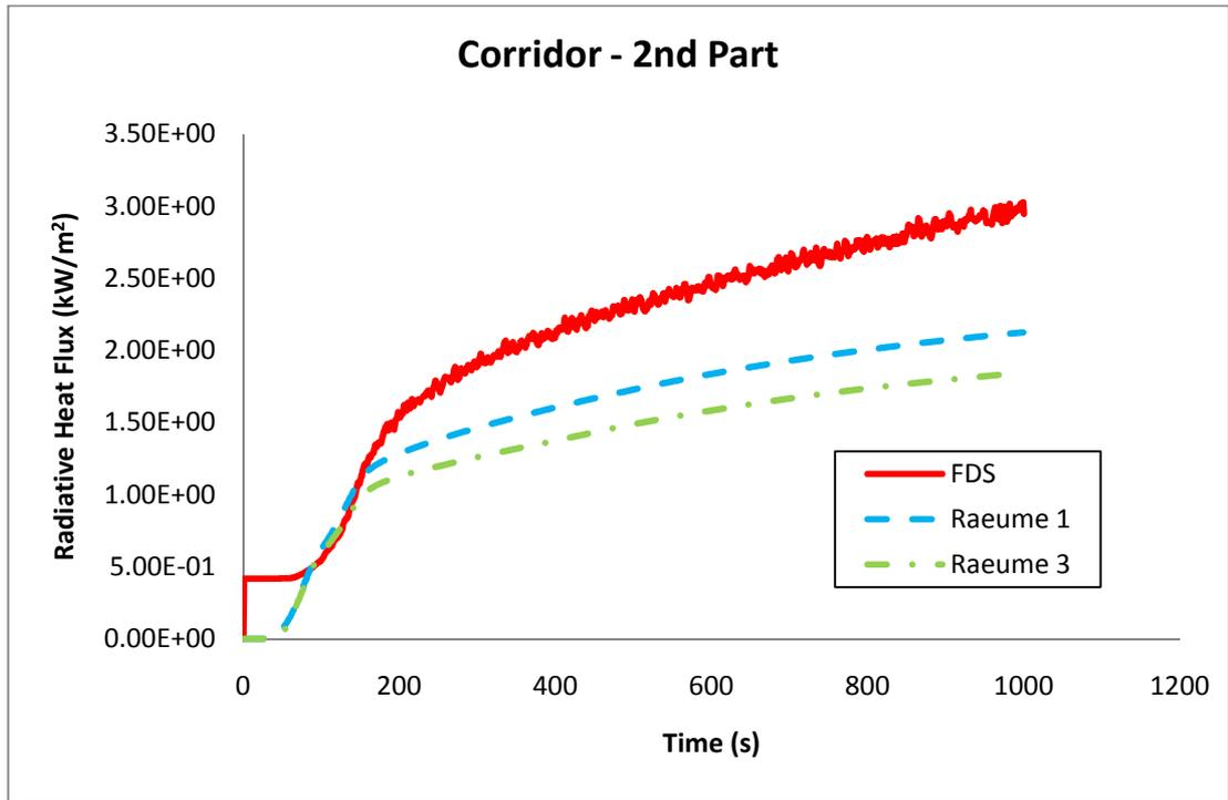
Figure B - 41: Radiative heat flux (kW/m<sup>2</sup>) in the second part of the corridor.
