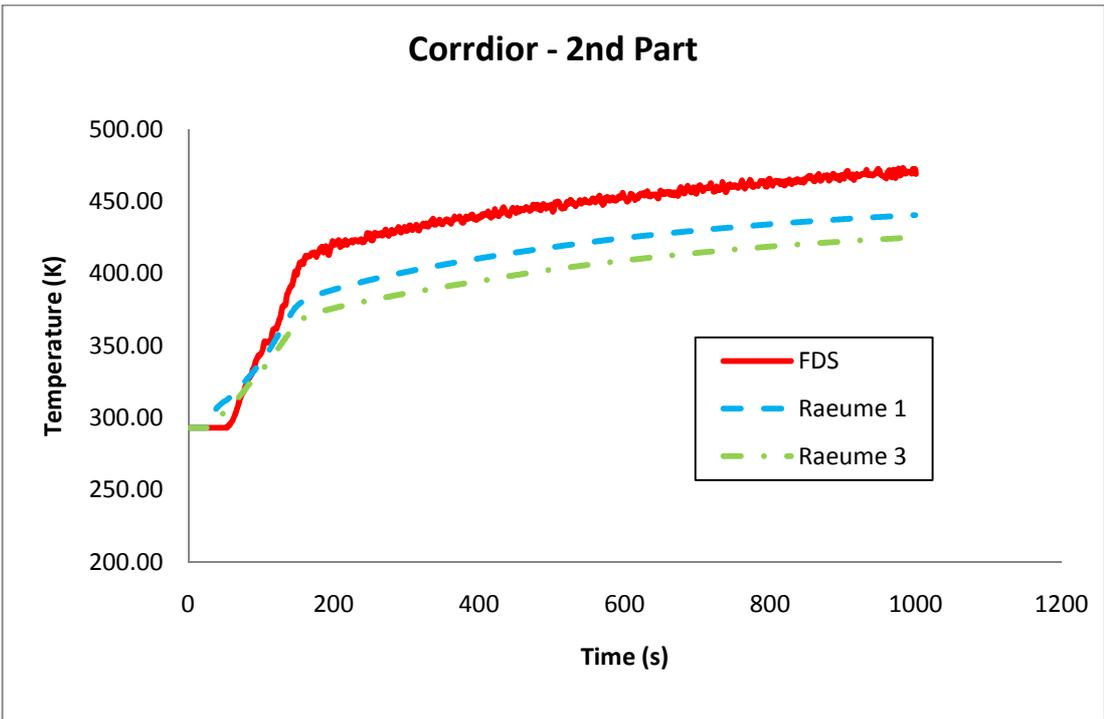
Figure B - 21: Temperature (K) in the second part of the corridor.
