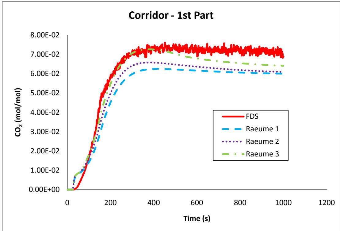
**Figure B - 28: Carbon dioxide concentration (mol/mol) in the first part of the corridor.**
