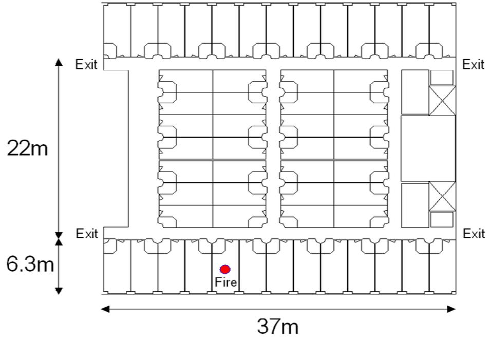
Figure 7-1: General Arrangements of the accommodation spaces fire scenario.
