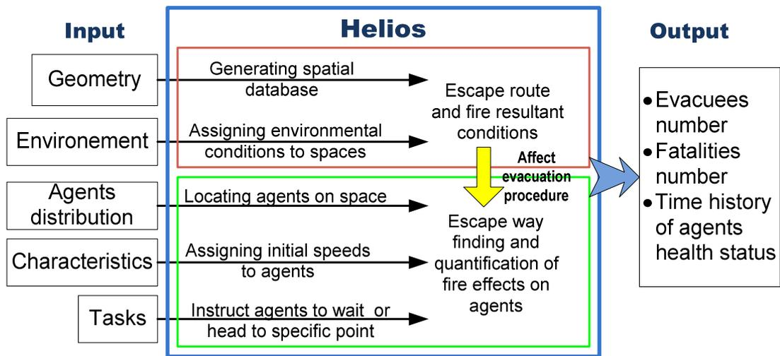
**Figure 4-6: Work procedure of the evacuation model Helios.**
