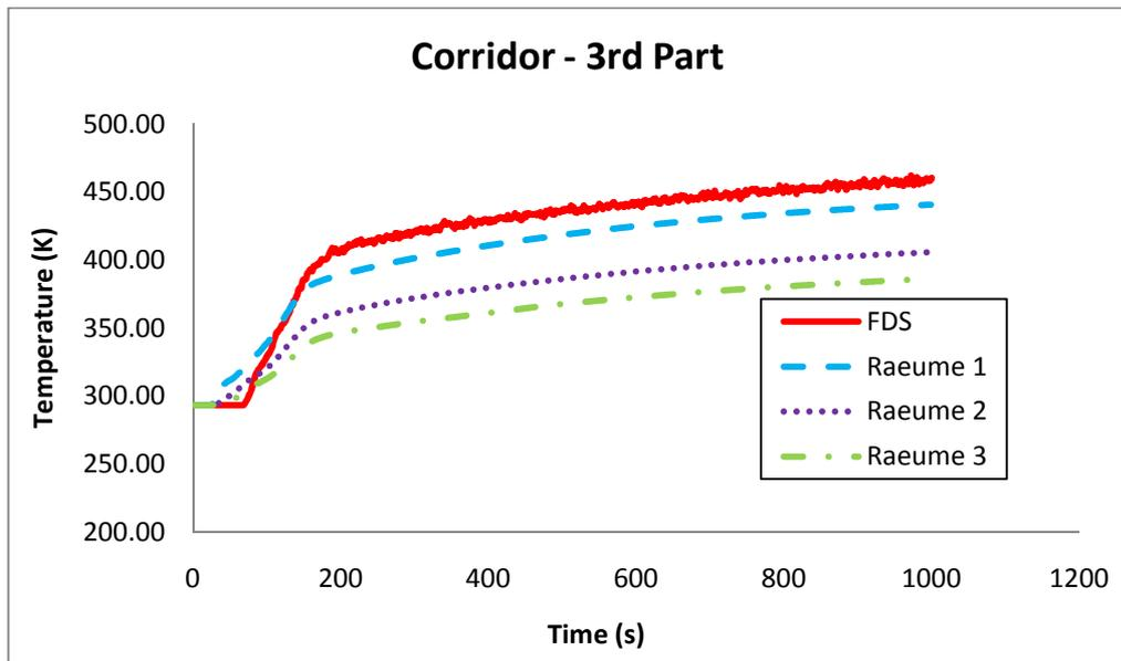
**Figure 6-21: Temperature (K) as predicted by FDS and Raeume (different configurations) in the third part of the corridor.**
