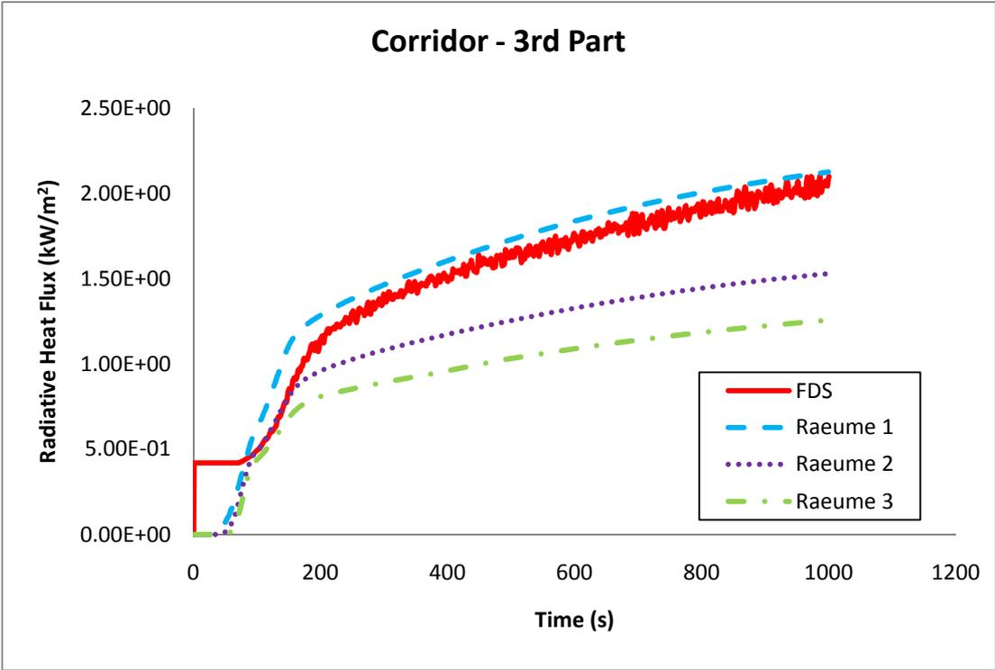
Figure B - 42: Radiative heat flux (kW/m<sup>2</sup>) in the third part of the corridor.
