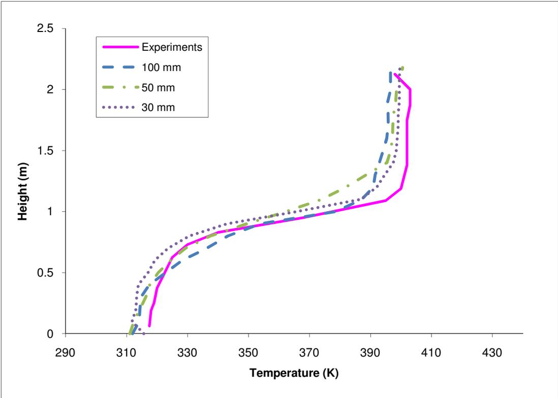
Figure 6-4: Temperature profiles in the corner of the room comparing experimental results to three simulations with different cell sizes; 100 mm, 50 mm and 30 mm.
