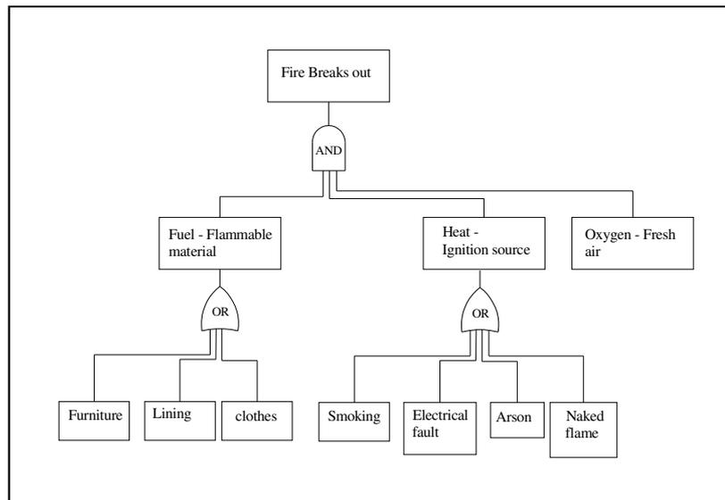
**Figure 5-1: Fault tree leading to fire in a stateroom in the accommodation area.**
