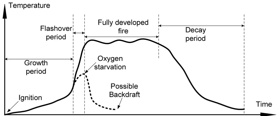
**Figure 3-12: Fire development stages; the solid curve represent a well-ventilated fire journey, the dotted curve is a fire under effect of oxygen depletion. [Karlsson and Quintiere, 2000] [Drysdale, 1988]**
