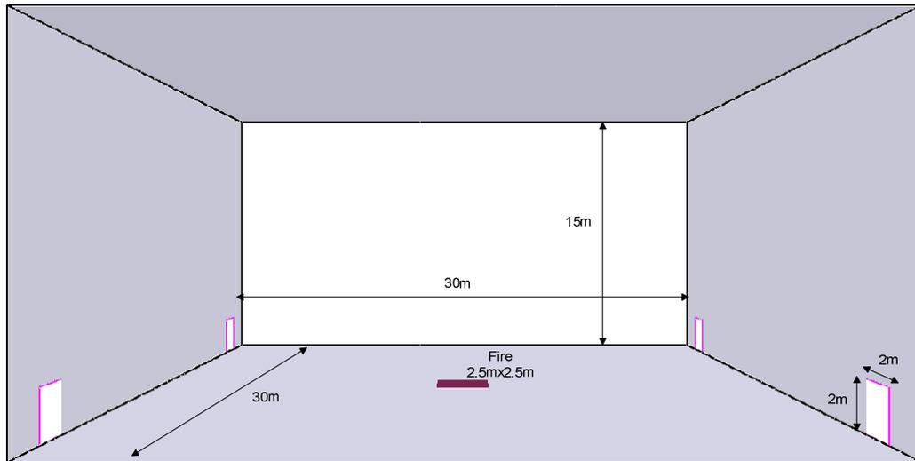
**Figure 6-15: Atrium geometrical configuration.**
