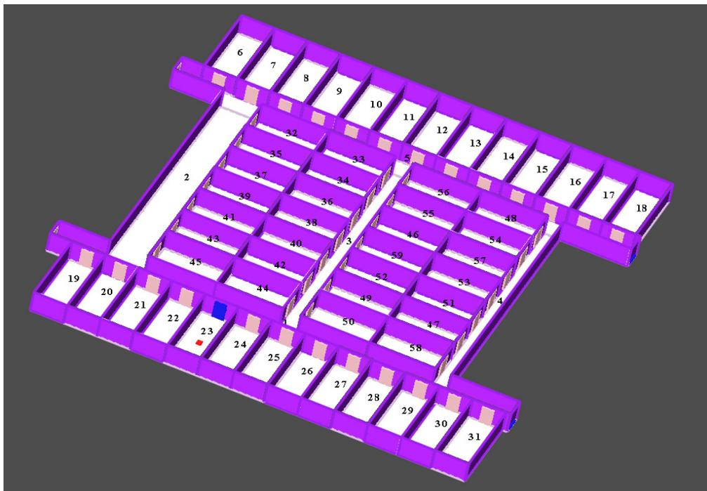
Figure 7-2: Snapshot from RamEditor (pre-processor of Raeume) illustrating the accommodation spaces including all the cabins and corridors where the evacuation process takes place.
