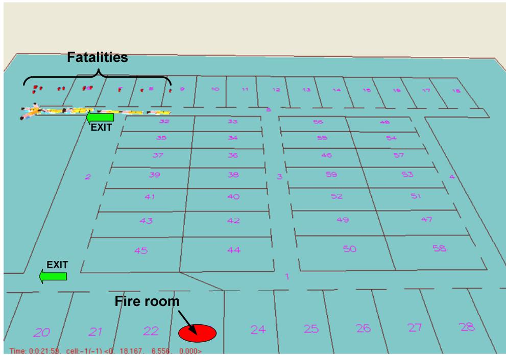
Figure 7-7: Snapshot from Helios showing the fatalities at the end of the corridor near the exit.
