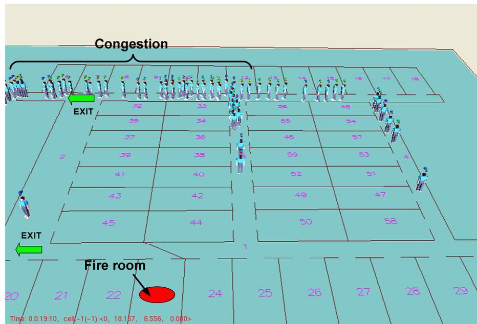
**Figure 7-6: Snapshot from Helios showing the congestion occurring in the fire scenario with two blocked exits.**
