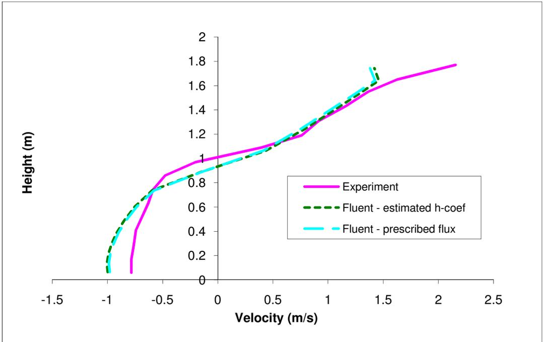
**Figure 6-11: Velocity profiles in the doorway of the room. The “estimated h-coef” is where the thermal boundaries are defined by estimating the heat transfer coefficient and “prescribed flux” is where the heat fluxes through boundaries are defined from previous knowledge.**
