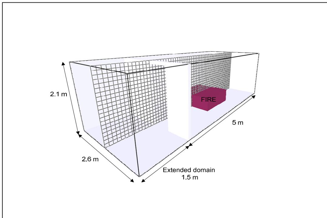
**Figure 6-12: A Smokeview snapshot for the cabin fire configurations.**
