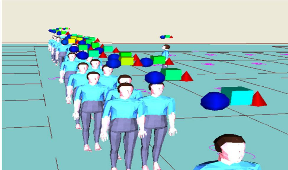
**Figure 7-4: Snapshot from the evacuation model Helios showing the indicators over the head of each evacuee (sphere for heat, cube for toxicity and cone for visibility).**
