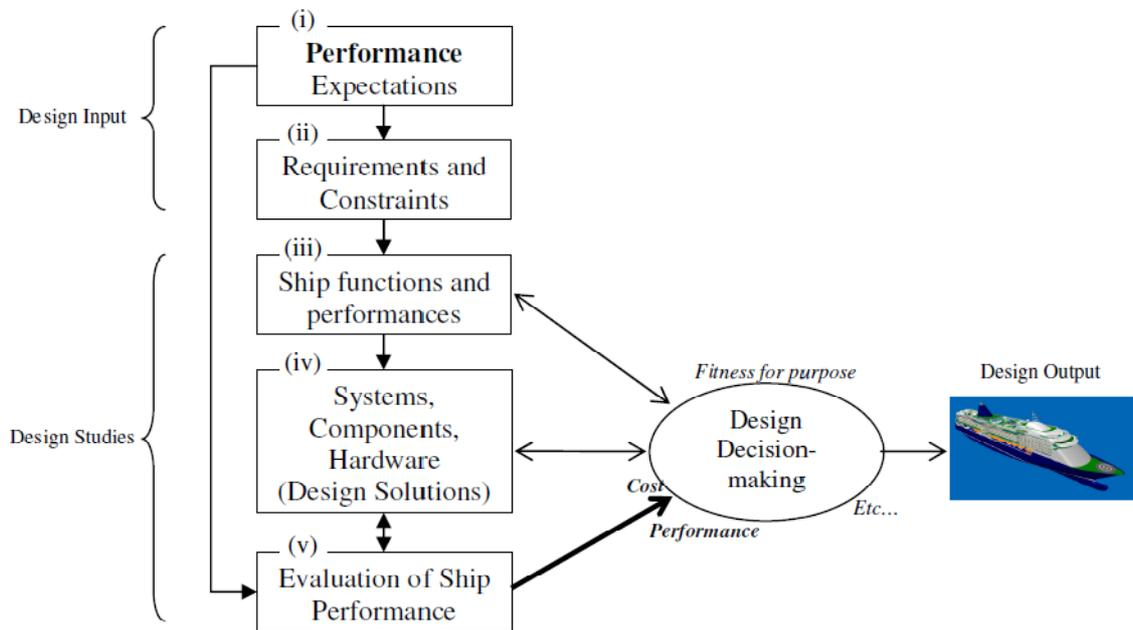
**Figure 3-2: High level conventional design process [Vassalos et al., 2006]**
