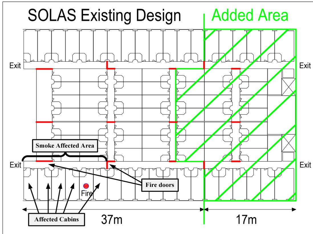
**Figure 8-5: The compartmentation of SOLAS and extended design by self-closing doors for smoke controlling purpose. Compartmentation doors are indicated as red lines.**
