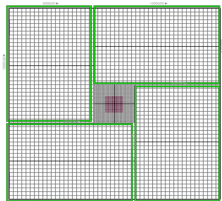
**Figure 6-16: Top view for the grid configuration of the atrium, showing the fine mesh in the centre surrounded by four symmetrical coarser meshes.**
