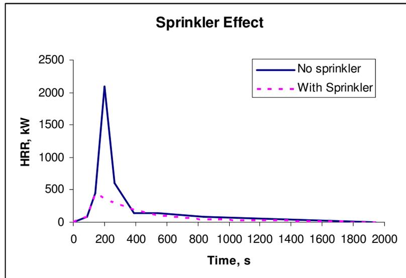
**Figure 4-4: Sprinkler effects on the heat release rate.**
