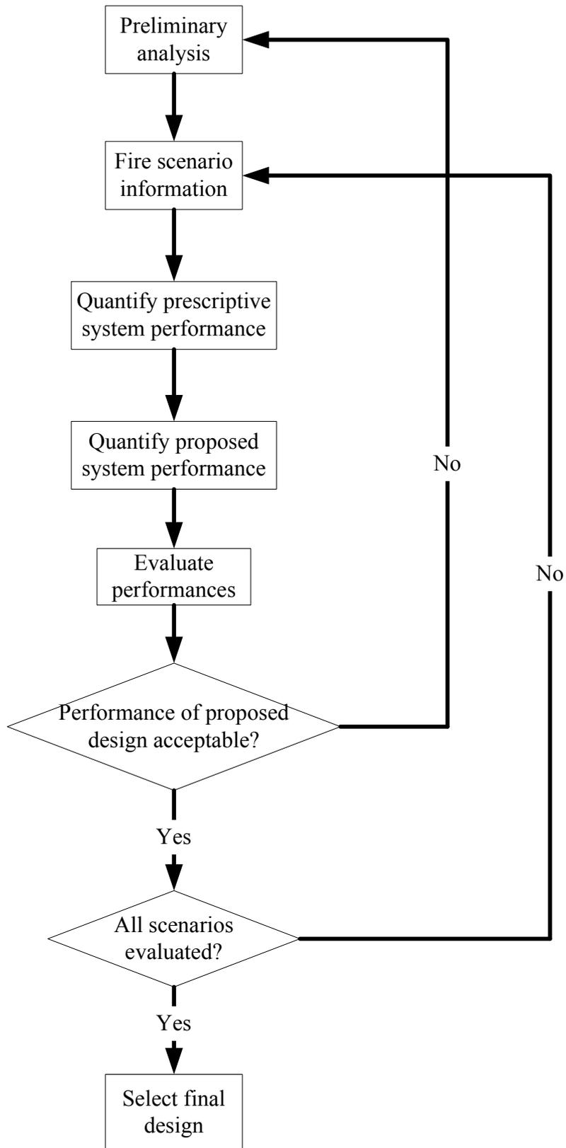
Figure 3-1: Alternative design and arrangements process flowchart [IMO, 2001].
