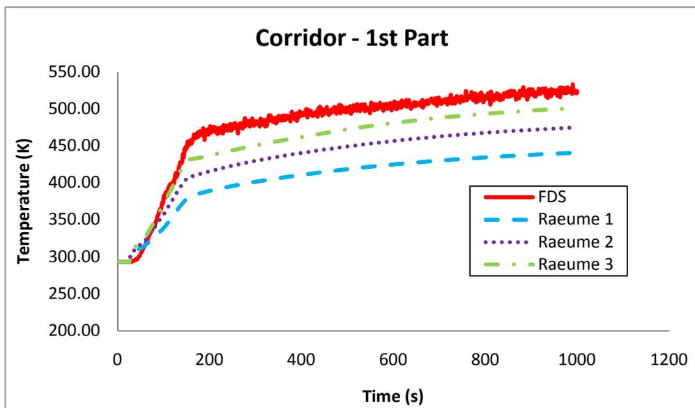
**Figure 6-20: Temperature (K) as predicted by FDS and Raeume (different configurations) in the first part of the corridor.**
