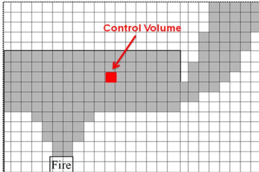
**Figure 4-5: The two layers and plumes in a room fire as divided by field models into small control volume.**
