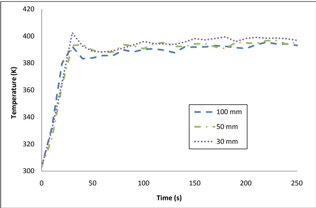
Figure 6-3: Temperature time histories monitored, for the purpose of grid sensitivity study, in the room corner at 1.6 m height of three different cell sizes: 100 mm, 50 mm and 30 mm.
