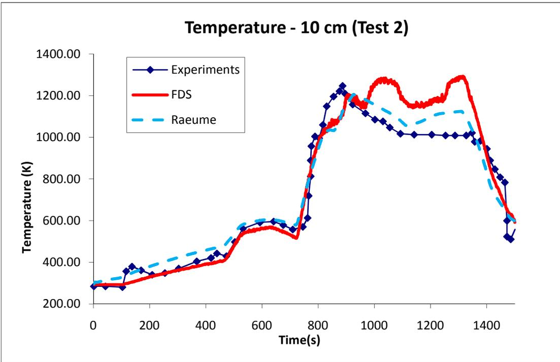
Figure B - 7: Temperature profiles, measured and predicted at 10 cm below ceiling for test 2
