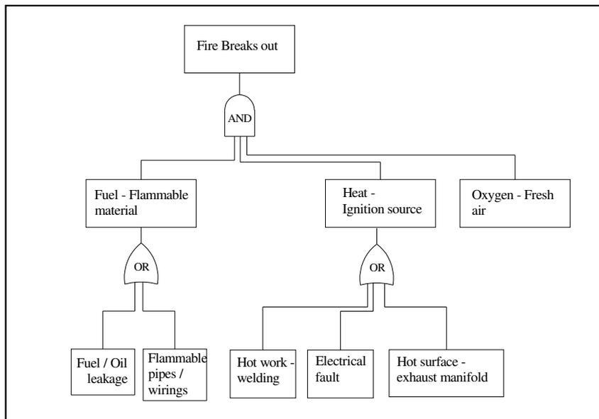
**Figure 5-2: Fault tree leading to fire in the engine room.**
