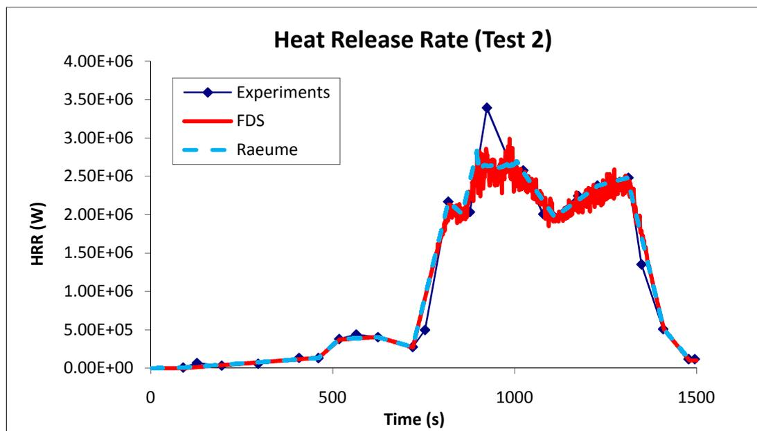
Figure B - 2: Heat Release Rates, measured and predicted for test 2
