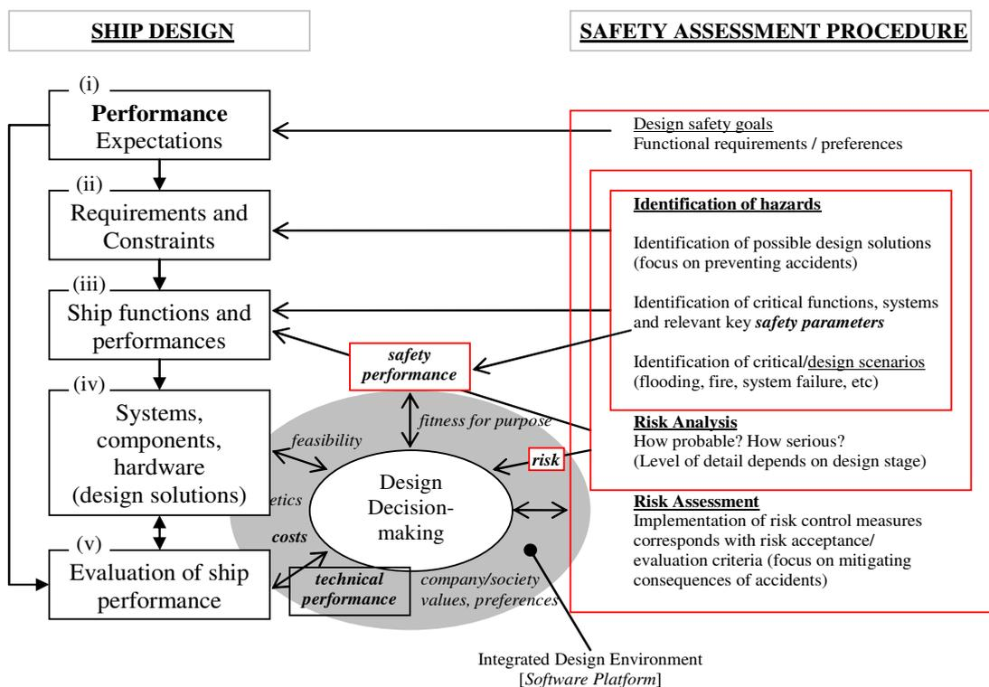
Figure 3-7: High level framework for risk-based design implementation [Vassalos et al., 2006]
