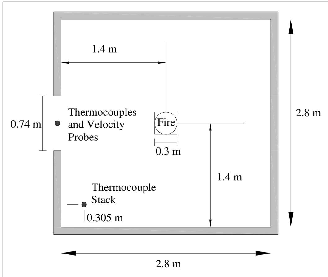
Figure 6-1: Configuration of the Steckler fire room [Steckler et al., 1982].
