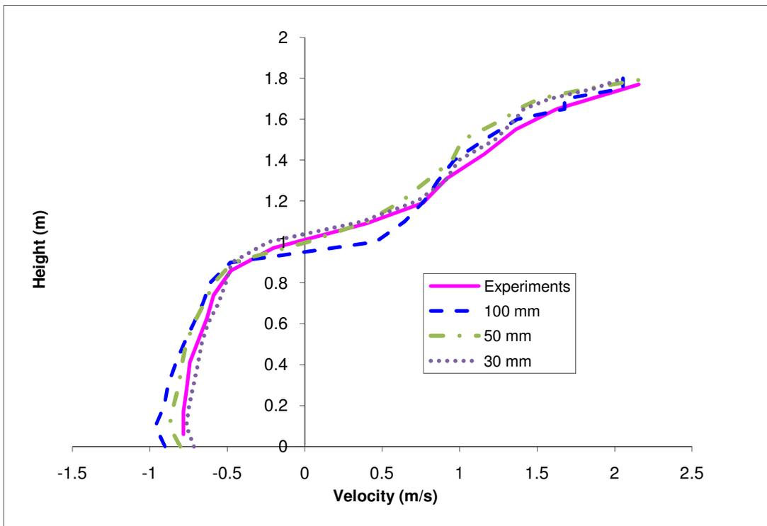
**Figure 6-6: Velocity profiles in the doorway of the room comparing experimental results to three simulations with different cell sizes; 100 mm, 50 mm and 30 mm.**
