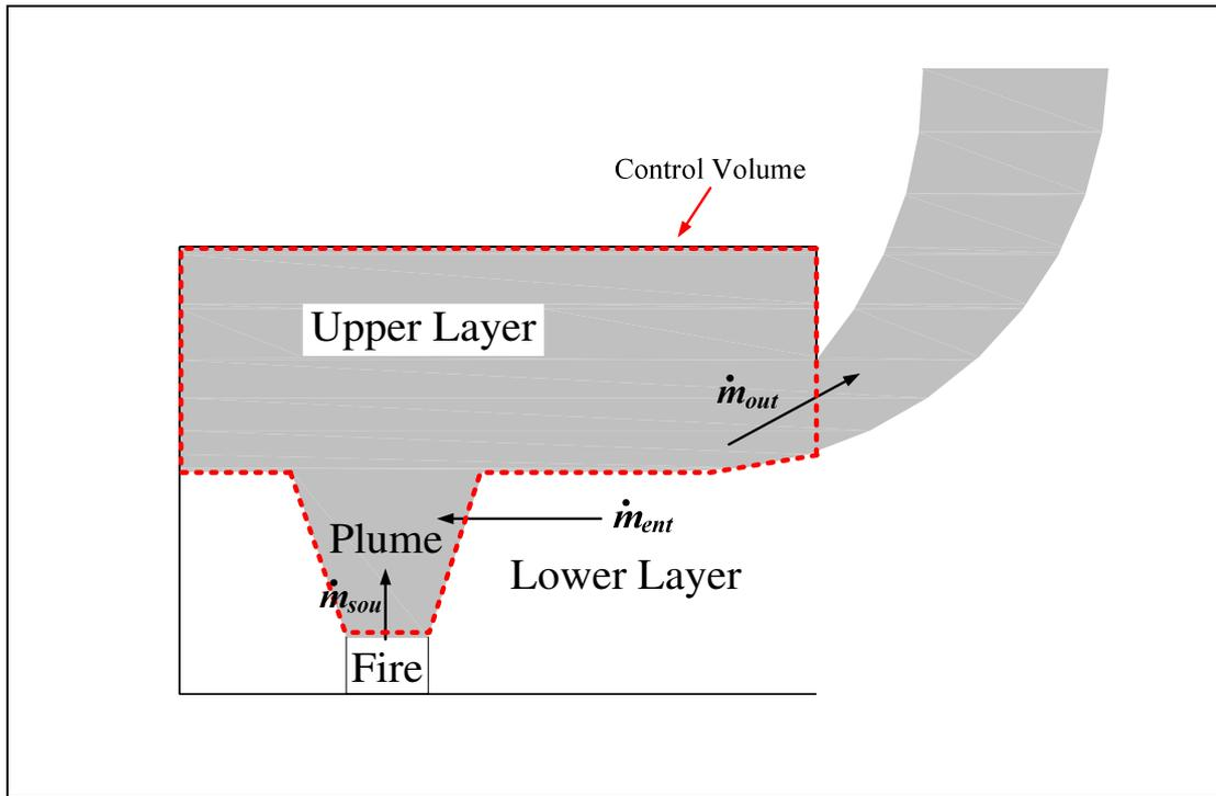
**Figure 4-3: The two layers (upper and lower) and the fire plume observed in enclosure's fire.**
