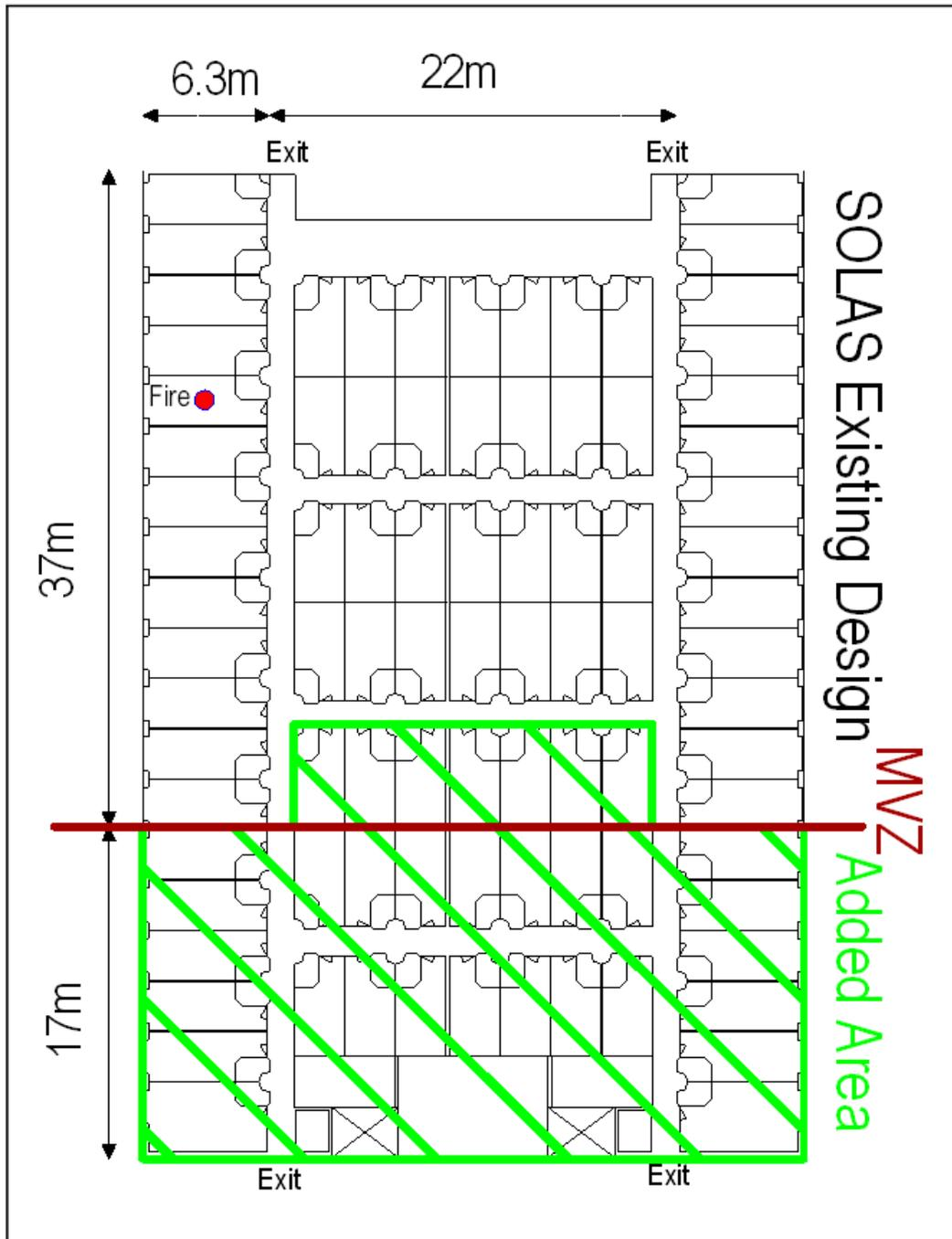
Figure 8-1: General Arrangements of the existing design complying with SOLAS and the additional area violating the rule restricting the size of a MVZ.
