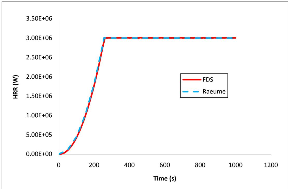
Figure B - 18: Output heat release rate (W) in the atrium as predicted by FDS and Raeume.
