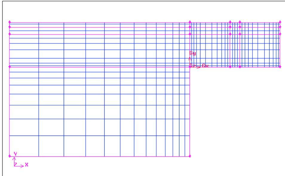
**Figure 6-7: X-Y plane top view of the computational domain and mesh in Gambit**
