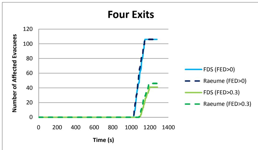
**Figure 7-5: Time histories of the affected evacuees with different severities of toxicities assuming four exits are used for escape. Solid lines \_\_\_ represent the prediction of FDS results integrated with Helios. Broken lines \_\_\_ represent the casualties predicted by the integration of Raeume results with Helios.**
