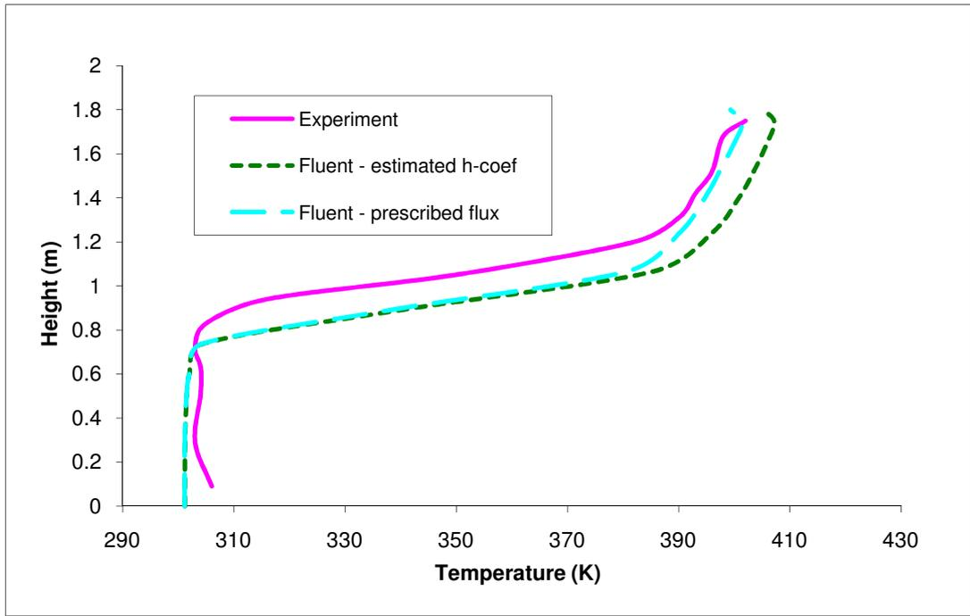
**Figure 6-10: Temperature profiles in the doorway of the room. The “estimated h-coef” is where the thermal boundaries are defined by estimating the heat transfer coefficient and “prescribed flux” is where the heat fluxes through boundaries are defined from previous knowledge.**
