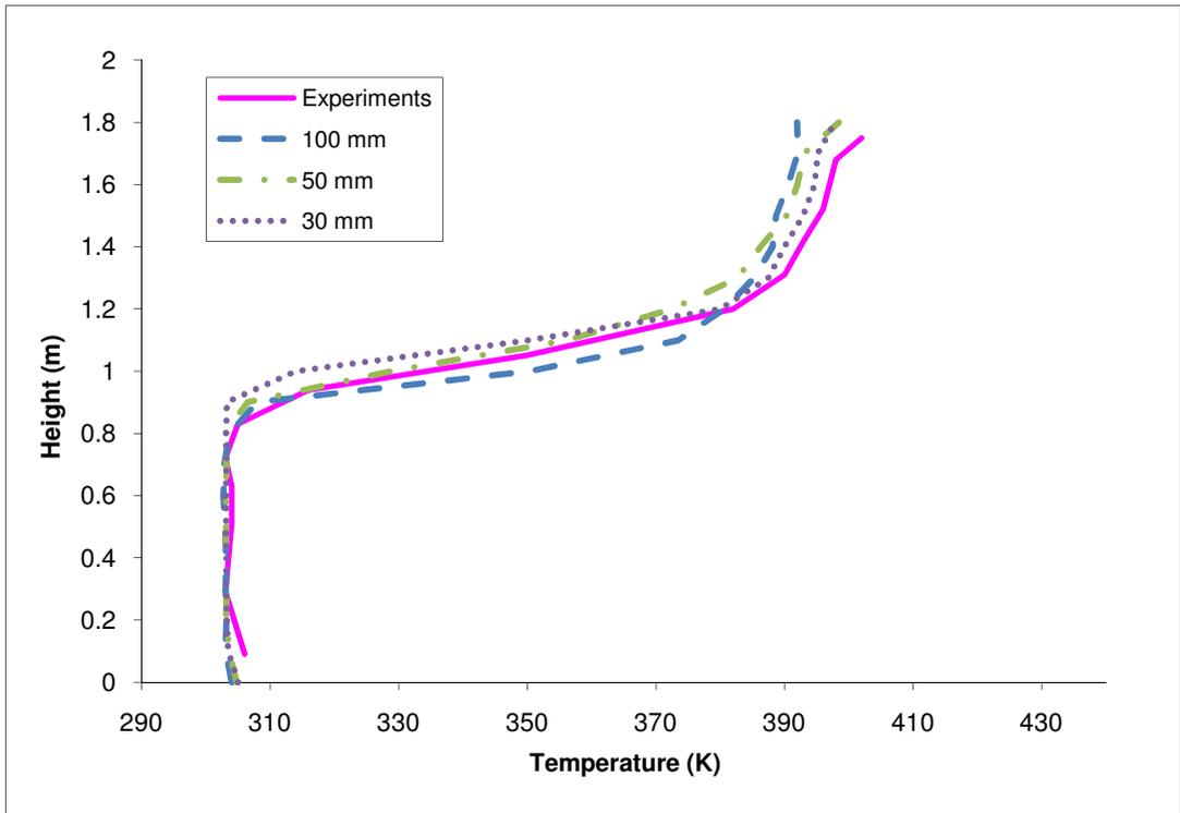
**Figure 6-5: Temperature profiles in the doorway of the room comparing experimental results to three simulations with different cell sizes; 100 mm, 50 mm and 30 mm.**
