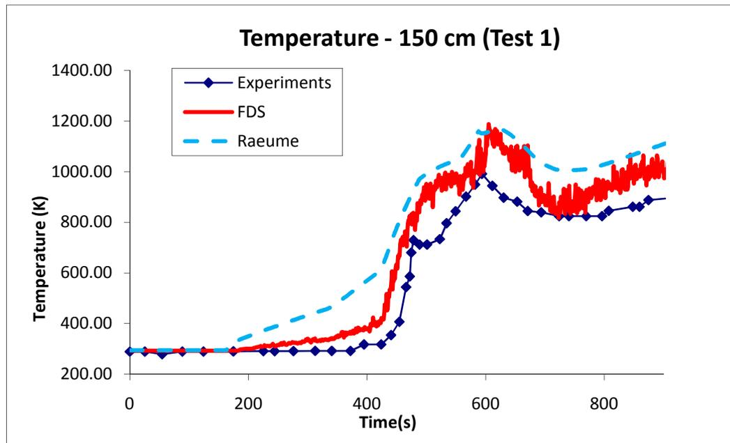
Figure 6-13: Comparison of the temperature as measured in experiments and predicted by FDS and Raeume at 150 cm below ceiling for cabin fire test 1.
