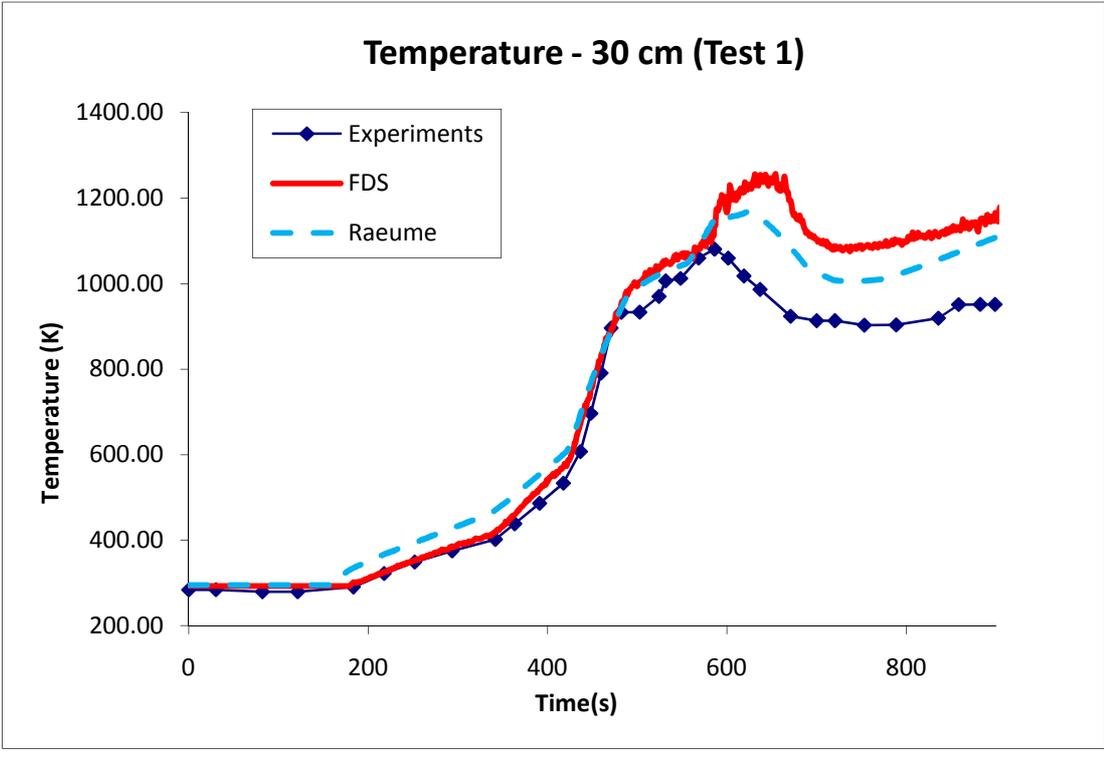
Figure B - 4: Temperature profiles, measured and predicted at 30 cm below ceiling for test 1
