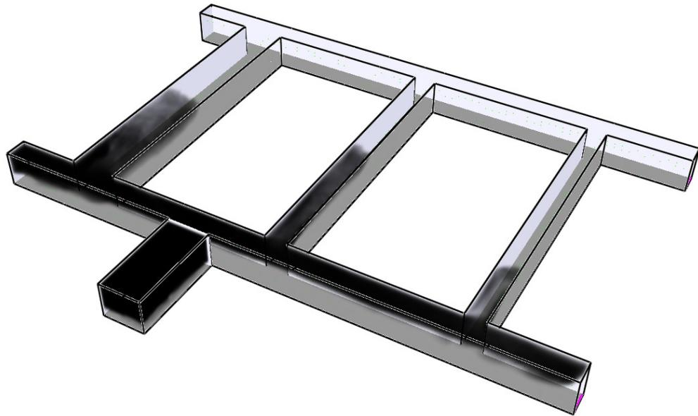
**Figure 7-3: Snapshot from Smokeview (post-processor of FDS) illustrating the accommodation spaces corridors where the smoke propagation is predicted.**
