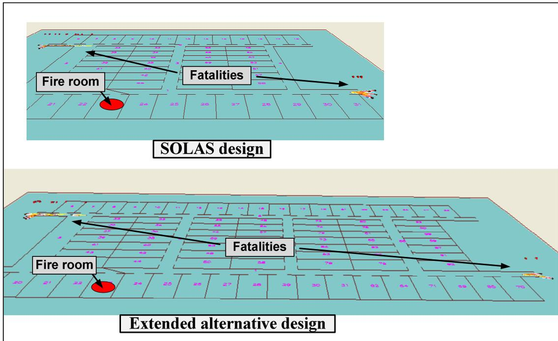
**Figure 8-3: Layouts of the SOLAS and the extended alternative designs showing the locations of fatalities in both fire scenarios.**
