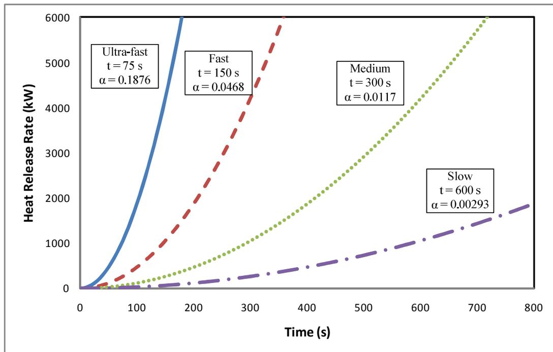
Figure 3-11: Heat Release Rates of  $t^2$  fire categories.
