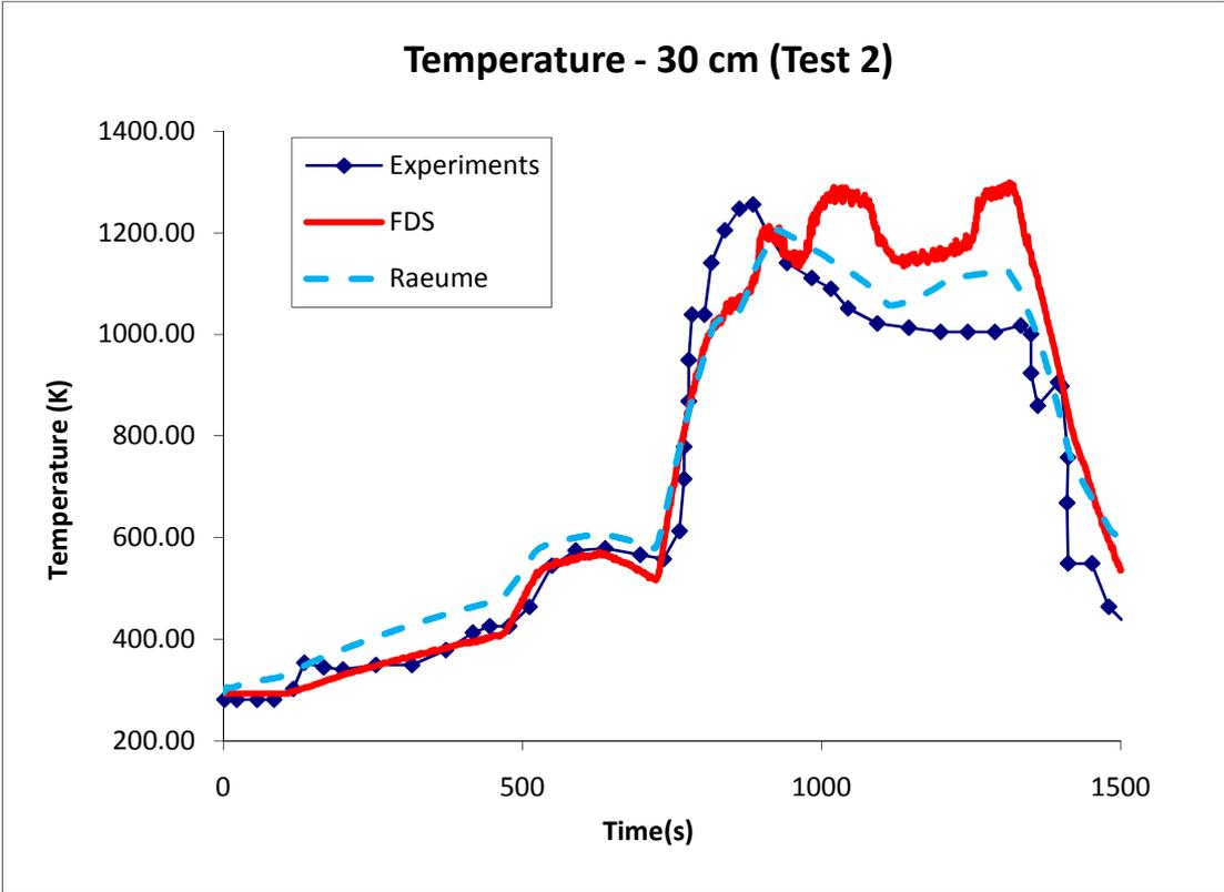
Figure B - 8: Temperature profiles, measured and predicted at 30 cm below ceiling for test 2
