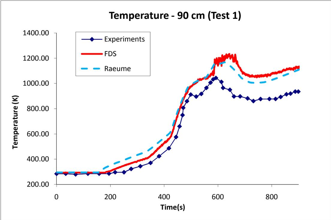
Figure B - 5: Temperature profiles, measured and predicted at 90 cm below ceiling for test 1
