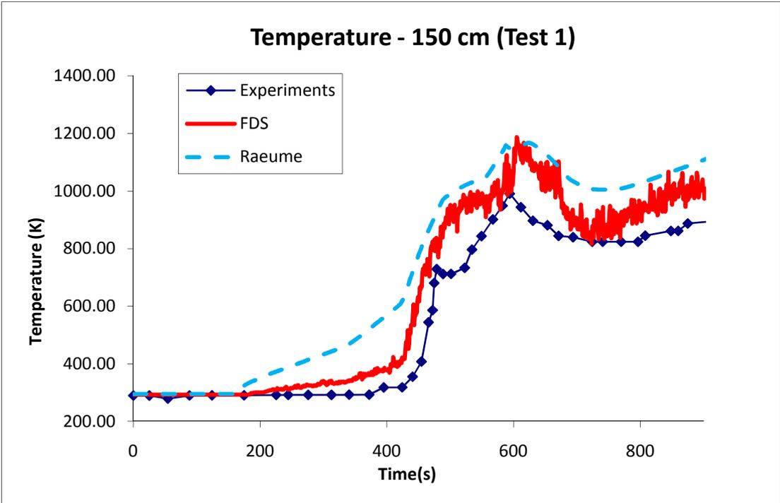
Figure B - 6: Temperature profiles, measured and predicted at 150 cm below ceiling for test 1
