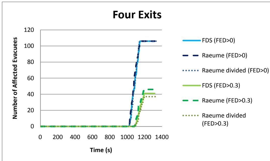
Figure 7-10: Comparison of the affected evacuees time histories assuming two exits are used for escape. Solid lines \_\_\_ represent the prediction of FDS results integrated with Helios. Broken lines \_\_\_ represent the casualties predicted by the integration of Raeume results with Helios. Dotted lines ..... represent the results of Raeume when the long corridors are divided into smaller compartments.
