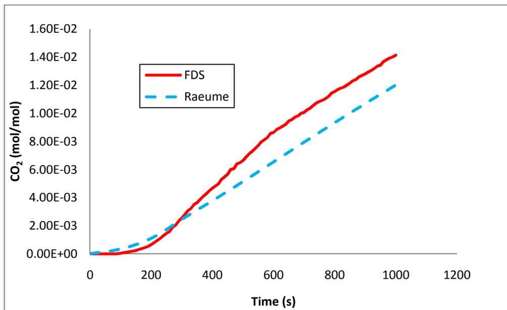
**Figure 6-17: Carbon dioxide concentration in an atrium as compared between FDS and Raeume predictions.**
