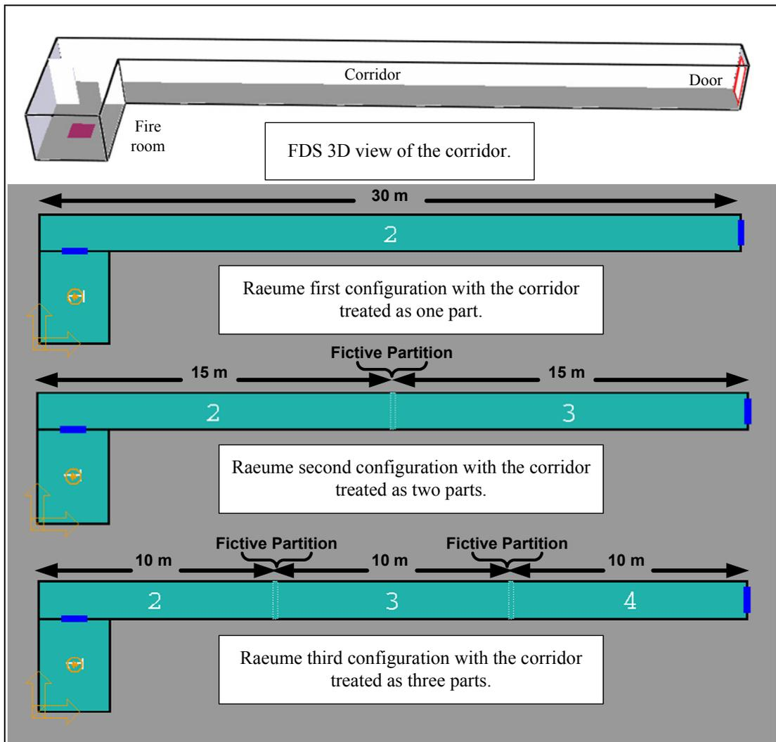
**Figure 6-19: Snapshots illustrating from top to bottom; the corridor and fire cabin as shown by Smokeview the postprocessor of FDS, the three configurations of Raeume as taken by the pre-processor RamEditor for the corridor treated as one part, two parts or three parts, respectively.**
