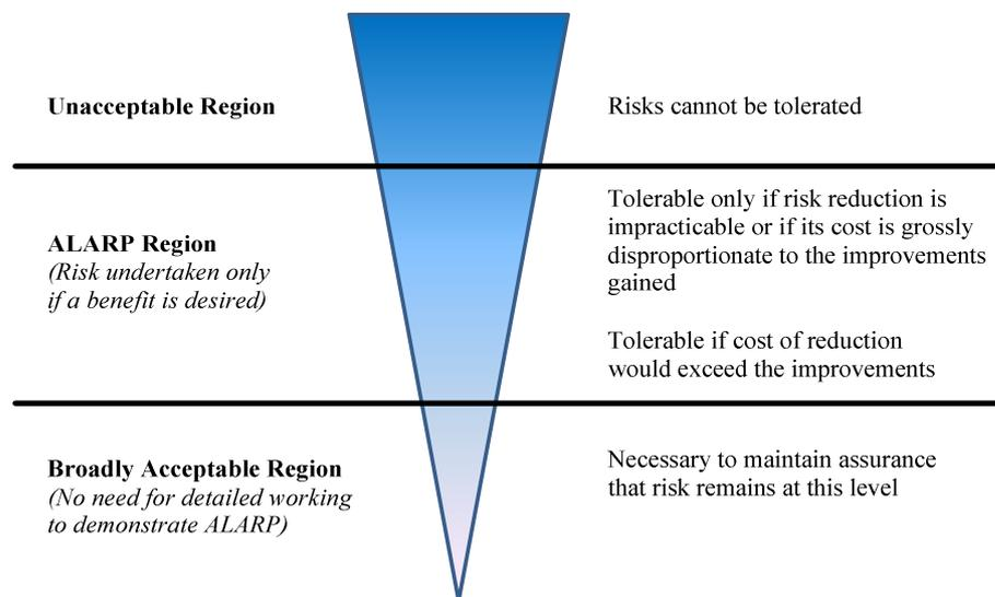
**Figure 3-8: The ALARP concept; [HSE, 1992]**
