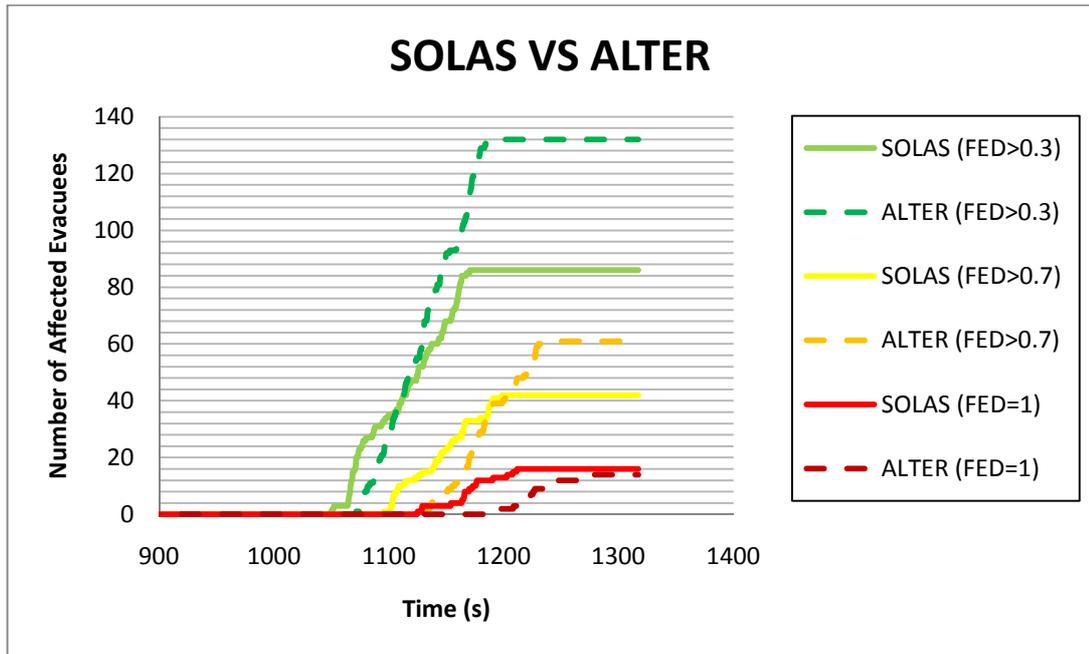
**Figure 8-2: Time histories of the affected evacuees with different severities of toxicities. Solid lines \_\_\_ represent the casualties of SOLAS complying design while broken lines \_ \_ \_ represent the extended alternative design.**
