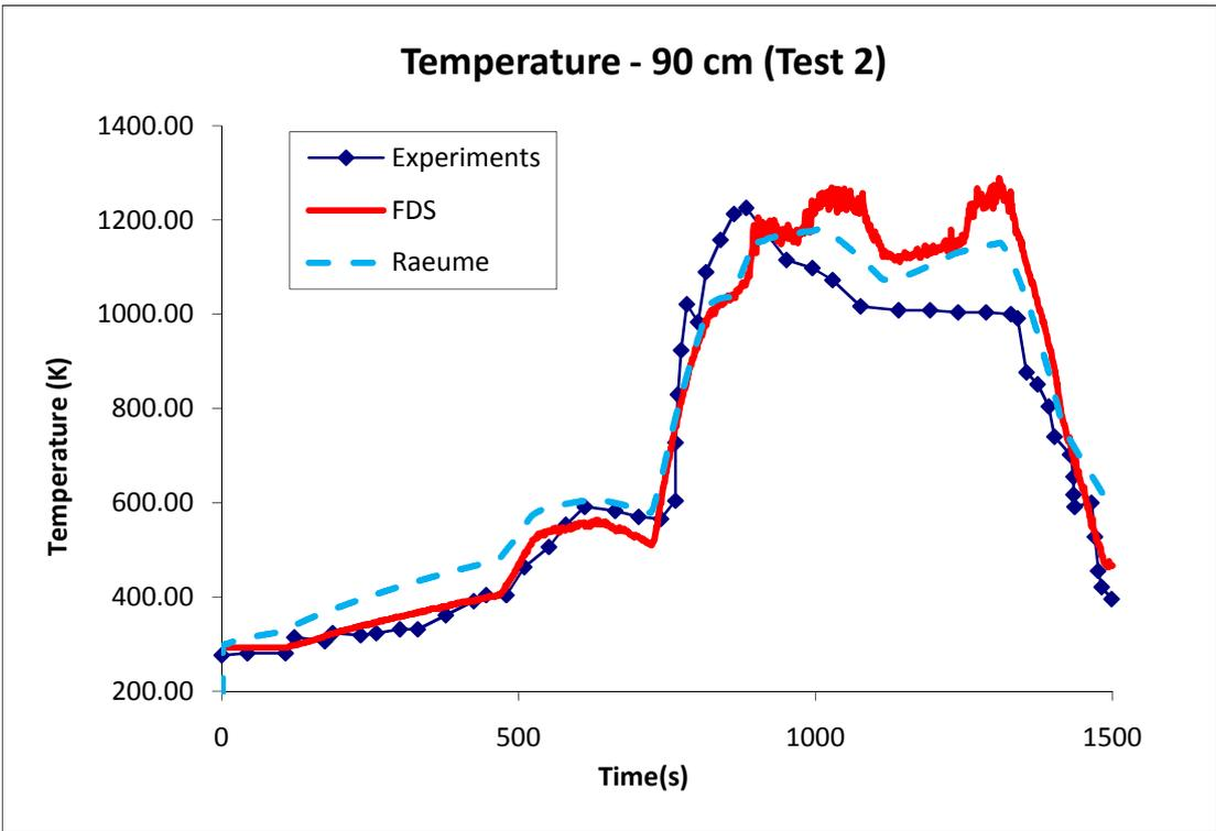
Figure B - 9: Temperature profiles, measured and predicted at 90 cm below ceiling for test 2
