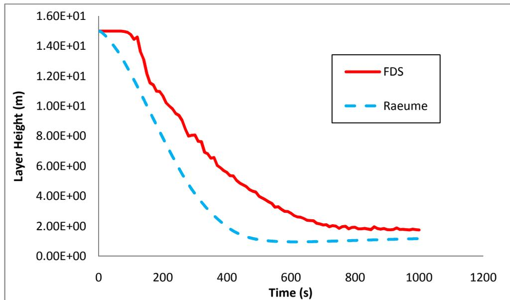
**Figure 6-18: Layer height interface in an atrium as compared between FDS and Raeume predictions.**
