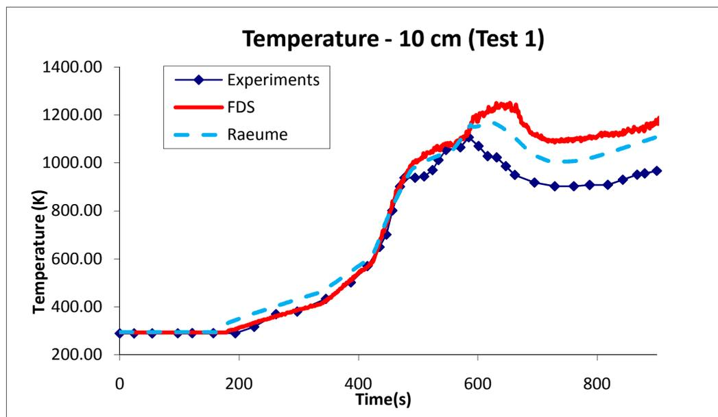
Figure 6-14: Comparison of the temperature as measured in experiments and predicted by FDS and Raeume at 10 cm below ceiling for cabin fire test 1.
