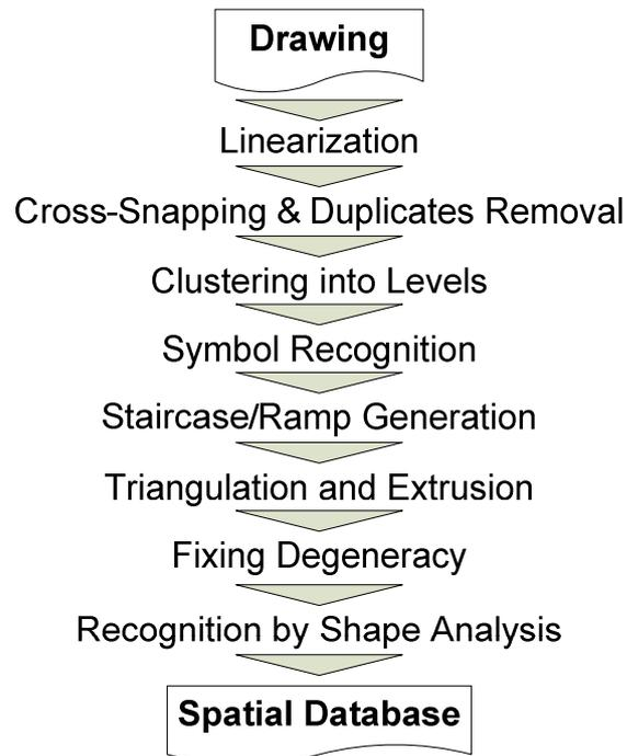
**Figure 4-7: General arrangement drawings to special database reproduced from [Majumder et al., 2005b].**
