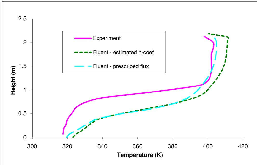
**Figure 6-9: Temperature profiles in the corner of the room. The “estimated h-coef” is where the thermal boundaries are defined by estimating the heat transfer coefficient and “prescribed flux” is where the heat fluxes through boundaries are defined from previous knowledge.**
