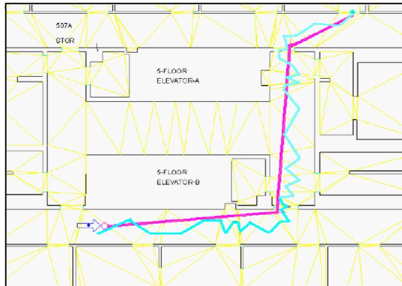
**Figure 4-9: Evacuee's path as based on furthest visible way point comparing to adjacent way point [Majumder et al., 2005b].**
