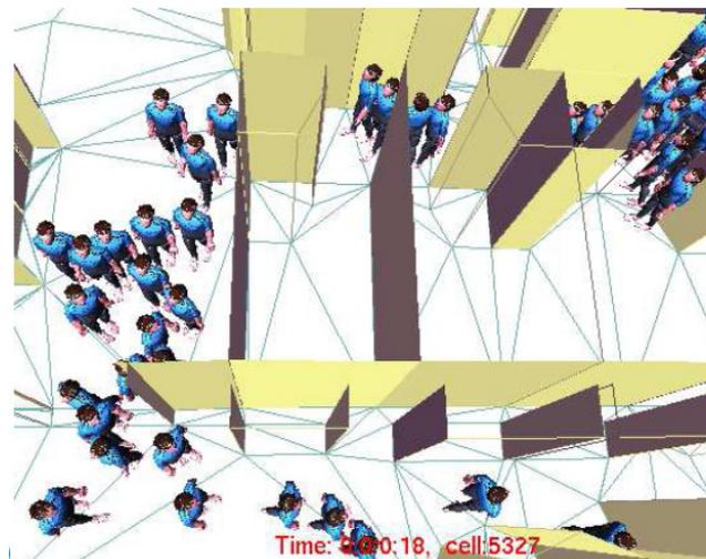
**Figure 4-8: Triangle mesh of floor space in cabins area.**
