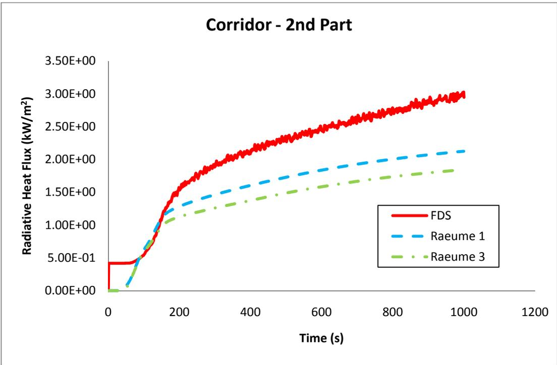
Figure B - 41: Radiative heat flux (kW/m<sup>2</sup>) in the second part of the corridor.
