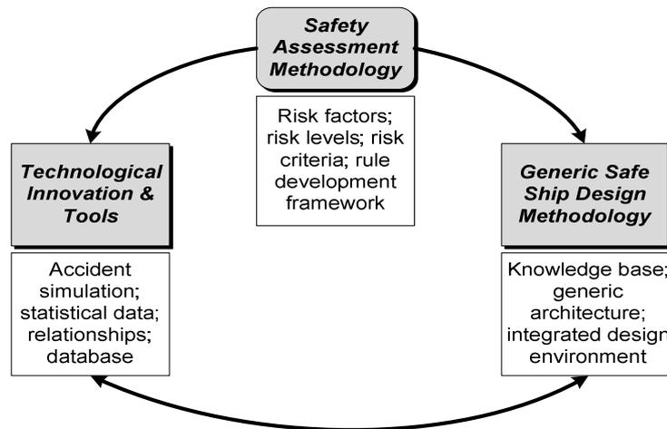
**Figure 3-3: Iterative process of the design for safety philosophy [Vassalos, 1999].**
