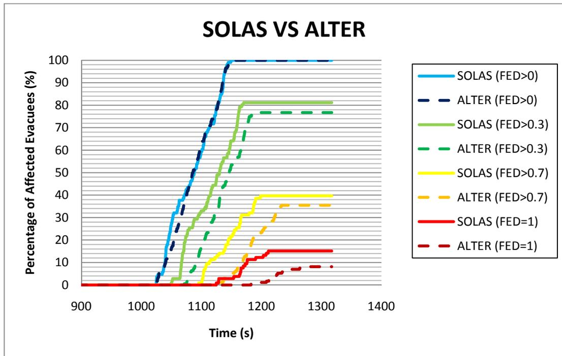
**Figure 8-4: Time histories of the percentages of affected evacuees with different severities of toxicities. Solid lines \_\_\_ represent the casualties of SOLAS complying design while broken lines --- represent the extended alternative design.**
