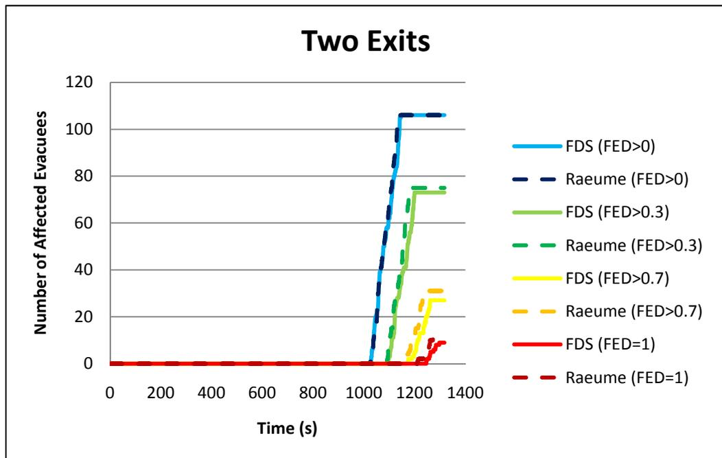
Figure 7-8: Time histories of the affected evacuees with different severities of toxicities assuming two exits are used for escape. Solid lines \_\_\_ represent the prediction of FDS results integrated with Helios. Broken lines \_\_\_ represent the casualties predicted by the integration of Raeume results with Helios.
