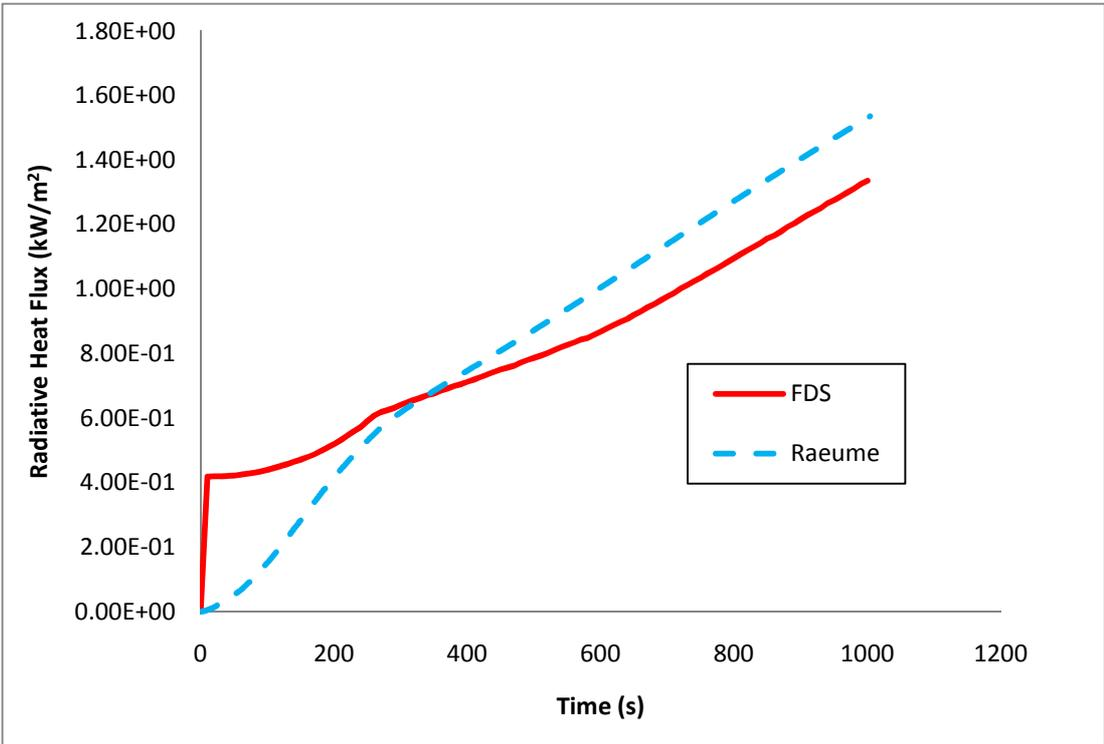
Figure B - 16: Radiative heat flux (kW/m²) in the atrium as predicted by FDS and Raeume.
