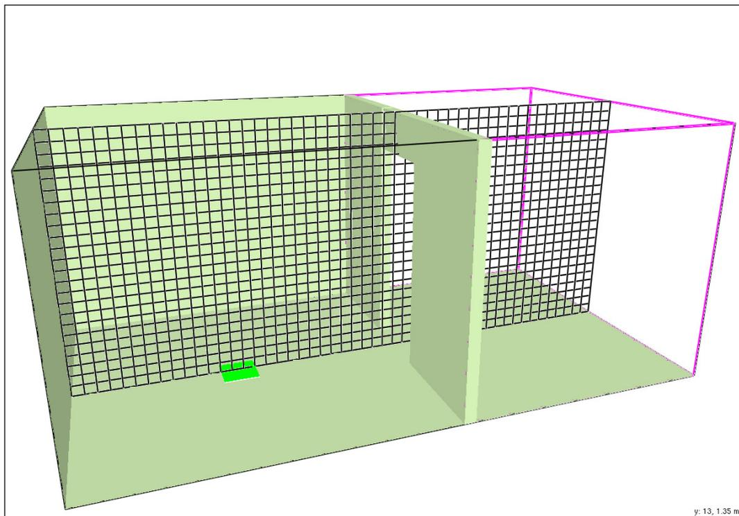
**Figure 6-2: Snapshot from Smokeview, the post-processor of FDS showing the geometry and a slice view of the grid.**
