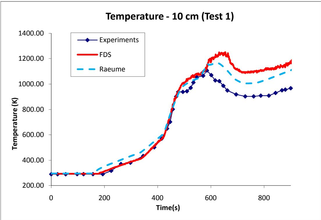
Figure B - 3: Temperature profiles, measured and predicted at 10 cm below ceiling for test 1
