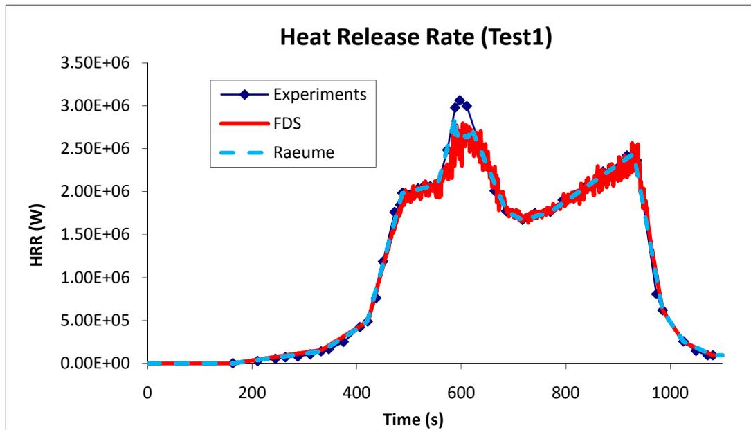
Figure B - 1: Heat Release Rates, measured and predicted for test 1
