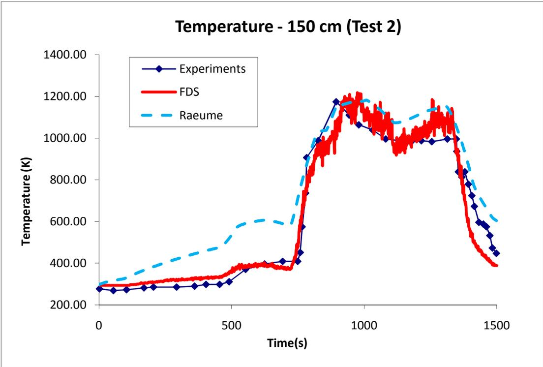
Figure B - 10: Temperature profiles, measured and predicted at 150 cm below ceiling for test 2
