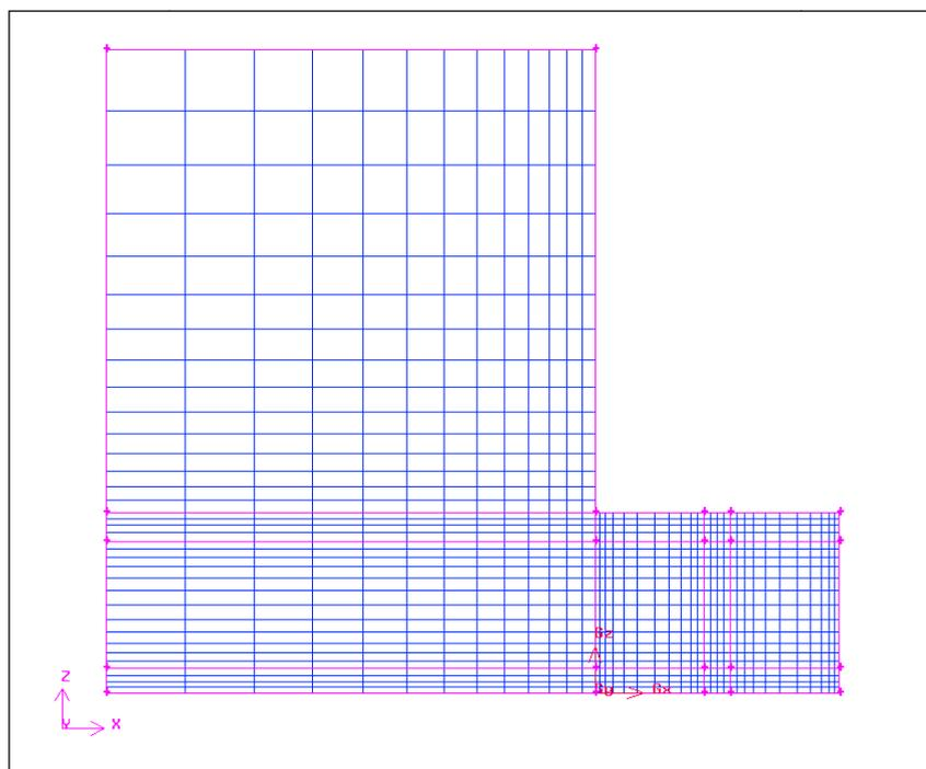
**Figure 6-8: X-Z plane profile of the computational domain and mesh in Gambit.**
