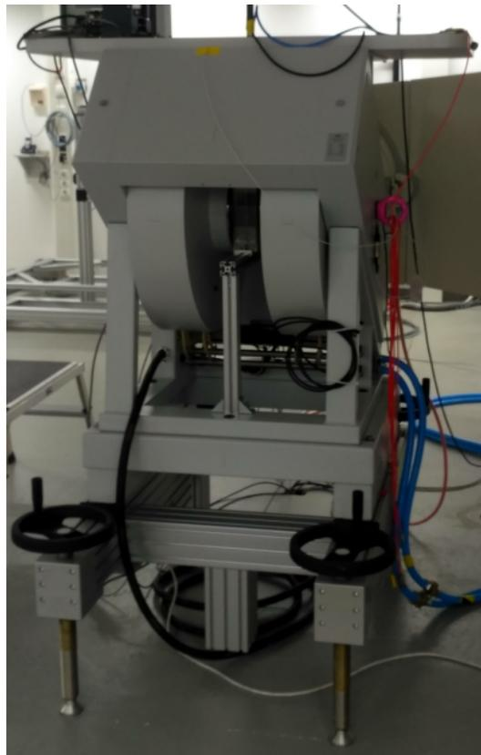
Figure 6.4: Electron paramagnetic resonance spectroscopy system at PTB.
