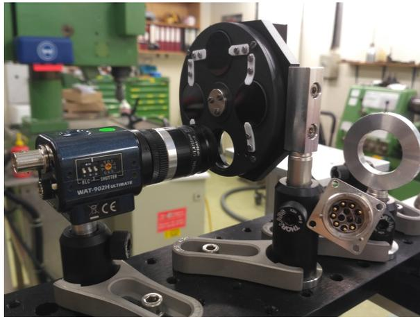
Figure 2.14: Monochrome CCD camera with filter wheel.
