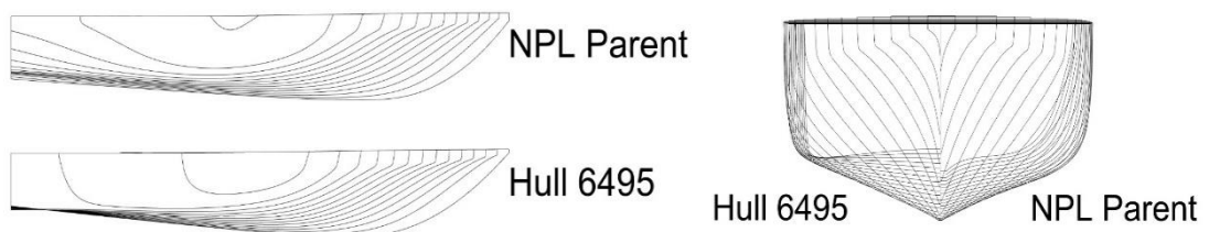
Figure 7-14 Comparison between sectional and buttock lines plans for hull 6495 and NPL parent hull
