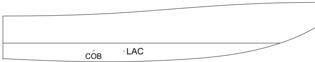
Figure 6-5 Longitudinal area coefficient diagram with highlighted centre of buoyancy
