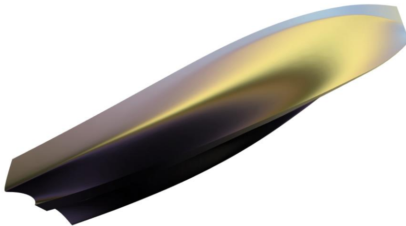
Figure 7-40 The baseline hull form visualised with an environmental map to highlight hull geometric curvature for greater ease of comparison
