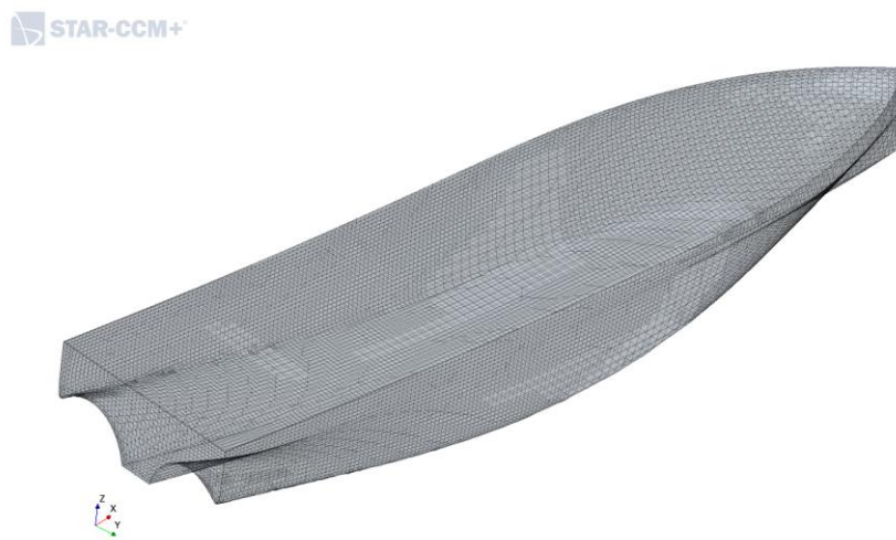
Figure 7-72 Hull 7971 surface mesh within Star CCM+
