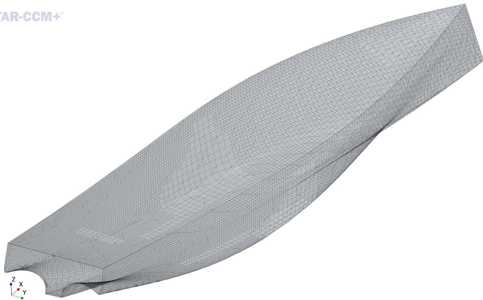
Figure 7-62 Hull 7828 surface mesh within Star CCM+
