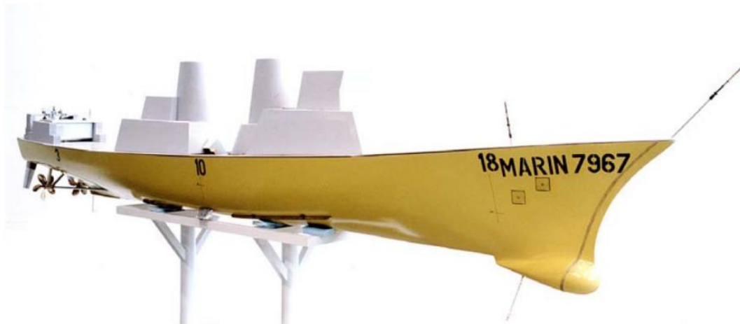
Figure 9-2 DTMB 5415 Free running hull model with superstructure (Toxopeu, et al., 2008)
