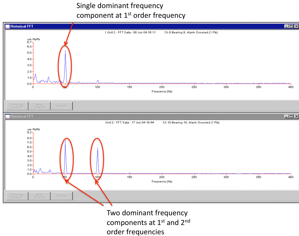
Figure 2.3: FFT plots captured from the Beran on-line condition monitoring system.
