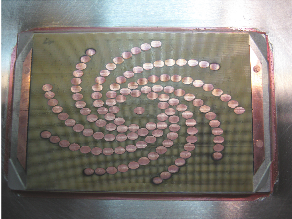
Figure 6-17 Rear face of the piezocomposite immediately after having its electrode applied. While there is some discoloration at the edge of the outer elements, these areas were still found to be conductive; the discoloration was an unwanted optical effect caused by the sputter process, and with further process development can now be avoided. The substrate is 70 x 50 mm, and the elements are 3 x 2 mm.
