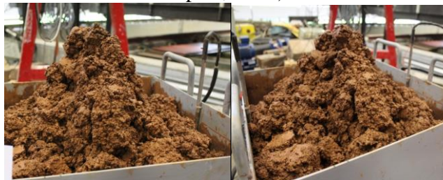
Figure 4 A Goethite sample before and after sea state test (TWG report, 2013)
