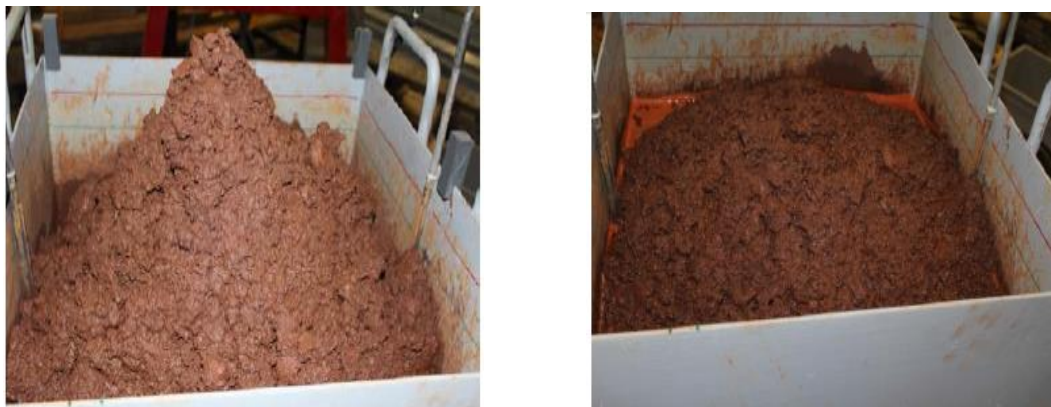
Figure 6.6 Iron ore piles before and after a sea state test (TWG report, 2013)
