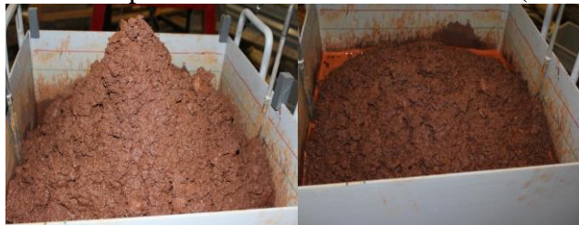
Figure 4 A Goethite sample before and after sea state test (TWG report, 2013)
