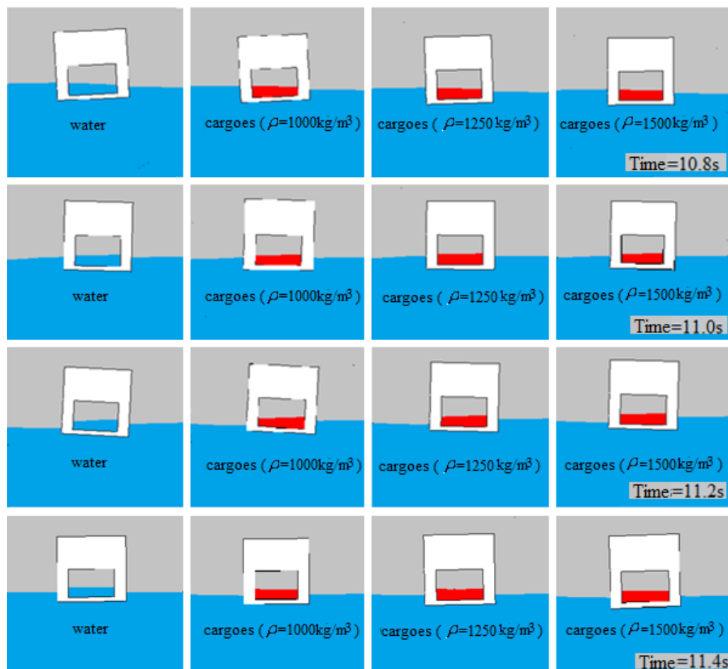
Figure 4.11 Contours of 2-D coupled motion in waves filled with water and non-Newtonian fluid (Time=10.8s, 11.0s, 11.2s and 11.4s)
