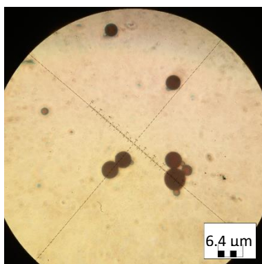
Figure 5-19. SPs of Cu-doped NPLs. PMMA: 30% of NPLs by mass. (Microscope objective \times 63 ).
