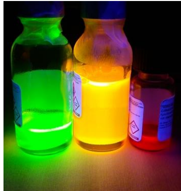
Figure 1-10. Picture of green (530 nm), yellow (575 nm) and red (630 nm) CQDs in solution taken from the laboratory. These CQDs all have nominally the same size (6 nm) but differ in alloy composition in the core.
