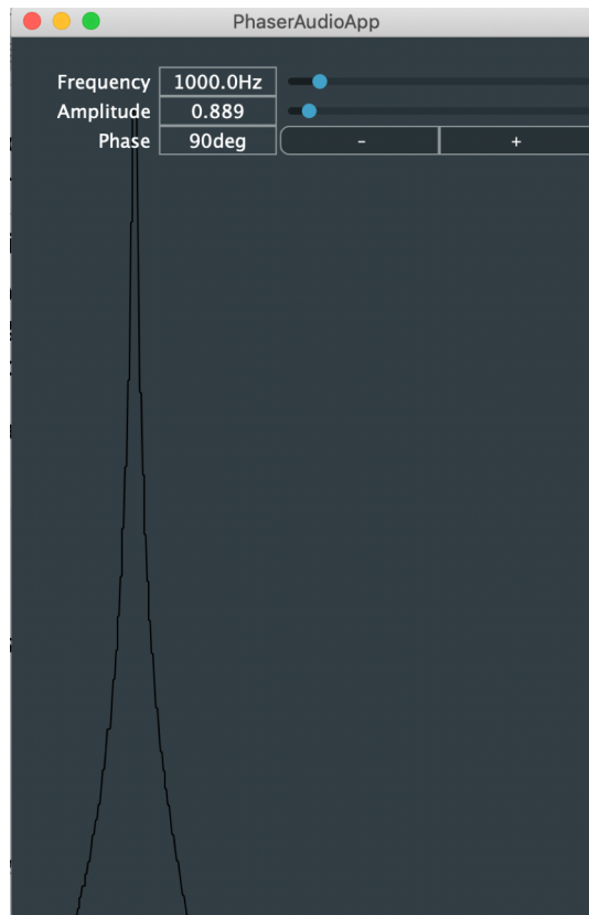
Figure 6.2: User Interface developed to measure the signal and control the phase and frequency of piezoelectric transducer in real-time.
