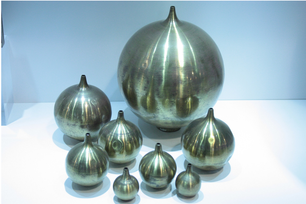
Figure 2.2: Helmholtz resonators made in 1870, Hunterian Museum and Art Gallery in Glasgow, source https://en.wikipedia.org .
