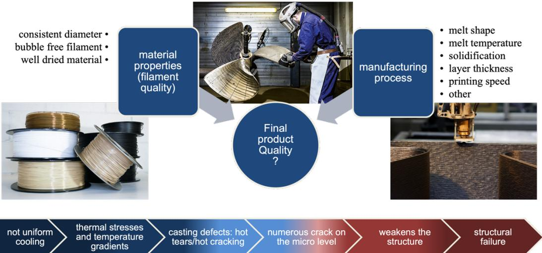
Figure 1.2 Process – induced (casting) defects due to layer-by-layer manufacturing [10].
