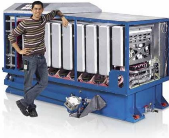
Figure 3.1: Transformer and rectifier device shown to indicate scale [9]
