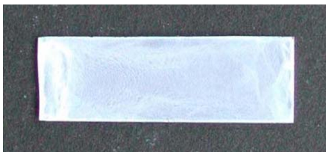
Figure 2-4 thick film of Degussa P25 deposited by repeated dip-coating in 5% aqueous slurry
