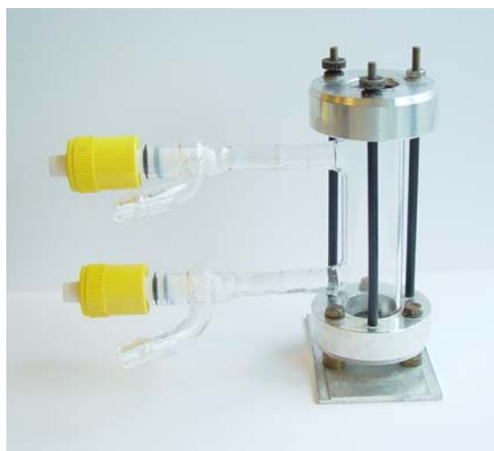
Figure 2-9 10cm gas-tight quartz cell fitted with quartz windows for UV-Vis analysis of gases
