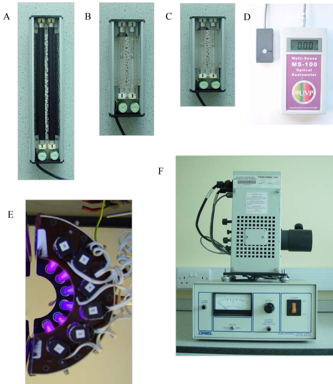
Figure 2-8 Apparatus for UV irradiation; A – 8W (with 2 × UVA); B – 6W (with 2 × UVC); C – 4W (with 2 × UVC); A, B and C supplied by Vilber Lourmat; D – PVP UV meter with detector; E – 6 × 8W (Lidam Scientific, with UVA bulbs); F – Xenon-Arc lamp (Oriol)
