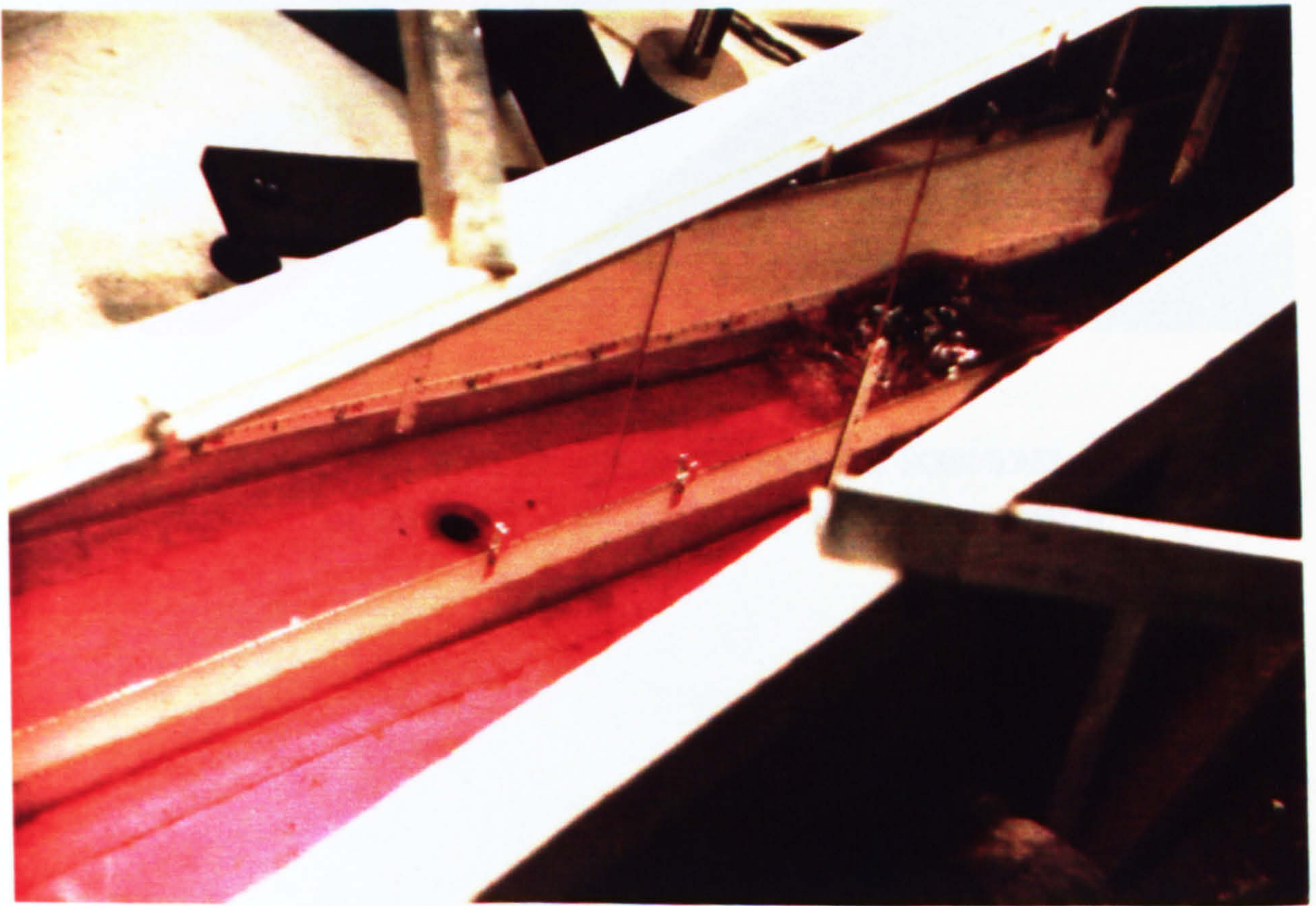
FIGURE 6.93 : PHOTOGRAPH OF THE WATER PROFILE DOWNSTREAM THE GATE IN THE ( XT - RT ) MODEL , H_1 = 15 cm AND H_0 = 1.5 cm.
