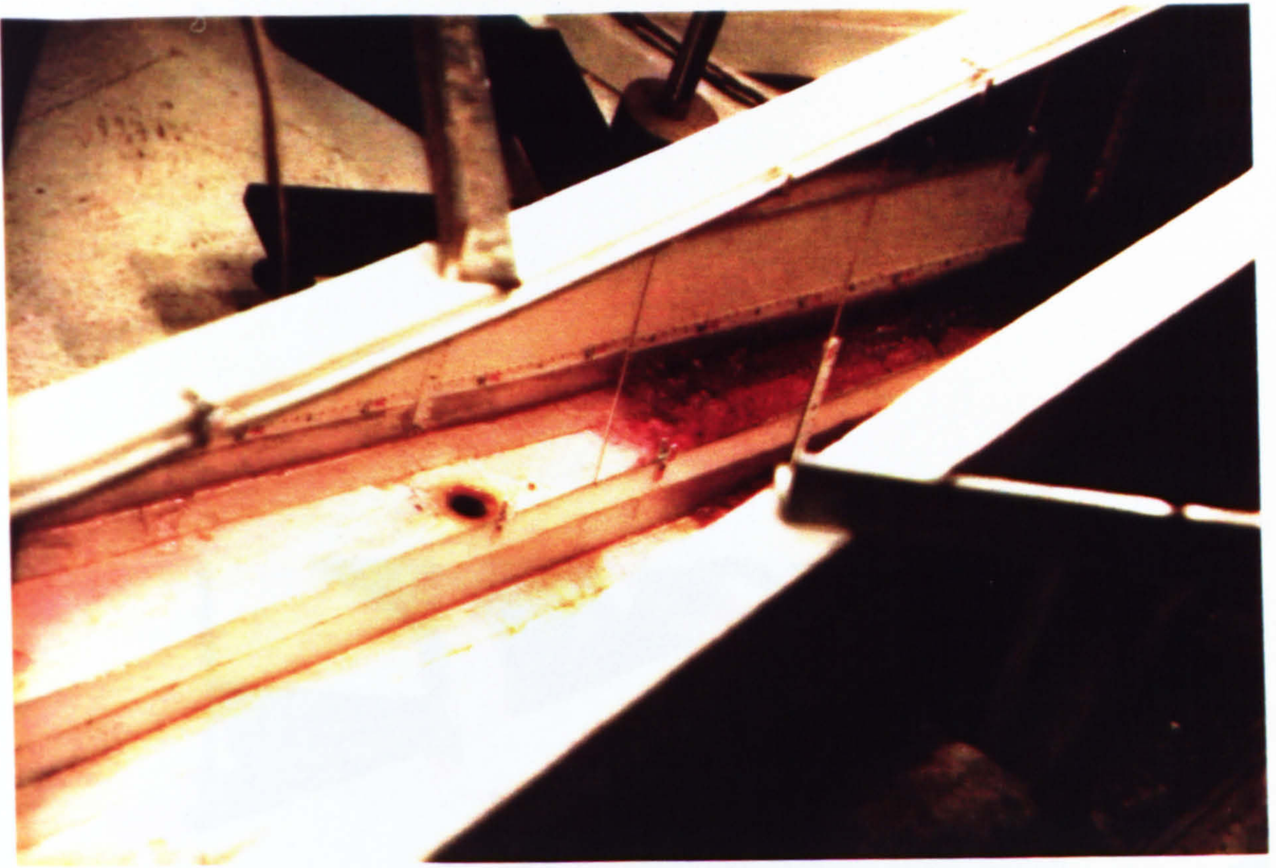
FIGURE 6.92 : PHOTOGRAPH OF THE WATER PROFILE DOWNSTREAM THE GATE IN THE ( XT - RT ) MODEL , H_1 = 15 cm AND H_0 = \text{DRY} .
