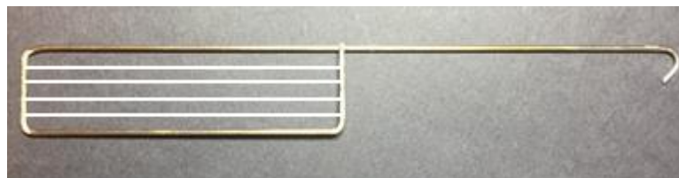
Figure B-4 Wire frame used for brief single fibre thermal conditioning with position of attached fibre drawn on
