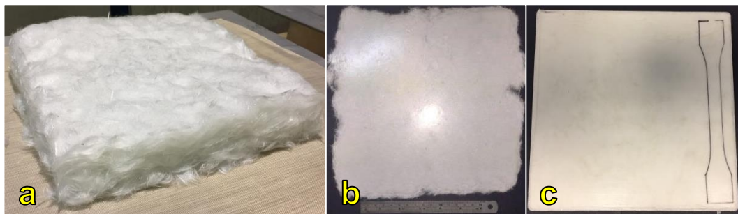
Figure 5-6 Various stages of GF-PP fabrication: a) dried GF-PP mat, b) preconsolidated layer, c) final compression moulded GF-PP laminate with tensile specimen geometry outlined
