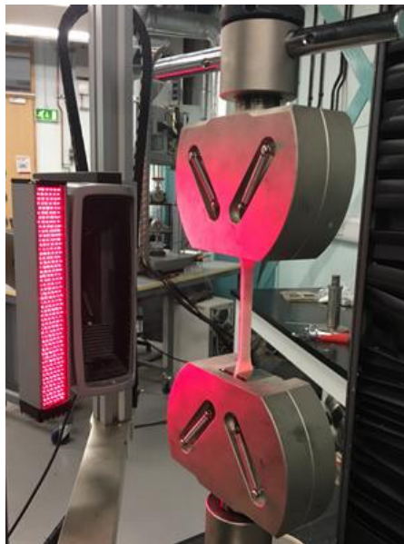
Figure 5-10 Tensile test set up on Instron 5969 testing machine
