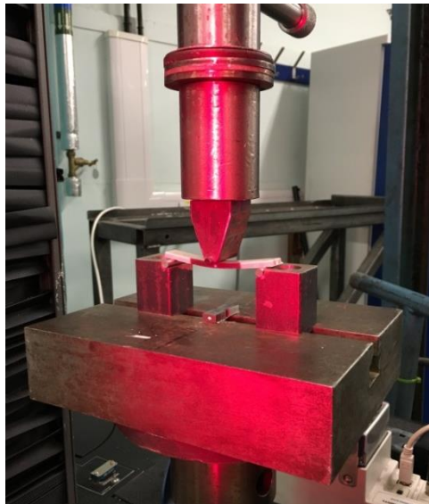
Figure 5-11 Three-point flexural test set up on Instron 5969 testing machine
