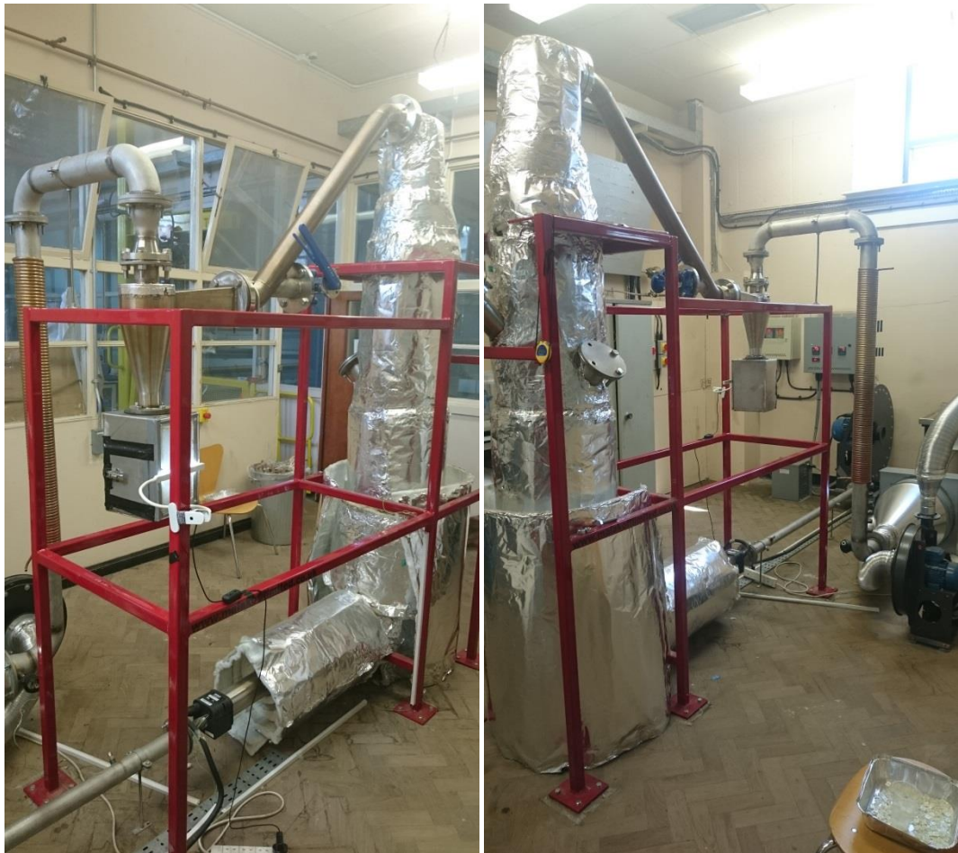
Figure 2-9 Images of the in-house developed fluidised bed recycling rig
