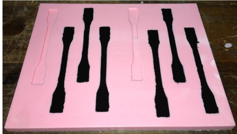
Figure 3-8 Silicone mould with epoxy+CuO specimens prior to curing
