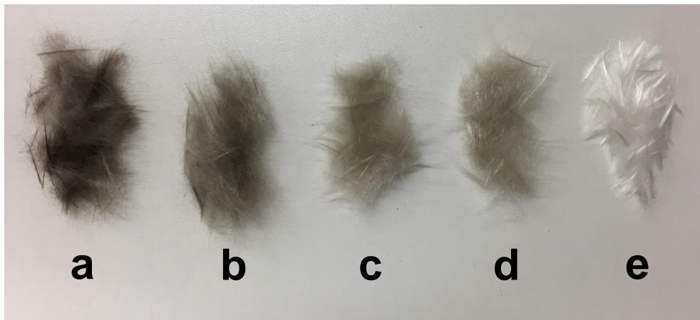
Figure 2-14 Glass fibres recycled in fluidised bed ( V_f=1.5 m/s) at a bed temperature of a) 400 °C, b) 450 °C, c) 500 °C, d) 550 °C and e) 500 °C + thermal cleaning at 550 °C for 60 min
