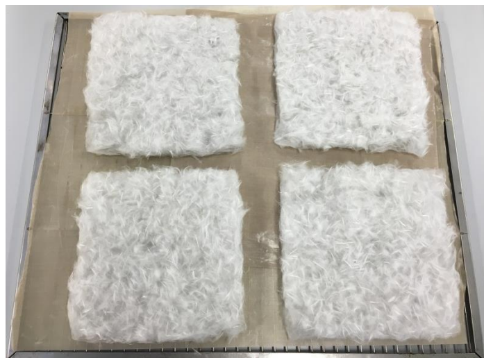
Figure 5-7 Randomly orientated discontinuous glass fibre mats used to prepare GF-EP with RGF
