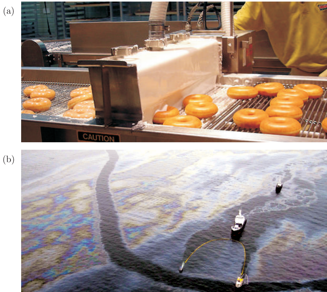
Figure 1.1: (a) Doughnuts passing through an enrober which coats each doughnut with a thin film of glaze; picture sourced from flickr.com/kathleenhaboc. (b) An oil spill in the sea; the oil floats on top of the water forming a thin film; picture sourced from NOAA Photo Library.
