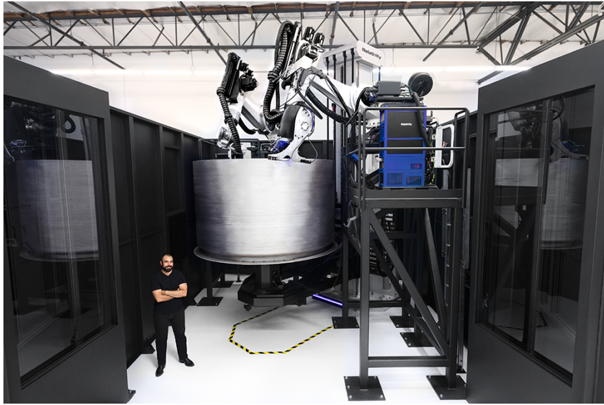
Figure 2.3: Relativity Space’s Stargate metal 3D printer manufacturing a cylindrical rocket section. Credit: Relativity Space.
