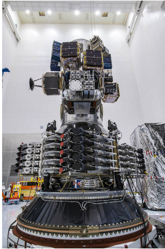
Figure 2.1: Payload stack of the Transporter-1 mission, photographed in the clean room before encapsulation in the fairing. Credit: SpaceX.
