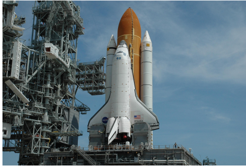
(a) Space Shuttle on the launch pad. The orbiter and the 2 solid rocket boosters were refurbished between flights. The orange external tank was demised, and not recovered. Credit: NASA.
