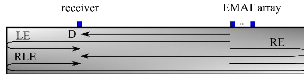
Figure 5.9. Schematic illustration showing wave propagation paths in pitch-catch configuration.
