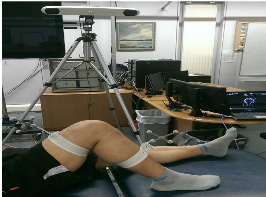
Figure 2.3: Passive navigation tracker clusters are secured to the thigh and leg with fabric strapping. The examination trolley is positioned so that the tested limb is approximately 2m from the camera, as per manufacturer's recommendations.
