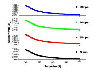
Fig. 10. Temperature dependence of sensitivity for the Co-catalyzed MWNTs-based film sensor in air and 40, 100, 140 & 200 ppm CO gas for the temperature range of (300500K).
