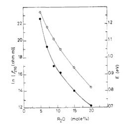
**Figure 2.** Dependence of both the resistivity ( $\bullet$ ) and the activation energy for conduction ( $\bigcirc$ ) on R<sub>2</sub>O (R<sub>2</sub>O = Na<sub>2</sub>O + CuO).
