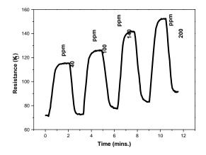
Fig. 4. Typical responses of Co-catalyzed MWCNTs gas sensor for different concentration of CO gas (40, 100, 140 & 200 ppm).
