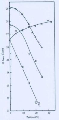
**Figure 1.** Dependence of  $\ln \rho_{350\%}$  on the ZnO content of the glasses 1 (0), 2 ( $\Delta$ ), 3 ( $\Box$ ) and 4 (×)
