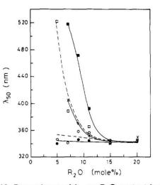
**Figure 10.** Dependence of  $\lambda_{50}$  on R<sub>2</sub>O content for samples treated thermally for 4 h at different temperatures ( $\bigoplus$ , 500 °C;  $\bigcirc$ , 520 °C;  $\times$ , 540 °C;  $\square$ , 560 °C;  $\blacksquare$ , 580 °C).
