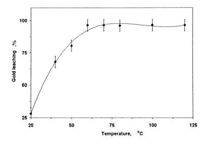
Fig. 2. Effect of temperature on the Au leaching (%) from the solid waste, 5h shaking time and 10ml/min chlorine gas.
