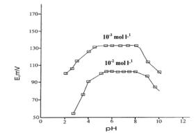
Fig. 4 Effect of the pH on the potentiometric response of the rhodamine-B chromate PVC membrane sensor.
