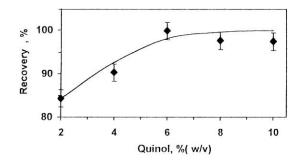
Fig. 7. Effect of quinol concentration (% (w/v)) on the Au recovery (%) from the stripped aqueous solution.
