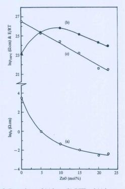
Figure 3. Dependence of (a)  $\ln \rho_{o}$  (b) E/KT and (c)  $\ln \rho_{350^{\circ}C}$  on ZnO content for the group 4 glasses
