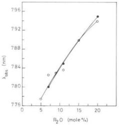
**Figure 6.**  $\lambda_{abs}$ , the wavelength of the absorption band, as a function of R<sub>2</sub>O content for untreated glasses ( $\bigcirc$ ) and glasses treated for 4 h at 560 °C ( $\bigcirc$ ).
