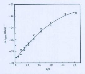
Figure 5. The natural logarithms of conductivity,  $\ln \sigma_{350^{\circ}C}$ , as a function of the oxygen to boron ratio of the glasses 2 ( $\Delta$ ), 3 ( $\Box$ ) and 4 (×)
