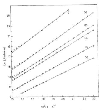
Figure 1. Resistivity-temperature dependence for glasses G1–G6.
