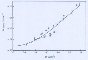
**Figure 9.** Change of  $\ln \sigma_{350^{\circ}C}$  with density of the glasses 1 (0), 2 ( $\Delta$ ), 3 ( $\Box$ ) and 4 ( $\times$ )
