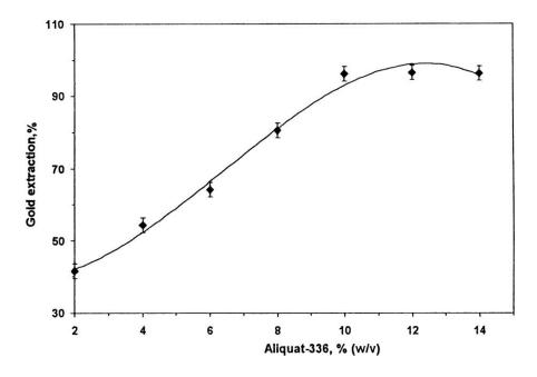
Fig. 6. Effect of aliquat-336 (% (w/v)) on the Au extraction from the leaching liquor at 1M HCl concentration.
