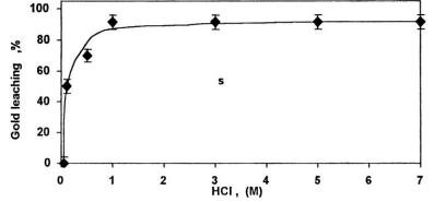
Fig. 1. Effect of HCl concentration (M) on the Au leaching (%) from the solid waste at 25 °C, 5h shaking time and 10ml/min chlorine gas.
