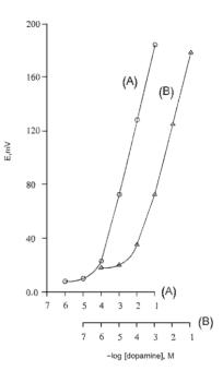
Fig. 2 Potentiometric responses of dopamine sensors CE-TPB (A) and CE-PTA (B).
