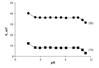
Fig. 3. Effect of pH on the potential response of barium(II)–Rose Bengal sensor  $10^{-3}$  M (A) and  $10^{-2}$  M (B).
