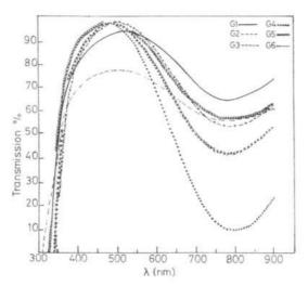
Figure 5. Spectral transmission of G1–G6, in UV and visible regions.
