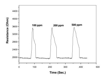
Fig. (6). Typical responses of MWCNTs gas sensor for different concentration of CO gas (100, 200 & 500 ppm).
