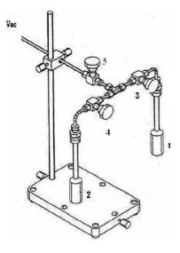
Figure 1. Apparatus for adsorption of pure solvent onto activated carbon.
