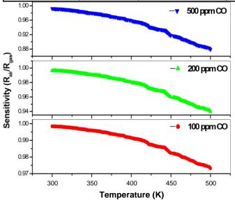
Fig. (8). Temperature dependence of sensitivity for the Fe-catalyzed MWNTsbased film sensor in air and 100, 200, & 500 ppm CO gas for the temperature range of (300-500K).
