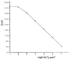
Fig. 3 Potentiometric response of the rhodamine-B chromate PVC membrane sensor.
