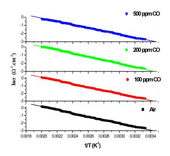
Fig. (9). Temperature dependence of conductivity for the Fe-catalyzed MWNTs- based film sensor in air and 100, 200, & 500 ppm CO gas for the temperature range of (300-500K).
