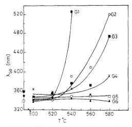
Figure 9. Effect of the heat-treatment temperature on  $\lambda_{50}$  of samples of G1–G6 treated for 4 h.
