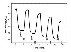
Fig. 6. Typical sensitivity of Co-catalyzed MWCNTs gas sensor for different concentration of CO gas (40, 100, 140 & 200 ppm).
