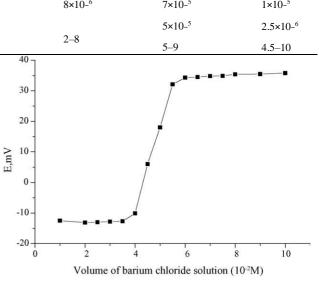
Fig. 4. Typical potentiometric titration curve for 15.0ml of sodium sulphate ( $10^{-2}$  M) with barium chloride ( $10^{-2}$  M) employing Ba–RB sensor.
