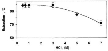
Fig. 5. Effect of HCl concentration (M) on the Au extraction (%) from the leaching with aliquat-336 (10% (w/v)) in kerosene. competition between the chloroaurate ion (AuCl<sub>4</sub>-)
