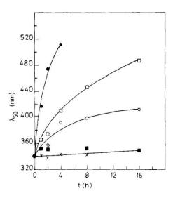
**Figure 8.** Effect of the heat-treatment time, at different temperatures, on  $\lambda_{50}$  of G2 (×, 500 °C; **I**, 520 °C;  $\bigcirc$ , 540 °C;  $\square$ , 560 °C; **O**, 580 °C).
