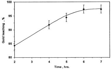
Fig. 3. Effect of shaking time (h) on the Au leaching (%) from the solid waste at 60-C, 1M HCl concentration and 10ml/min chlorine gas. percent of Au (Fig. 4) was increased by shaking the Au slime for 5h with the leachant up to 15g:100ml extraction could be proceeded as follows: pulp density and reached an approximate constant value.
