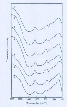
**Figure 10.** Infrared spectra of the glass samples (1) 10ZnO.40PbO.50B<sub>2</sub>O<sub>3</sub>, (2) 10ZnO.50PbO.40B<sub>2</sub>O<sub>3</sub>, (3) 60PbO.40B<sub>2</sub>O<sub>3</sub>, (4) 5ZnO.60PbO.35B<sub>2</sub>O<sub>3</sub>, (5) 10ZnO.60PbO.30B<sub>2</sub>O<sub>3</sub>, (6) 15ZnO.60PbO.25B<sub>2</sub>O<sub>3</sub> and (7) 20ZnO.60PbO.20B<sub>2</sub>O<sub>3</sub>
