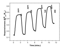
Fig. 5. Typical responsesiveness of Co-catalyzed MWCNTs gas sensor for different concentration of CO gas (40, 100, 140 & 200 ppm).
