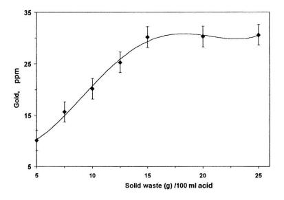
Fig. 4. Effect of pulp density (solid waste, g/100ml acid) on the Au leaching (ppm) from the solid slime at 60°C, 1M HCl concentration and 5h shaking time at 10ml/min chlorine gas.
