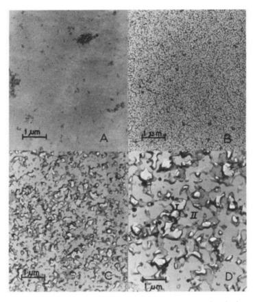
Figure 3. Electron micrographs of G2: A, as obtained after annealing; B, after 1 h at 560 °C; C, after 4 h at 560 °C; D, after 8 h at 560 °C.
