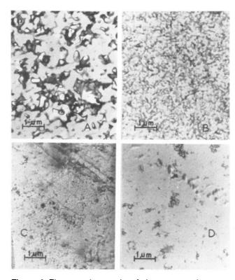
Figure 4. Electron micrographs of glasses treated thermally for 8 h at 560 °C: A, G3; B, G4; C, G5; D, G6.
