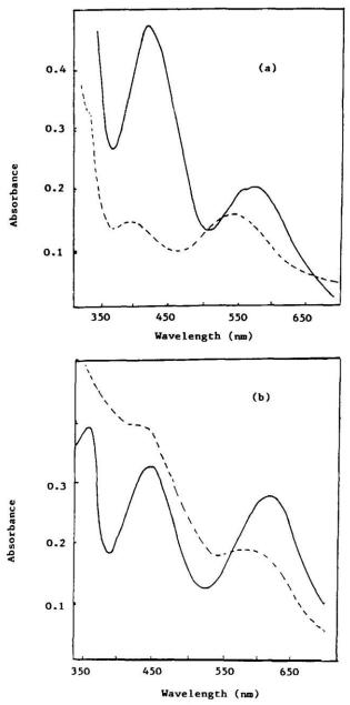
Fig. 2. Electronic spectra of (a)  $Cr(Cys)_3$ , — and  $[Cr(-Cys)_2Cl]_2$ , … and (b)  $Cr(Cyst)_3$ , — and  $[Cr(Cyst)_2Cl]_2$ , … .
