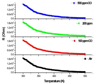
**Fig. (7).** Temperature dependence of resistance for the Fe-catalyzed MWNTsbased film sensor in air and 100, 200, & 500 ppm CO gas for the temperature range of (300-500K).
