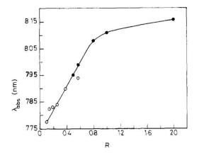
**Figure 7.** Change of  $\lambda_{abs}$  with *R* value of sodium borosilicate glasses; ( $\bigcirc$ ) the present results and ( $\bigcirc$ ) data taken from Shen *et al* (1982).
