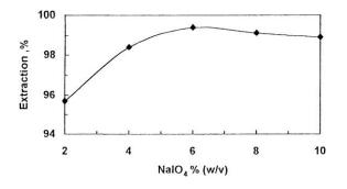
Fig. 8. Effect of NaIO<sub>4</sub> concentration (% (w/v)) on the Sb extraction (%) from the leaching liquor.
