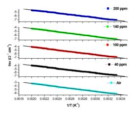
Fig. 8. lnσ versus 100/T for the Co-catalyzed MWNTs-based film sensor in air and 40, 100, 140 & 200 ppm CO gas for temperature range of (300-500K).
