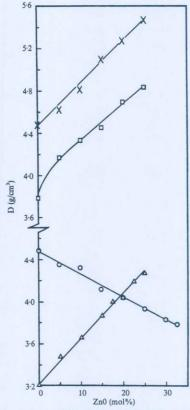
Figure 6. Dependence of density on the ZnO content of the glasses 1 (0), 2 ( $\Delta$ ), 3 ( $\Box$ ) and 4 ( $\times$ )
