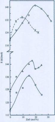
**Figure 2.** Change of activation energy with ZnO content of the glasses 1 (0), 2 ( $\Delta$ ), 3 ( $\Box$ ) and 4 (×)
