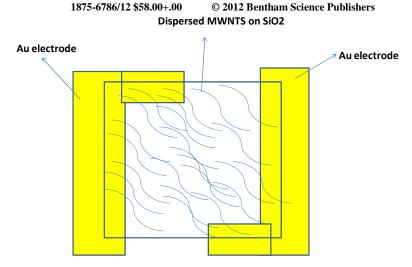
Fig. (1). Electrode pattern of MWNTs film sensor.
