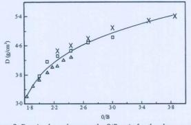
Figure 8. Density dependence on the O/B ratio for the glass samples 2 ( $\Delta$ ), 3 ( $\Box$ ) and 4 (×)
