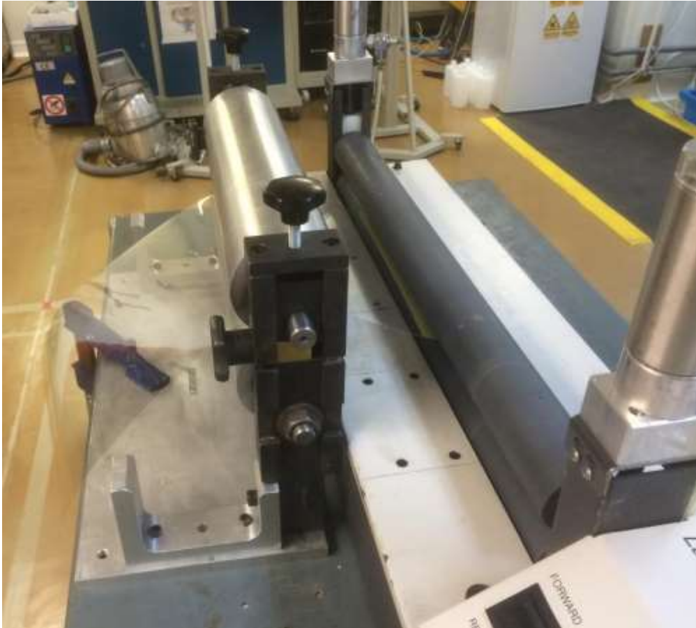
Figure 2.04: Lamination set-up used for the application of polyurethane adhesives.
