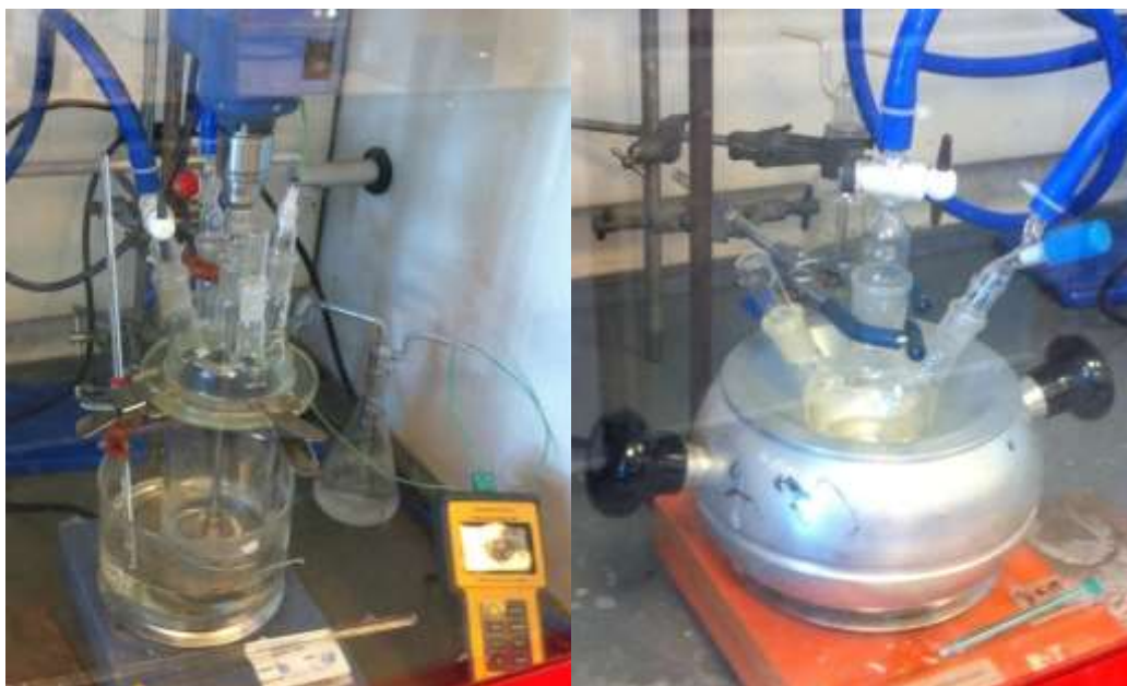
Figure 2.03: Apparatus used in synthesis of polyurethane adhesives. (a) Reaction kettle complete with nitrogen inlet/outlet, overhead mechanical stirrer, thermocouple, addition port and (b) three necked round bottom flask for preparation of isocyanate.
