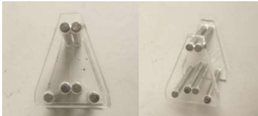
Figure 2.15: 180° T-peel roller system used to ensure correct angle obtained during testing on laminates containing different ply materials.
