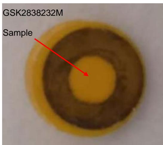
**Figure 5.17:** Powder GSK2838232M sample mounted in metallic washer between sticky Kapton film.
