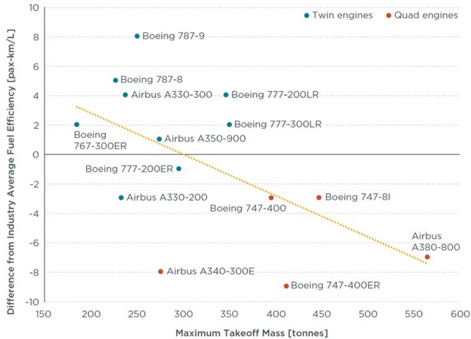
Figure 1.4: Difference From Industry Average Fuel Efficiency for 14 Aircraft Types, 2016 [21]
