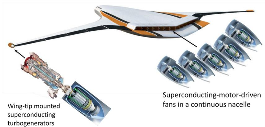
Figure 1.5: NASA N3-X Aircraft Concept [23]
