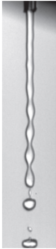
Figure 1.31: A cylindrical jet of fluid emanating from a nozzle experiences the Rayleigh–Plateau instability and breaks up into a stream of beads. Adapted with permission, Copyright 2020, Speirs et al. [186].
