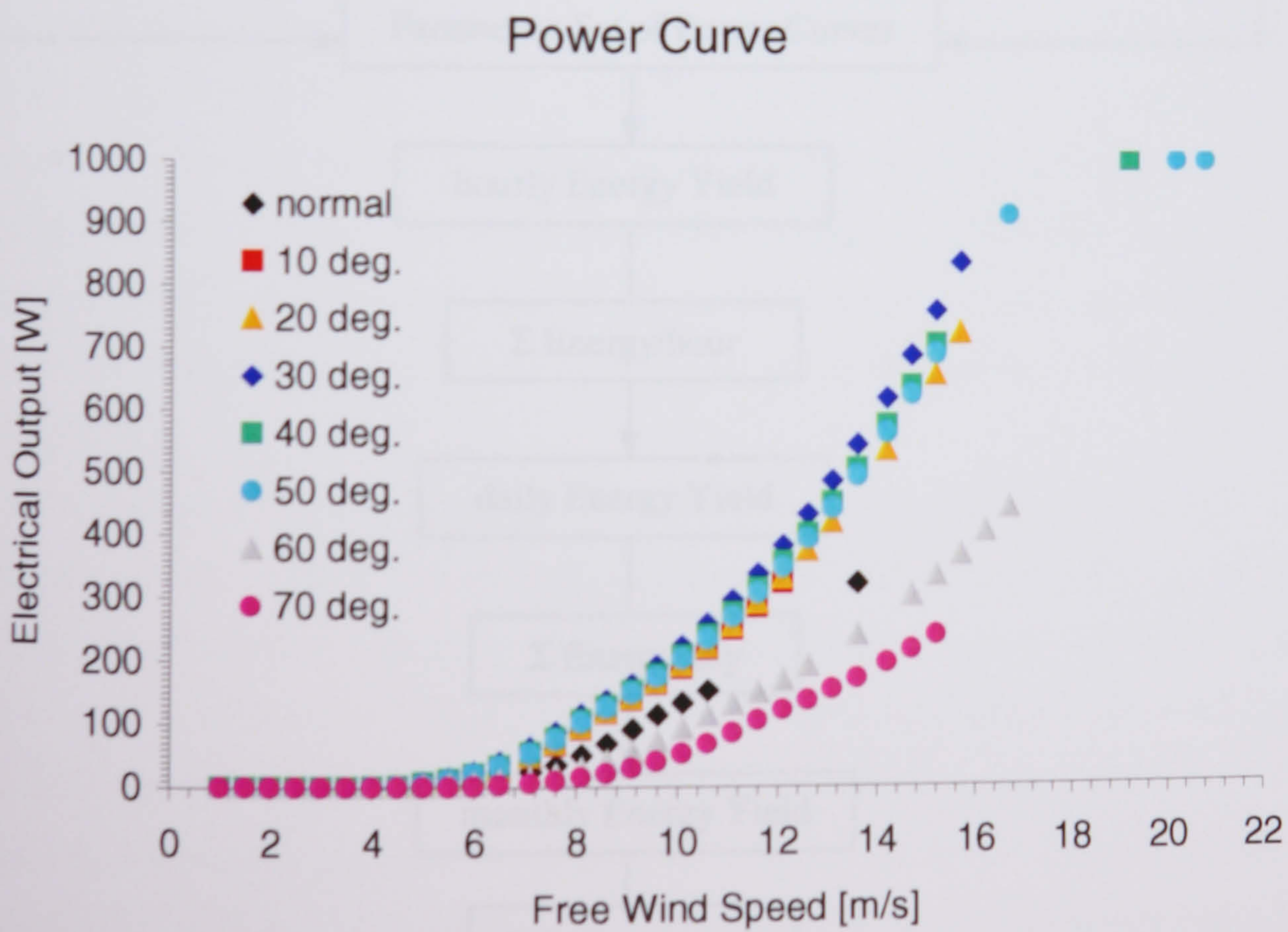
Figure 8.2.3: Modelled power curve for the configuration of experiment 6 ( 90^\circ duct, spoiler II). Parametric set for various angles of incidence
