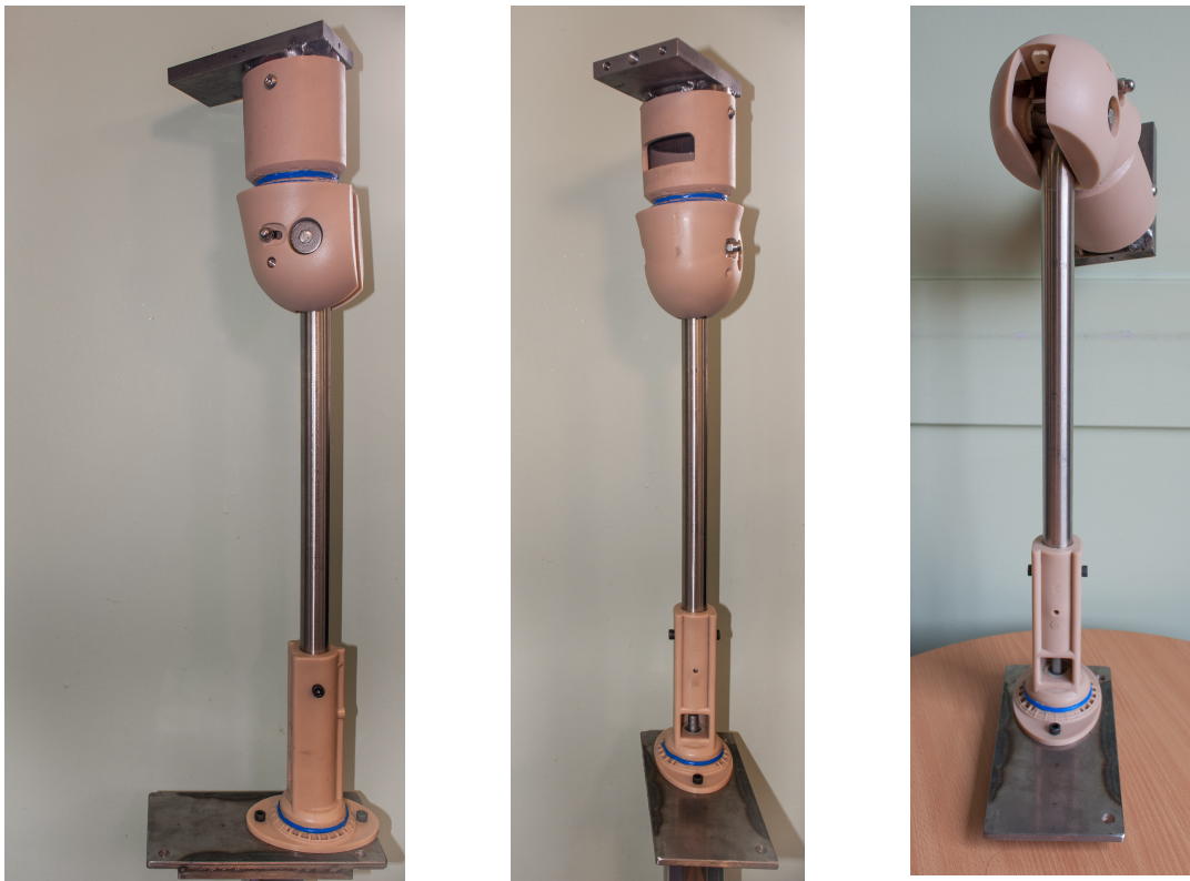
Figure 4.10: The whole assembly fully extended in the sagittal plane (on the left), fully extended in the coronal plane (in the centre) and fully flexed in the coronal plane
