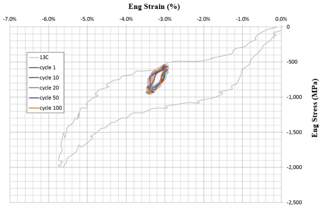
Figure 3-18: Cyclic stress-strain behavior of 1mm NiTi wire at 37 C in compression: 100 cycles at 0.4 % peak-to-peak \Delta\varepsilon during unloading (Test Set 13, sample 13C)
