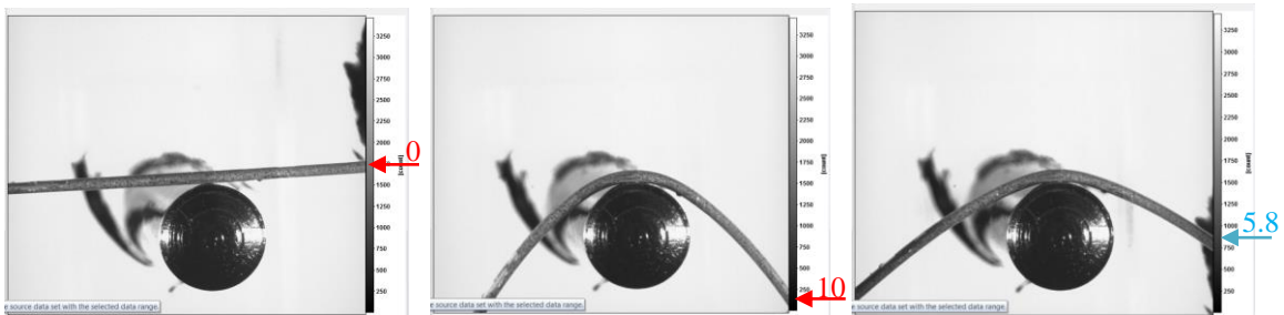
Figure A3-10: zoomed-out ‘macro’ CCD images of wire in 3-Point Bending. Left image shows initial pin position; middle image shows known ‘maximum deflection’ pin position; right image shows interpolated intermediate pin position
