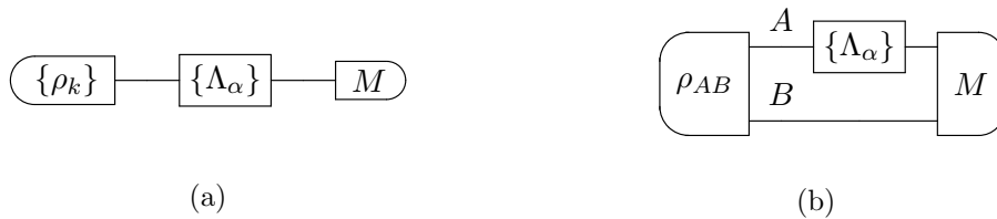
Figure 4.1: Two strategies for distinguishing channels. (a) No ancilla is used: a probe undergoes one of many possible quantum evolutions described by channels \{\Lambda_\alpha\} , and is later measured (box M ). Many different input states \{\rho_k\} are in general needed to discriminate between arbitrary channels, if one cannot tailor the input to the channels. (b) ancilla-assisted: the probe A is correlated with an ancilla B ; the output probe and the ancilla are jointly measured. Depending on the initial probe-ancilla correlations, it might be possible to distinguish between arbitrary evolutions, without modifying the input.
