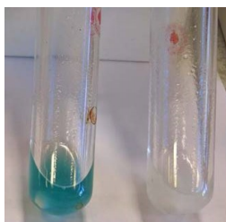
Figure 6.4: Reactions of benzophenone with \text{KO}^t\text{Bu} in benzene, left - exposed to 400 nm LEDs, right - not exposed to light.
