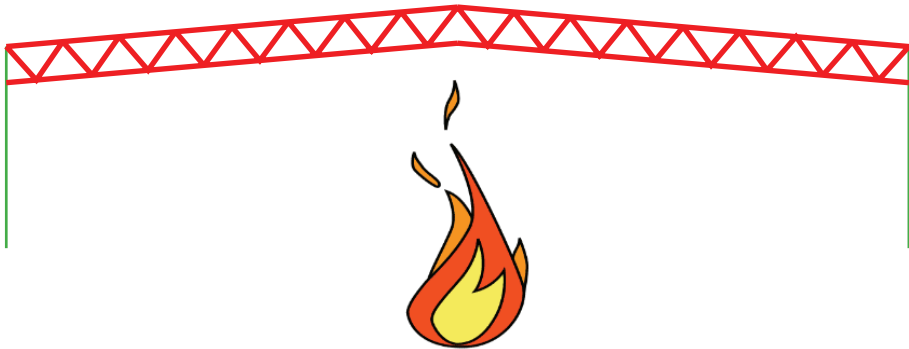
Figure 5.66: Fire scenarios for standard portalised truss frame. Thick red indicates members in fire and thin green indicates member at ambient temperature.
