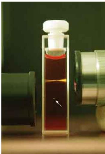
Figure 1.17: A comparison between confocal and two-photon excitation of fluorescence. In confocal stimulation, shown in the upper half of the cuvette, fluorescence from out-of-focus planes is generated at first and then filtered out at the detector. In two-photon stimulation, fluorescence is generated only in a confined volume around the focal position; the two-photon spot is indicated by the arrow.
