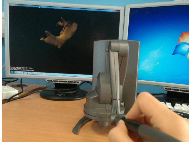
Figure 5-30 Experimental setup for the dental surgery simulation
