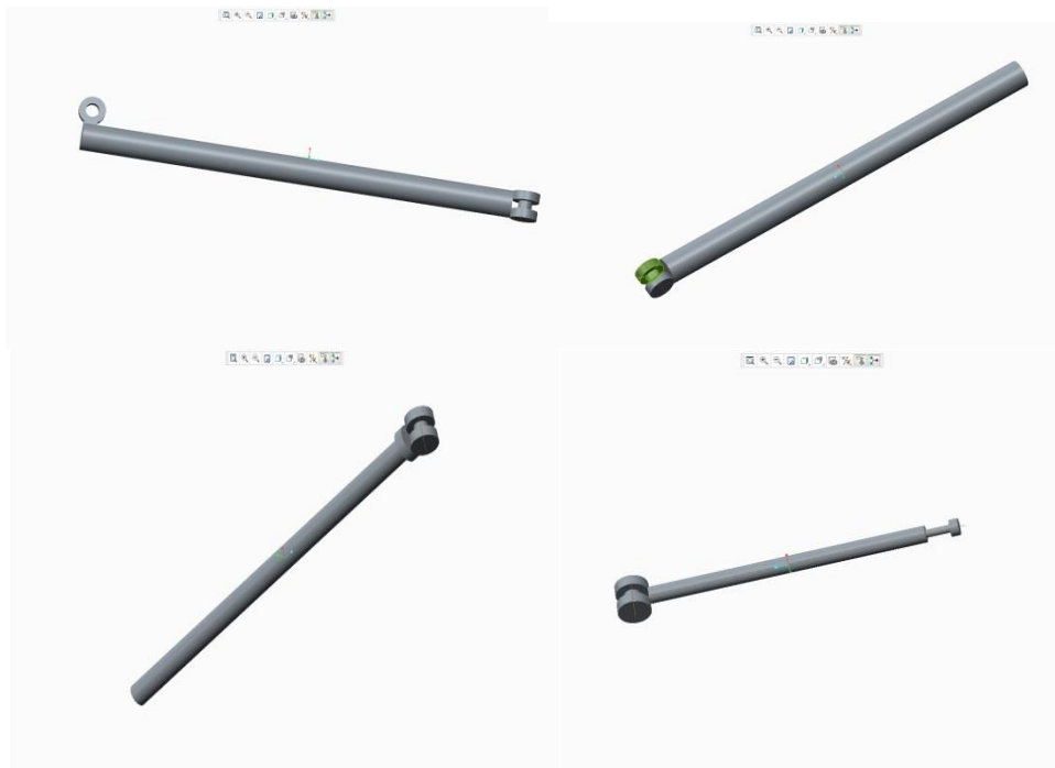
Appendix 1 Beams of the robotic arm
