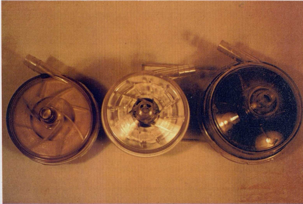
Figure 2.2: Aries Medical Isoflow TM , Sarns/3M Delphin TM and Medtronic Bio-Pump TM (from left to right).
