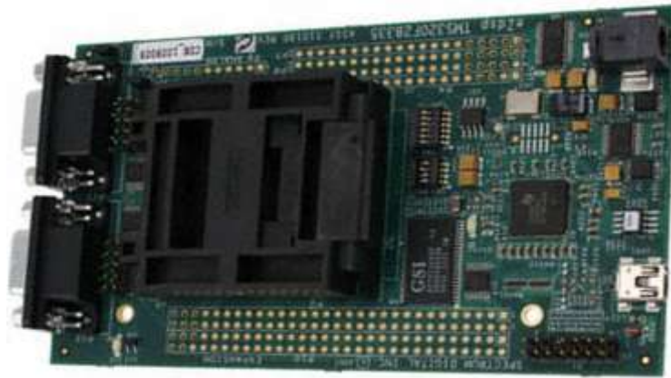
Figure C.2. eZdsp™ F28335 board
