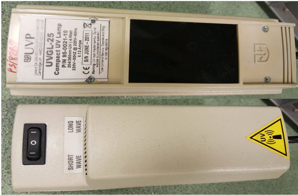
Figure 3.9 UVP UVGL-25 UV lamp used for the exposure of bacterial suspensions and bacteria seeded on surfaces UV-C light.
