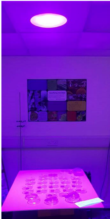
Figure 3.8 The experimental arrangement for the 405 nm light exposure of C. difficile spores inoculated onto surfaces. The irradiance was measured at each sample position on the board, with a 0.4 \text{ mWcm}^{-2} irradiance average.
