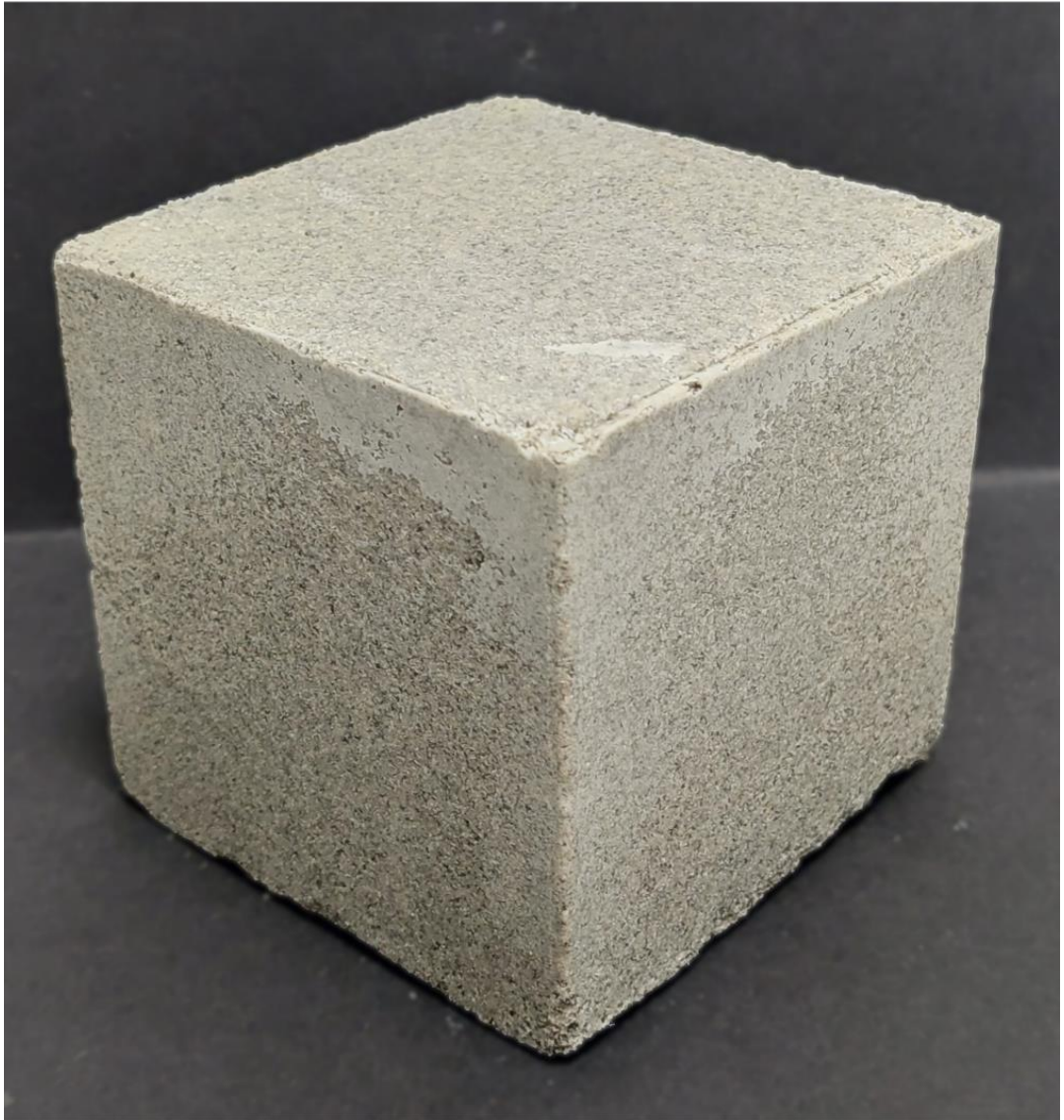
Enzyme induced bio-block, Glasgow – August 2024
