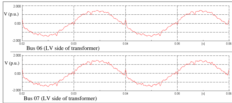
(b) Voltage waveforms of non-linear loads at LV side of bus 6 and 7
