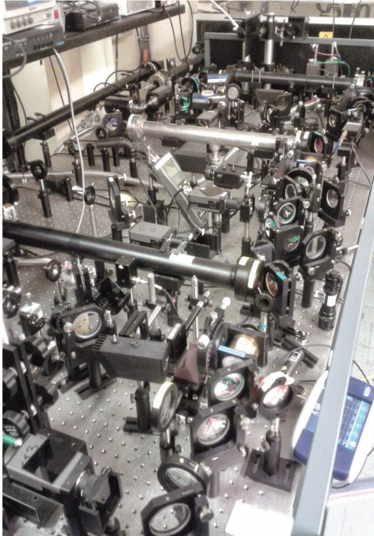
Figure A.8: Three stage nano-second OPCPA system used on the petawatt beam line
