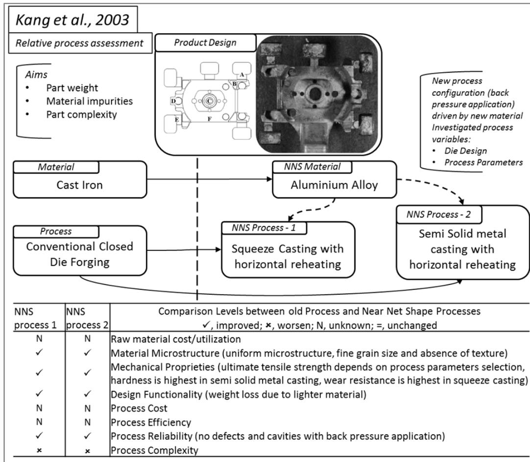
Figure A.5: Schematic representation of Kang et al. [2003] experimental paper on aluminum carter squeeze casting (old process, material, product design and new NNS tested process and material; investigation aims; NNS variables developments and comparison levels between new and old NNS process).
