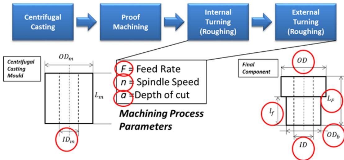
Figure 6.12: Valve cage manufacturing optimization: schematic of process parameters and design variables.
