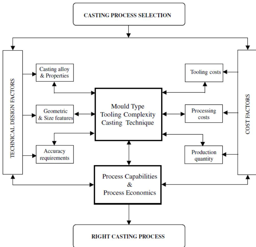
Figure 2.8: Casting process selection parameters and their interactions [Er and Dias, 2000].
