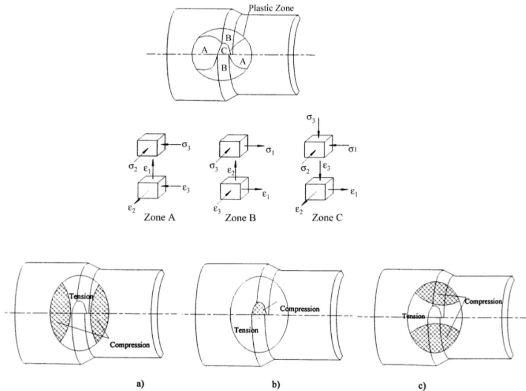
Figure D.3: Schematic diagram of stress and strain in various regions (top). Distribution of deformation in various direction: (a) axial direction; (b) radial direction; (c) tangential direction [Xu et al., 2001b].
