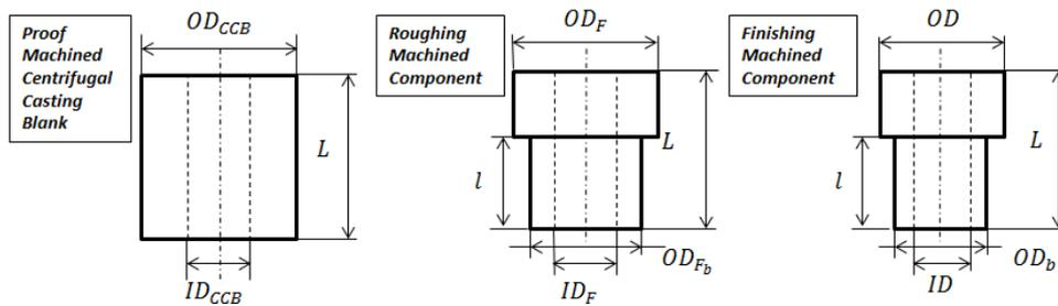
Figure 6.2: CAD representation of the valve cage and schematic of its nomenclature.
