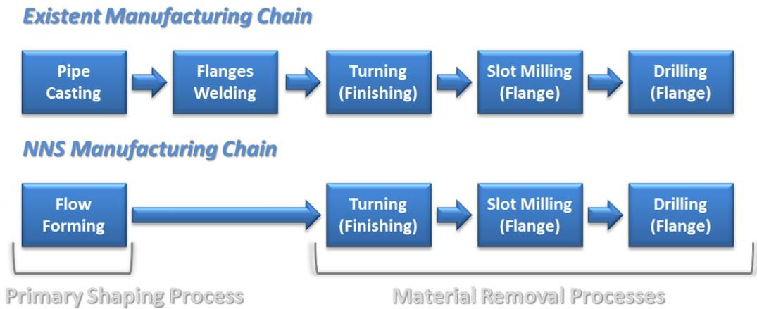
Figure 5.7: Comparison between existent (top) and NNS (bottom) manufacturing chains of the Case Study IA.
