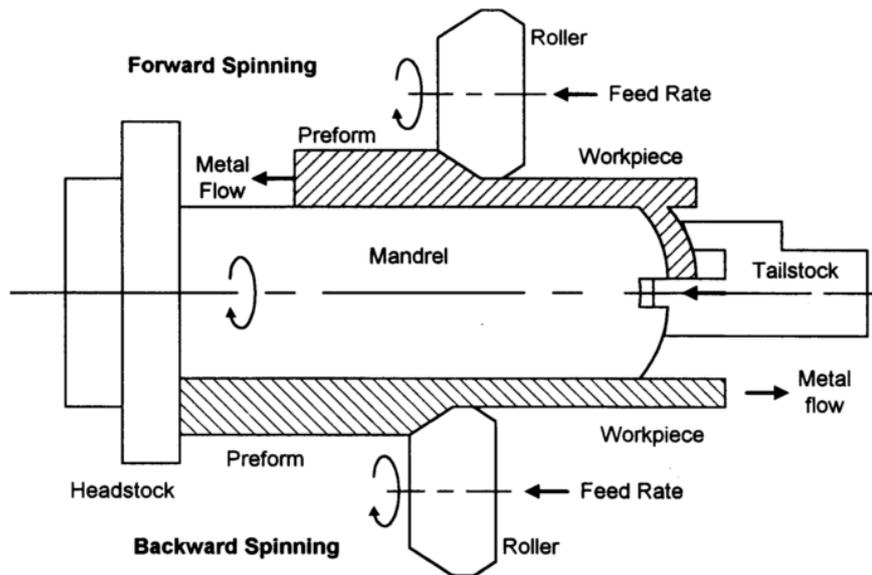
Figure 5.1: A schematic illustration of Flow forming [Chang et al., 1998].
