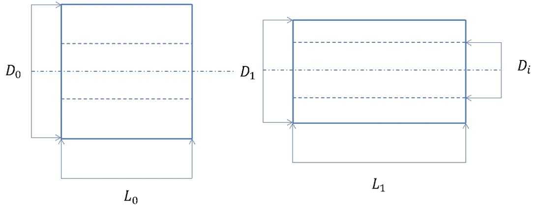
Figure E.1: Volume constancy for a simple pipe.
