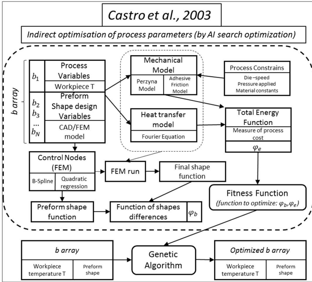
Figure A.2: Schematization of the Castro et al. [2004] Genetic Algorithm for optimizing closed hot die forging process in terms of preform shape and process temperature.
