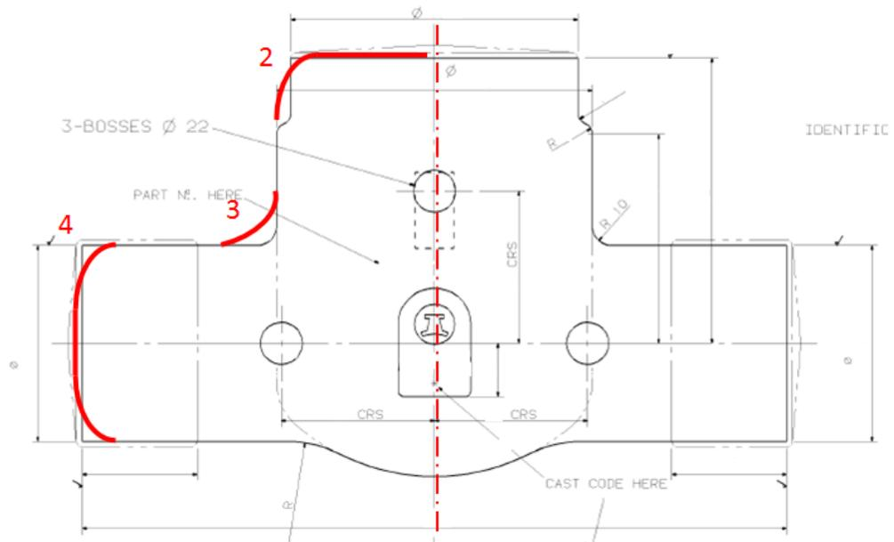
Figure 7.5: Schematic of the parallel gate valve, including the considered design variables (2, 3, 4).
