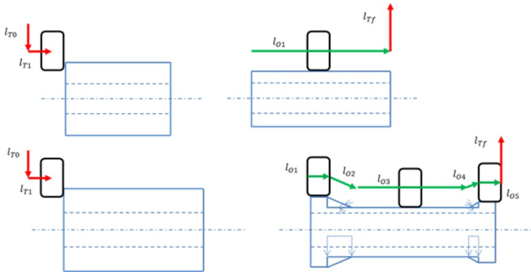
Figure 5.13: Flow forming time model schematization for hollow tube (up) and flanged pipe (down).
