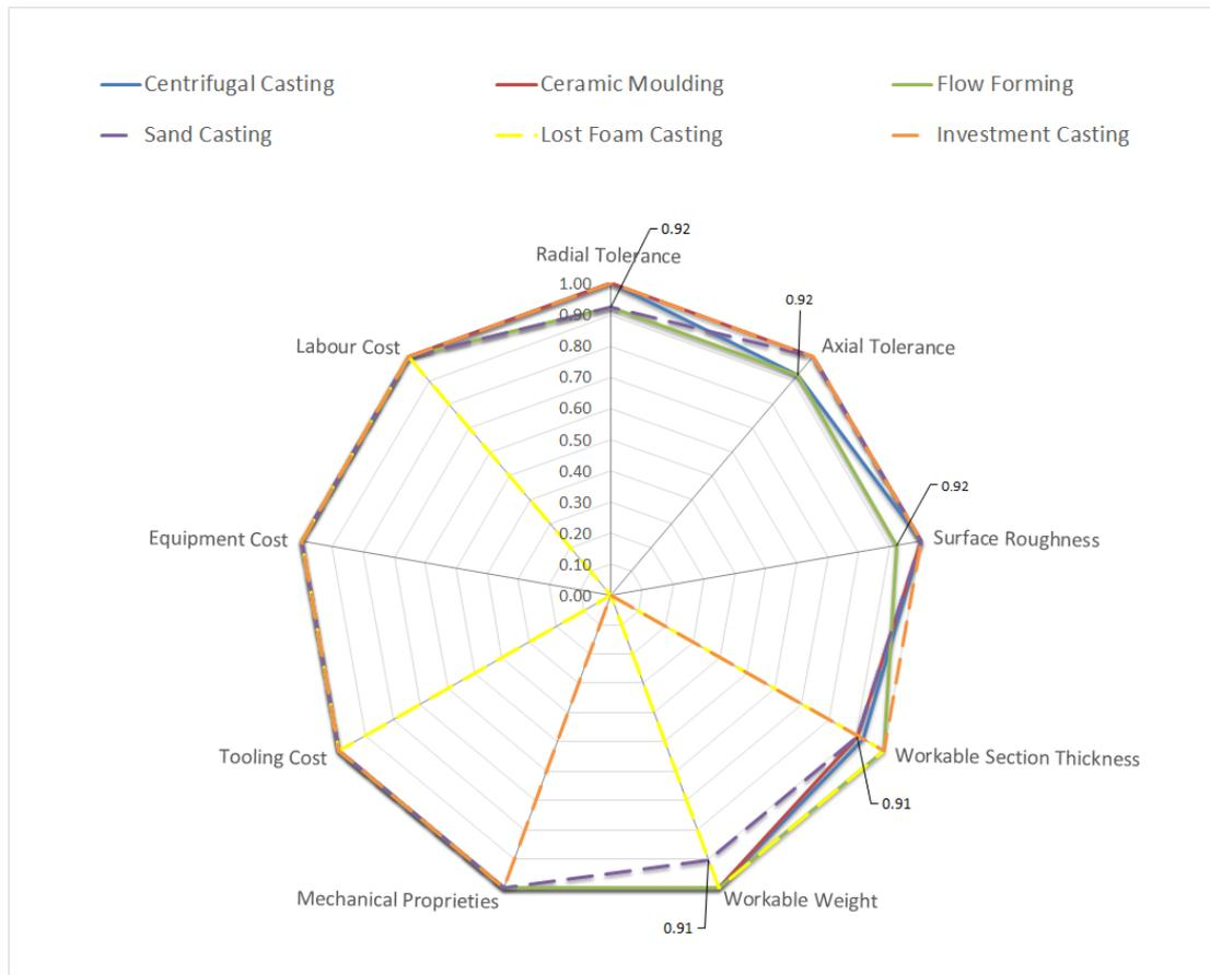
Figure 4.15: Process compatibilities breakdown for the Case Study II.
