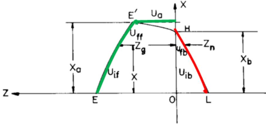
Figure E.4: Definition of the contact zone for the case-study:  $z_g(z > 0)$  in red and  $z_n(z < 0)$  in green.
