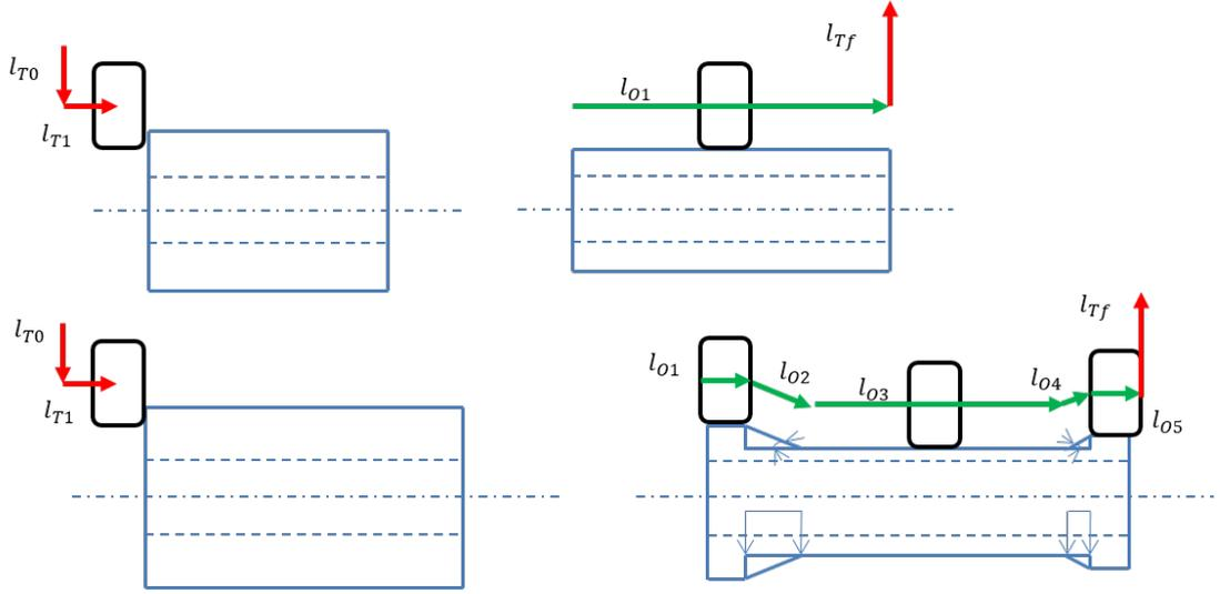
Figure E.5: Precess-time modelling for simple pie (up) and flanged pipe (down). Schematic of flow forming tool-path: transverse motion (red) and forming motion (green)
