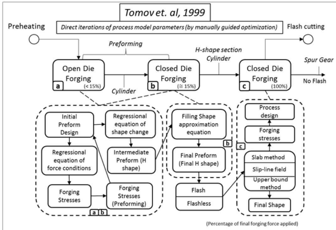
Figure A.1: Schematization of Tomov and Gagov [1999] procedure for analytical optimization of forging process.
