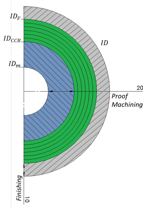
Table F.6: External turning process scheme and nomenclature scheme (grey: finishing zone; green: roughing zone; blue: proof machining zone).
