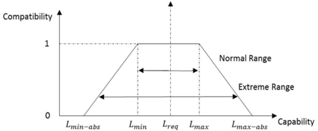
Figure 2.6: Fuzzy set for process capabilities (adapted from Ravi [2005]).
