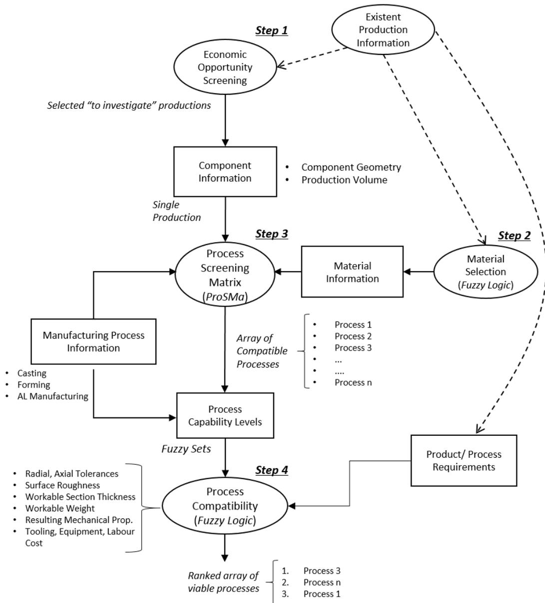
Figure 3.2: Product Geometry, Manufacturing and Material Matching (ProGeMa3) Methodology schematic.
