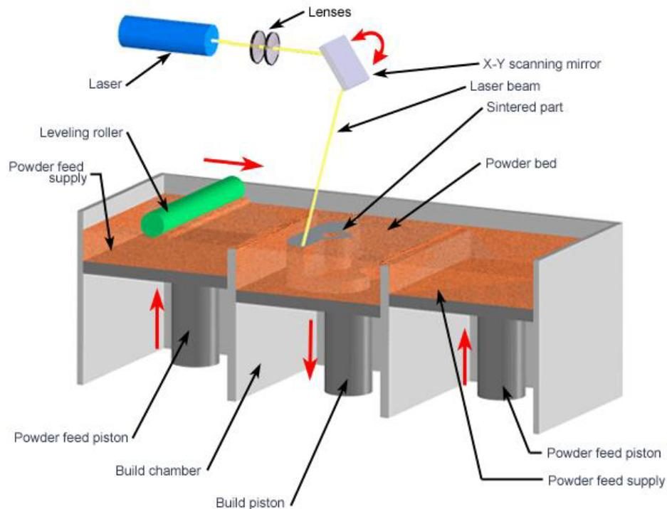
Figure B.5: Schematic of Direct Metal Laser Sintering process [Esmailian et al., 2016].
