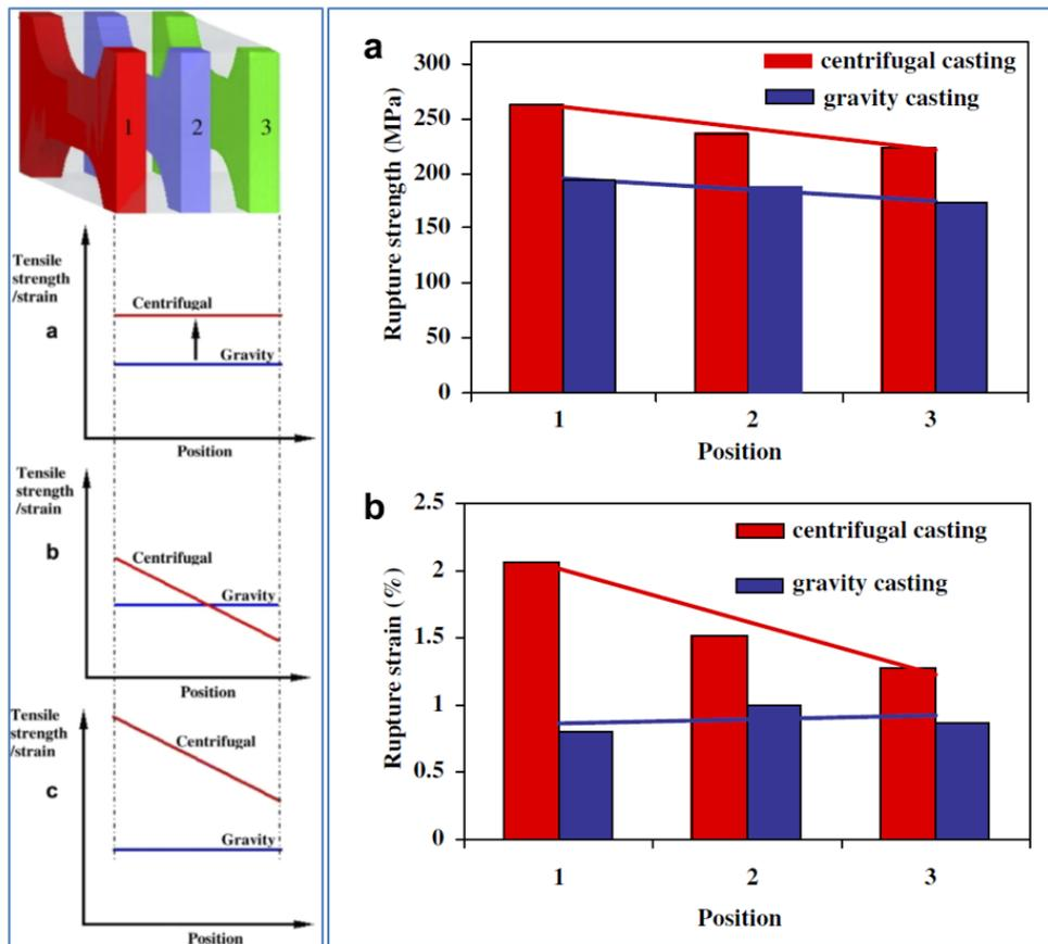
Figure D.6: Left - (a) Ultimate strength and (b) rupture strain results for both centrifugal and gravity castings in different positions of the casting- Right - Scheme of the mechanical properties variation with the following variables: (a) vibration or fluid dynamics; (b) centrifugal pressure; (c) combined effect of (a) and (b). Adapted from Chirita et al. [2008].
