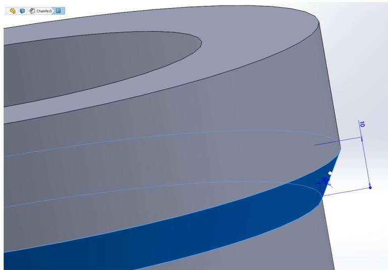
Figure 5.10: Chamfer design modification for adapting to flow forming process.
