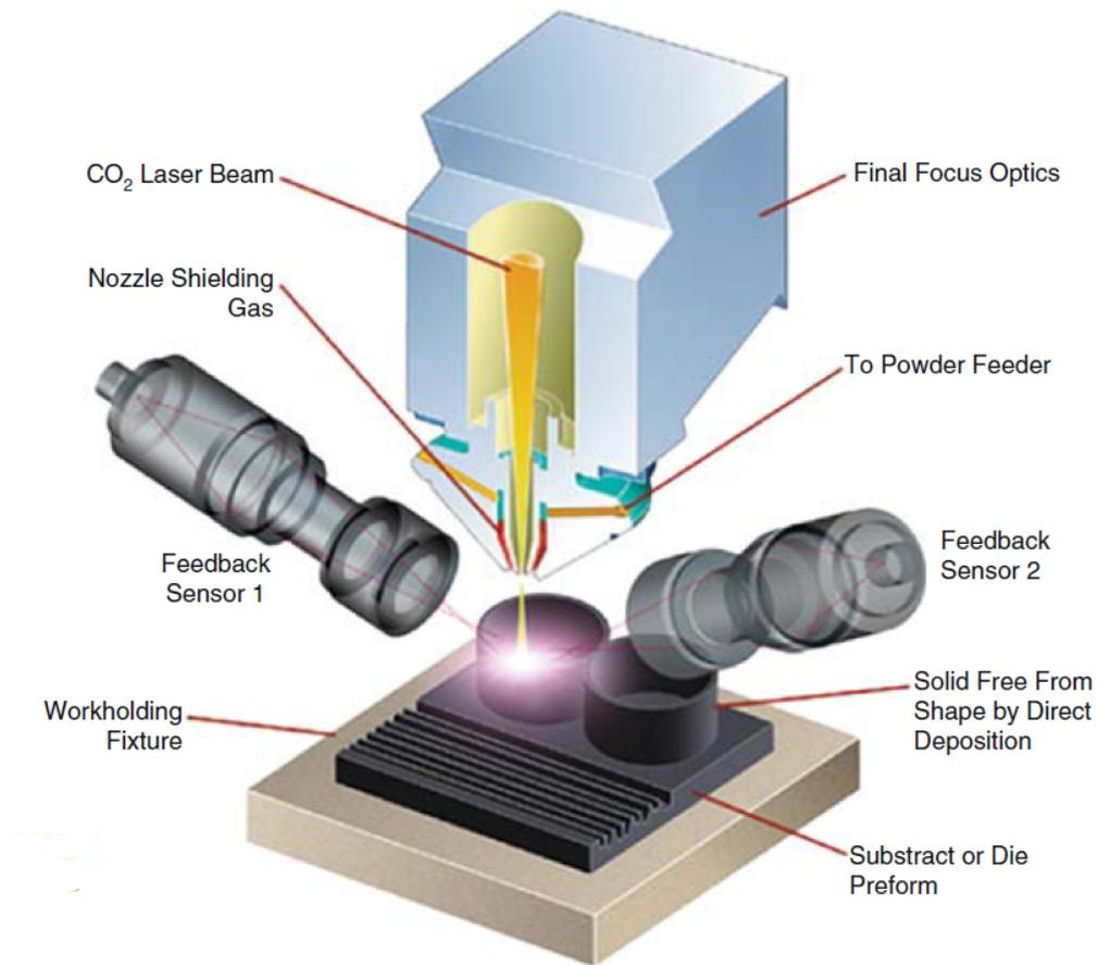
Figure B.6: Schematic of a Direct Energy Deposition process [Esmailian et al., 2016].
