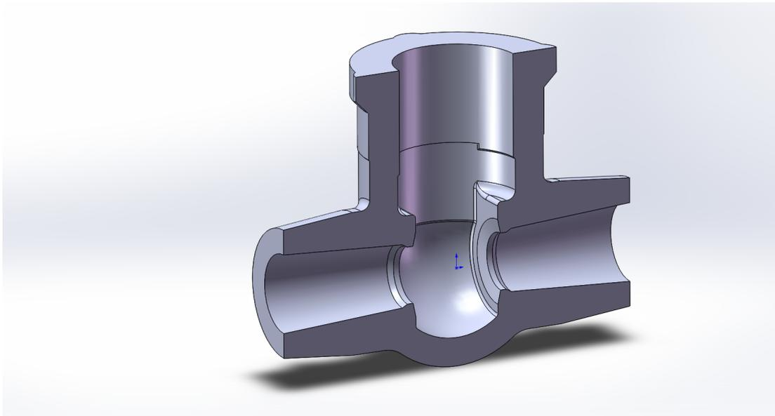
Figure 7.3: Body of a parallel gate valve.
