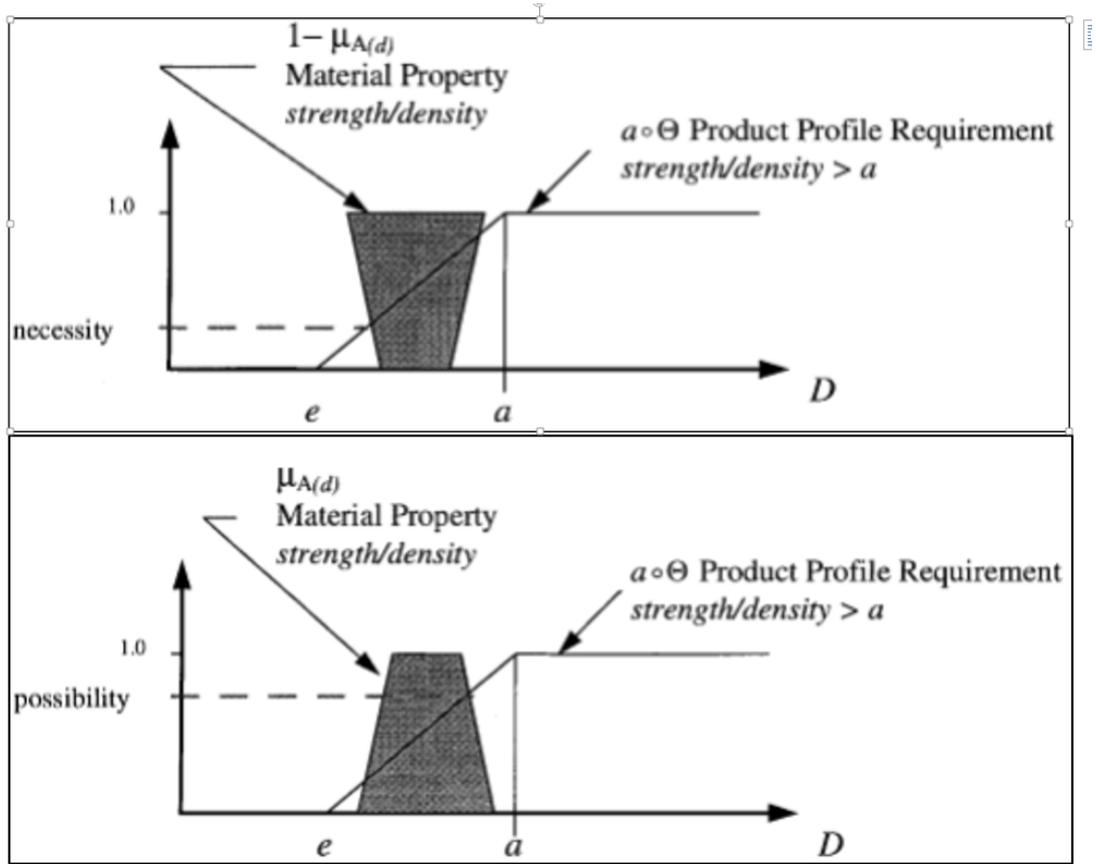
Figure 2.7: Possibility measure (left) and Necessity measure (right) under a variable requirement [Giachetti, 1998].
