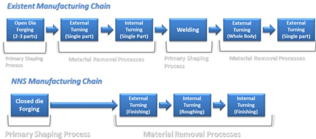
Figure 7.6: Comparison between existent (top) and NNS (bottom) manufacturing chains of the Case Study III.
