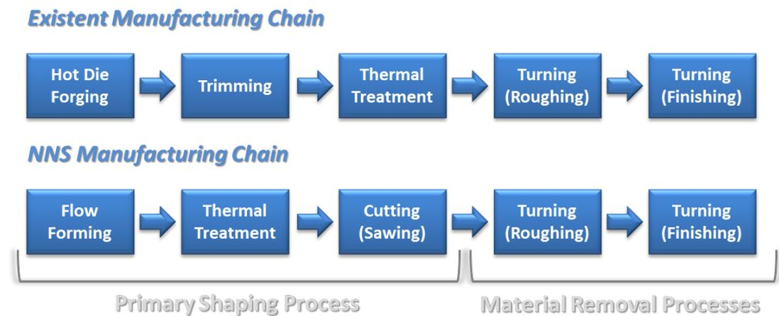
Figure 5.12: Comparison between existent (top) and NNS (bottom) manufacturing chains of Case Study IB.
