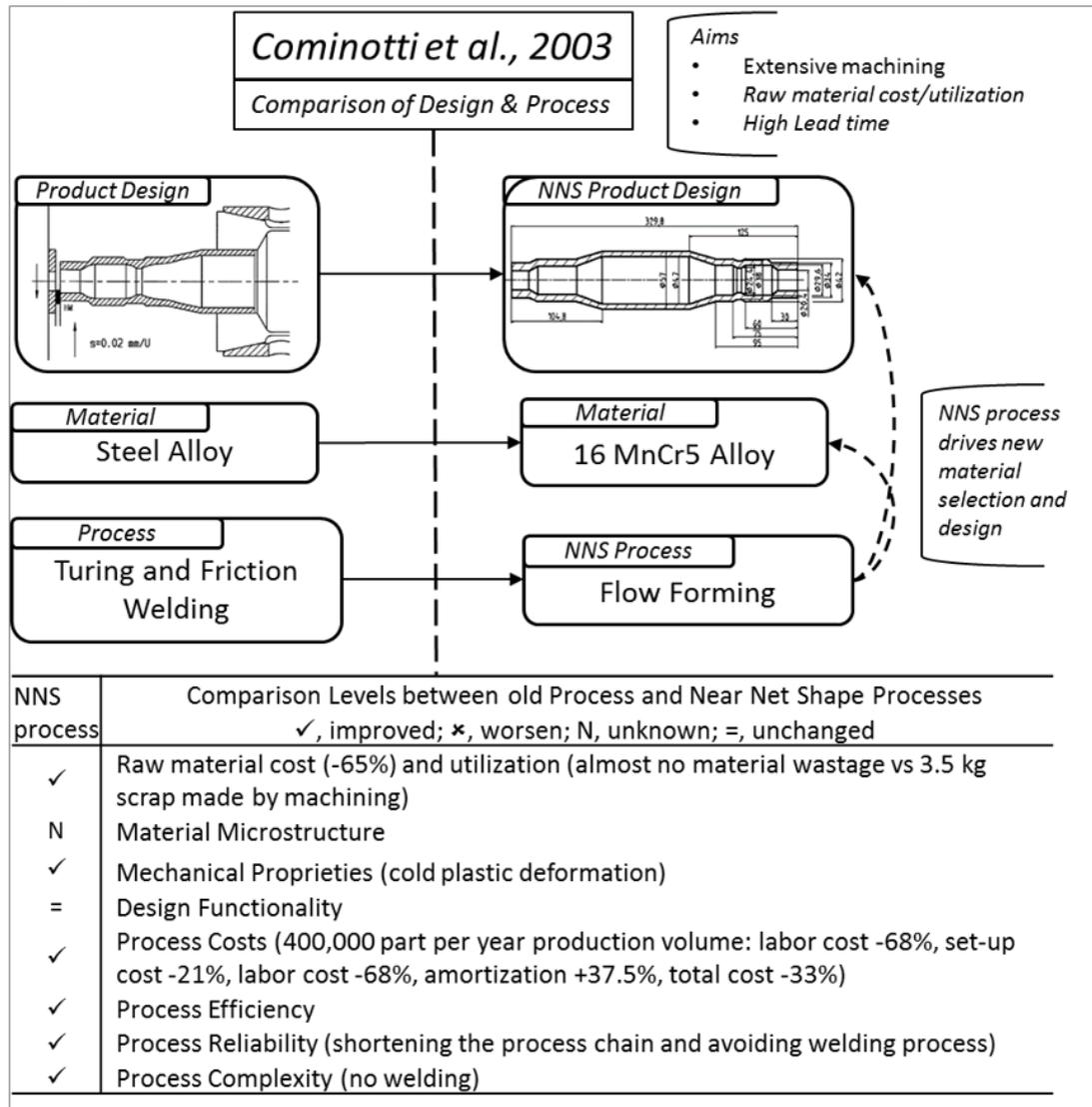
Figure A.9: Schematic representation of Cominotti and Gentili [2008] experimental paper (old process, material, product design and new NNS tested process, investigation motives and Targets, NNS variables developments and comparison levels).
