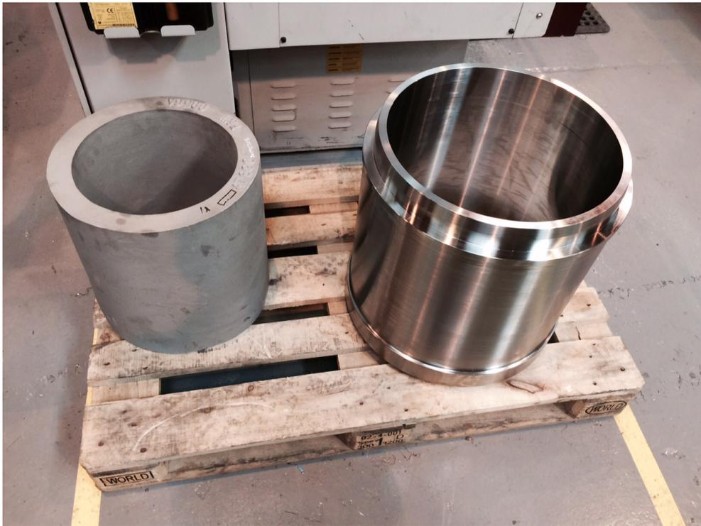
Figure 6.5: Centrifugal casting blank (left), semi-finished valve cage (right).
