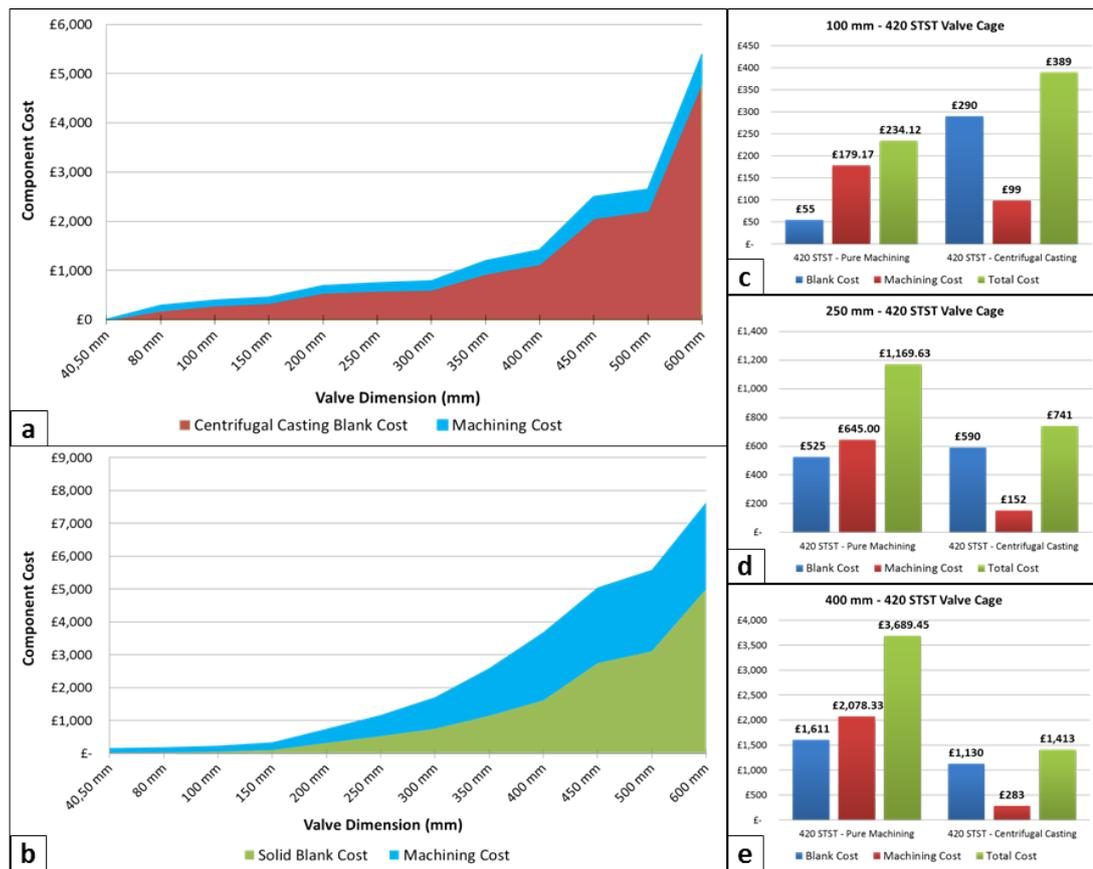
Figure 6.8: Cost comparison for the NNS process chain (a) and existing chain (b). Cost details for different cages sizes: 100 mm (c), 250 mm (d) and 400 mm (e). Component cost comparison of component evaluated costs for the NNS process chain (i.e. centrifugal casting and finish machining) and the existing process chain (i.e. machining from solid blank) (f).
