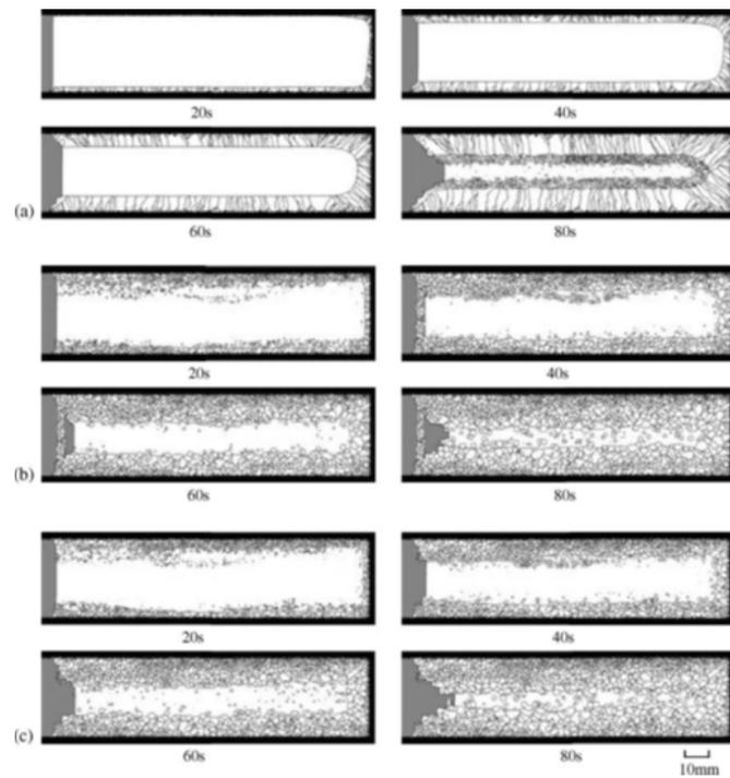
Figure D.5: Simulated microstructures of Ti-6Al-4V alloy at different solidification and mould rotation speeds in centrifugal casting: (a) 0 rpm, (b) 160 rpm, (c) 260 rpm [Ping et al., 2006]
