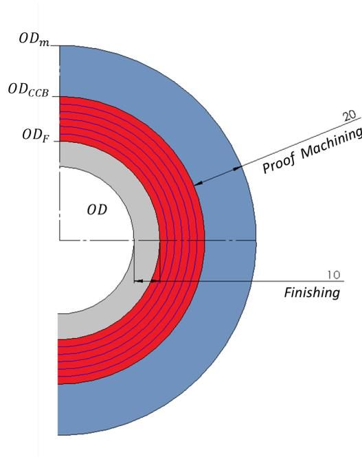
Table F.5: External turning process scheme and nomenclature scheme (blue: proof machining zone; red: roughing zone; grey: finishing zone)
