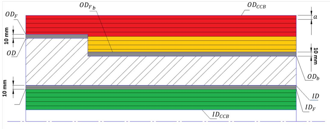
Figure 6.13: Turning strategy scheme and diameters: external turning zone (red); external bottom section turning (yellow), internal turning (green).
