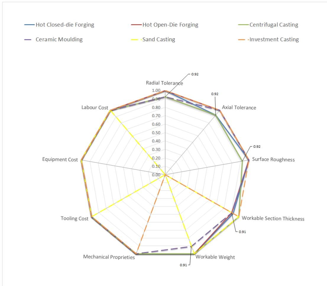
Figure 4.17: Process compatibilities breakdown for the Case Study III.
