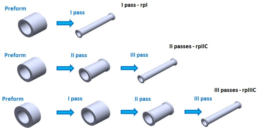
Figure 5.8: Examples of low forming processes for valve seat: rpIC (top), rpIIC (middle), rpIIC (bottom).
