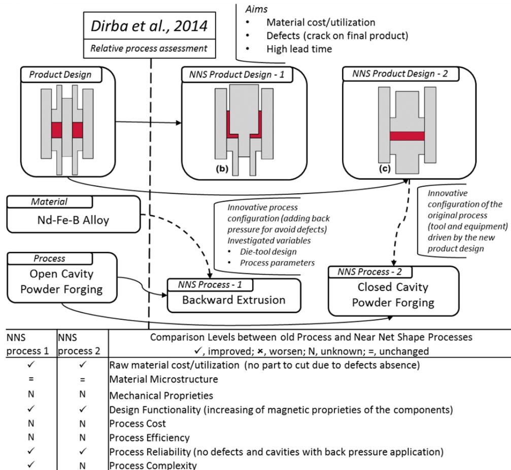
Figure A.6: Schematic representation of Dirba et al. [2014] experimental paper on magnet forging (old process, material, product design and new NNS tested processes and product designs; investigation motives and targets, NNS variables developments; comparison levels between old and NNS process).
