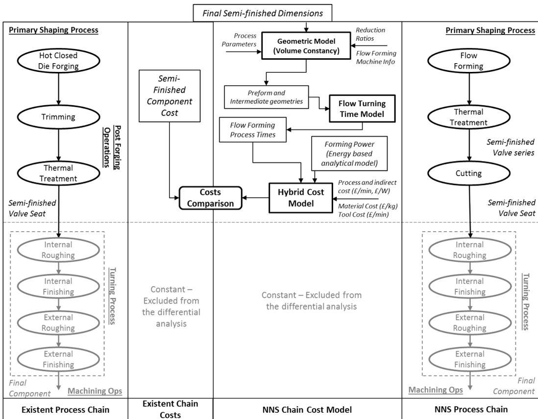
Figure 5.16: Differential cost analysis between the existent and NNS manufacturing processes of Case Study IA.
