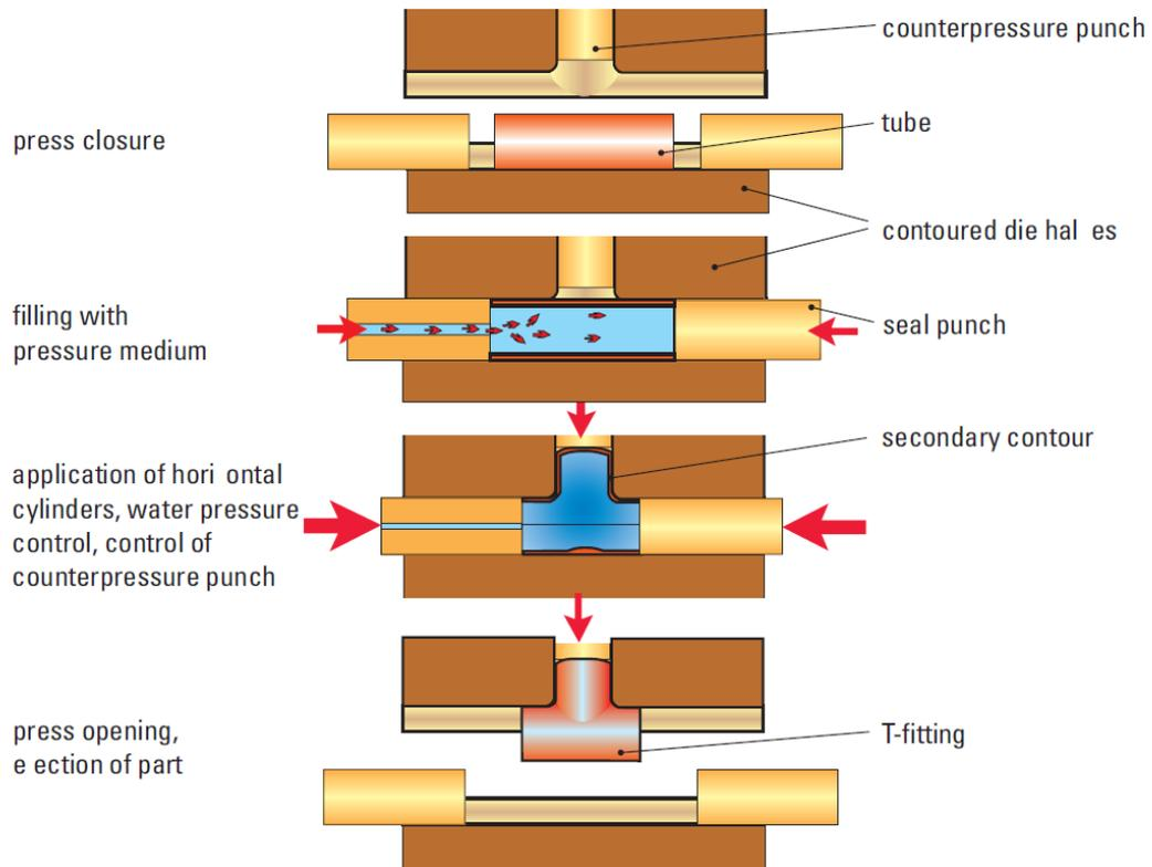
Figure B.3: Schematic of a Tube hydroforming process [Schuler, 1998].
