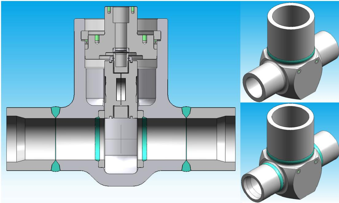
Figure 7.4: Different options for open die forging of a valve body: two piece (*left and right-top*) and four pieces (*right-bottom*).
