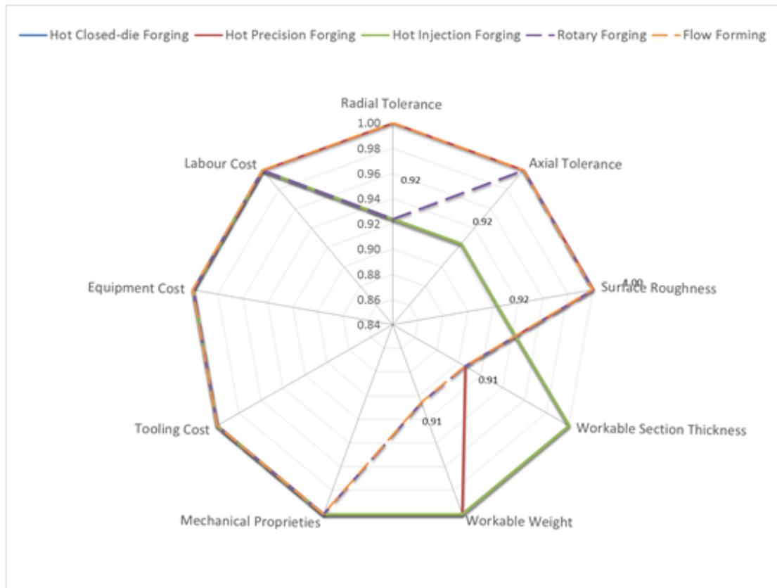
Figure 4.10: Process compatibilities breakdown for the Case Study IA (part I).
