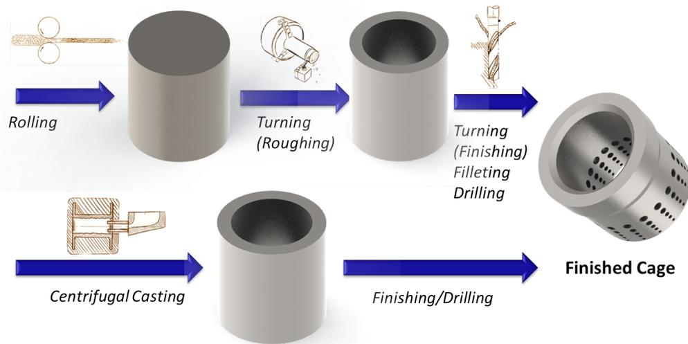
Figure 6.4: Schematic of the existing manufacturing process chain (top) and NNS manufacturing process chain (bottom).
