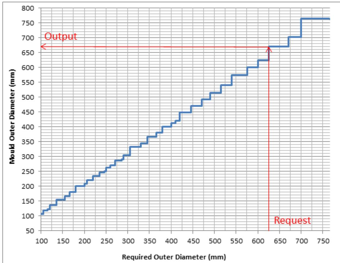
Figure F.1: Step diagram for selecting the centrifugal casting mould outer diameter from the required outer diameter.
