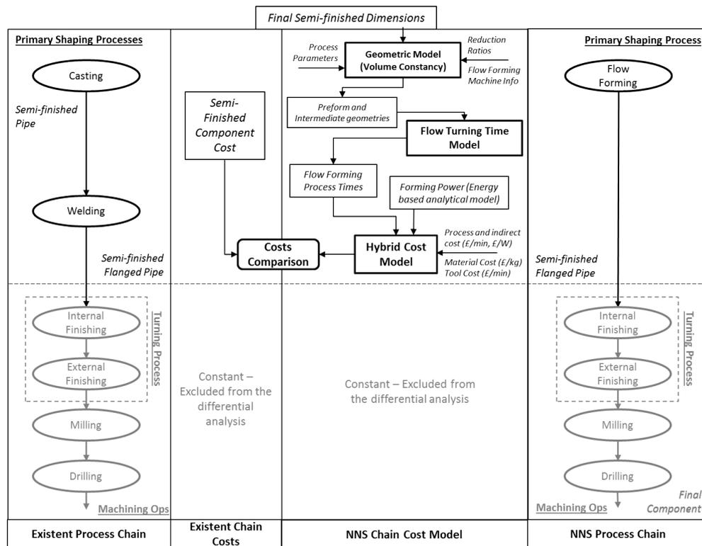
Figure 5.17: Differential cost analysis between the existent and NNS manufacturing processes of the Case Study IB.
