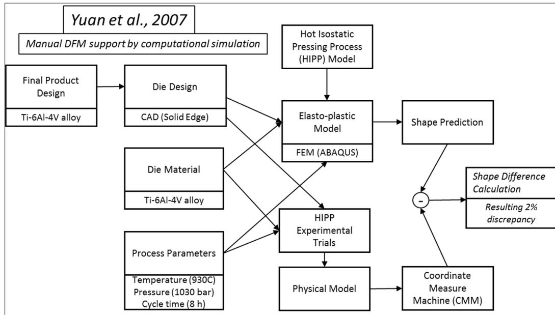
Figure A.3: Yuan et al. [2007] numerical investigation scheme for evaluating hot isostatic pressing final shape prediction through FEM.
