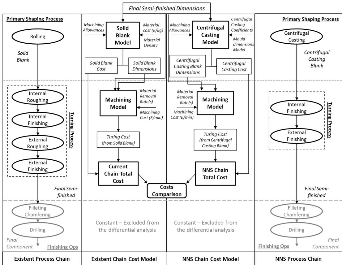
Figure 6.6: Differential cost analysis between the existent and NNS manufacturing processes of Case Study II.
