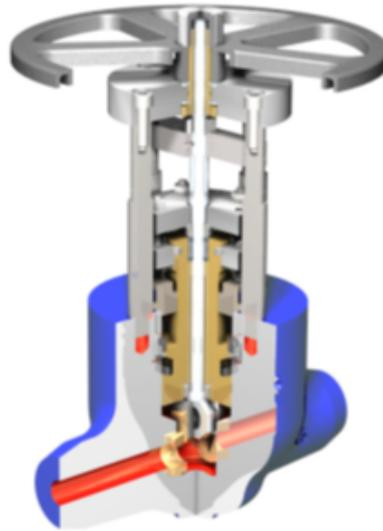
Figure 7.2: Parallel gate valve.
