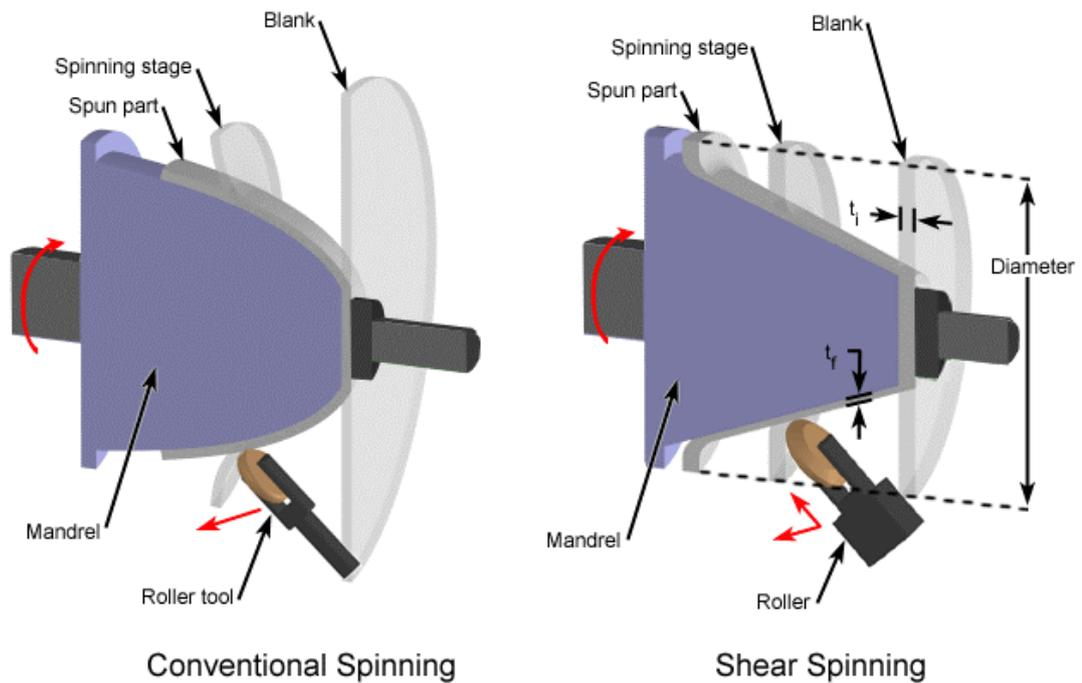
Figure B.2: Schematic of Conventional Spinning and Shear Forming processes [Sivanandini et al., 2012].
