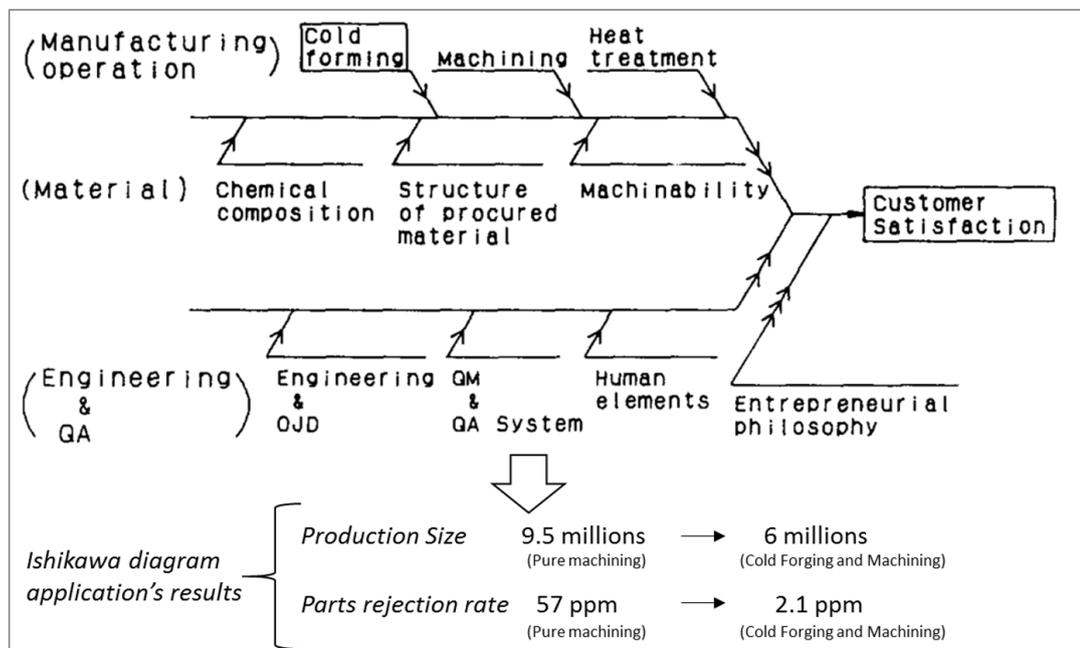
Figure A.8: Onodera and Sawai [1992]'s Ishikawa diagram for cold forging and results of its application
