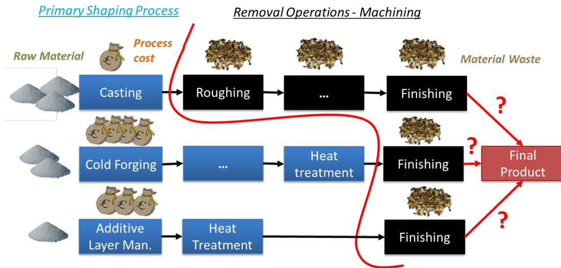
Figure 1.1: Primary shaping process change: impact on the manufacturing line.
