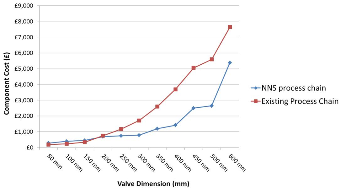
Figure 6.9: Component cost comparison of component evaluated costs for the NNS process chain (i.e. centrifugal casting and finishing machining) and the existing process chain (i.e. machining from solid blank).
