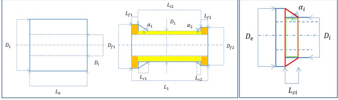
Figure E.2: Volume constancy modification for a flanged pipe.
