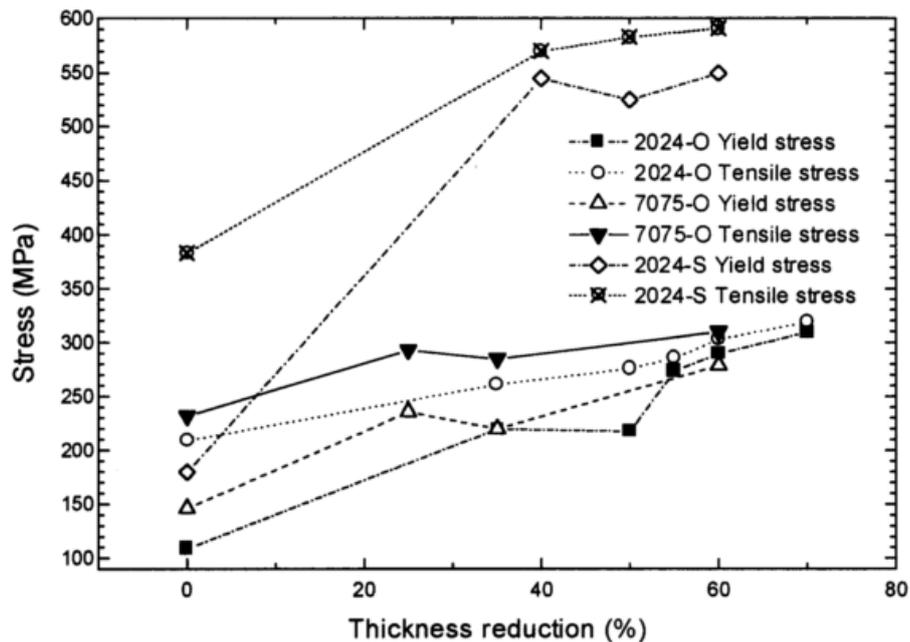
Figure D.1: Axial tensile properties of 7075-O, 2024-O and 2024 aluminium tubes for different reduction ratios [Chang et al., 1998].
