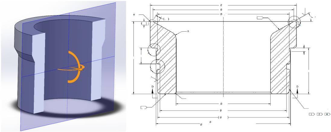
Figure 5.9: CAD representation of the valve seat (without finishing details).
