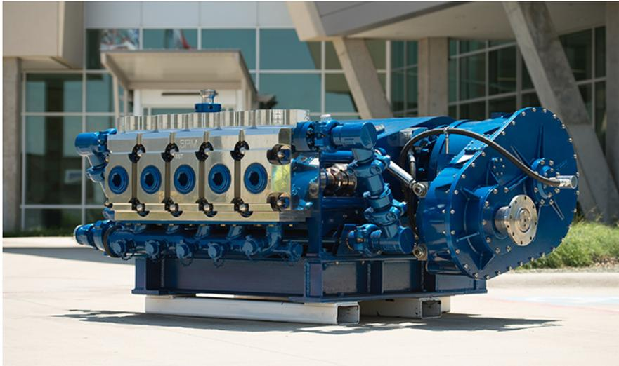
Figure 4.1: Fracking pump.
