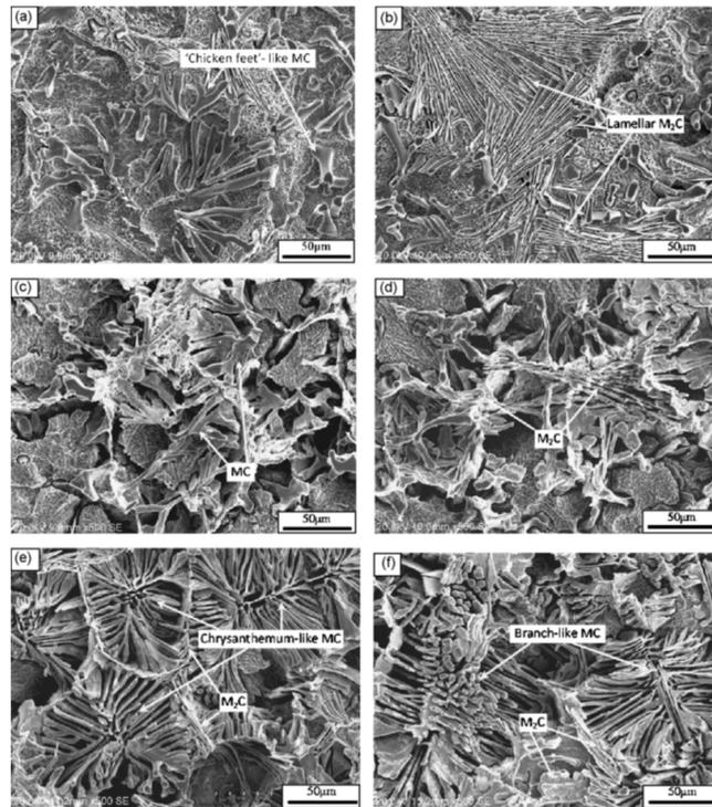
Figure D.7: SEM micrographs of the morphology of deep etched eutectic carbides [Luan et al., 2010]
