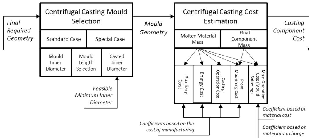
Figure 6.7: Schematic of the developed centrifugal casting cost model.
