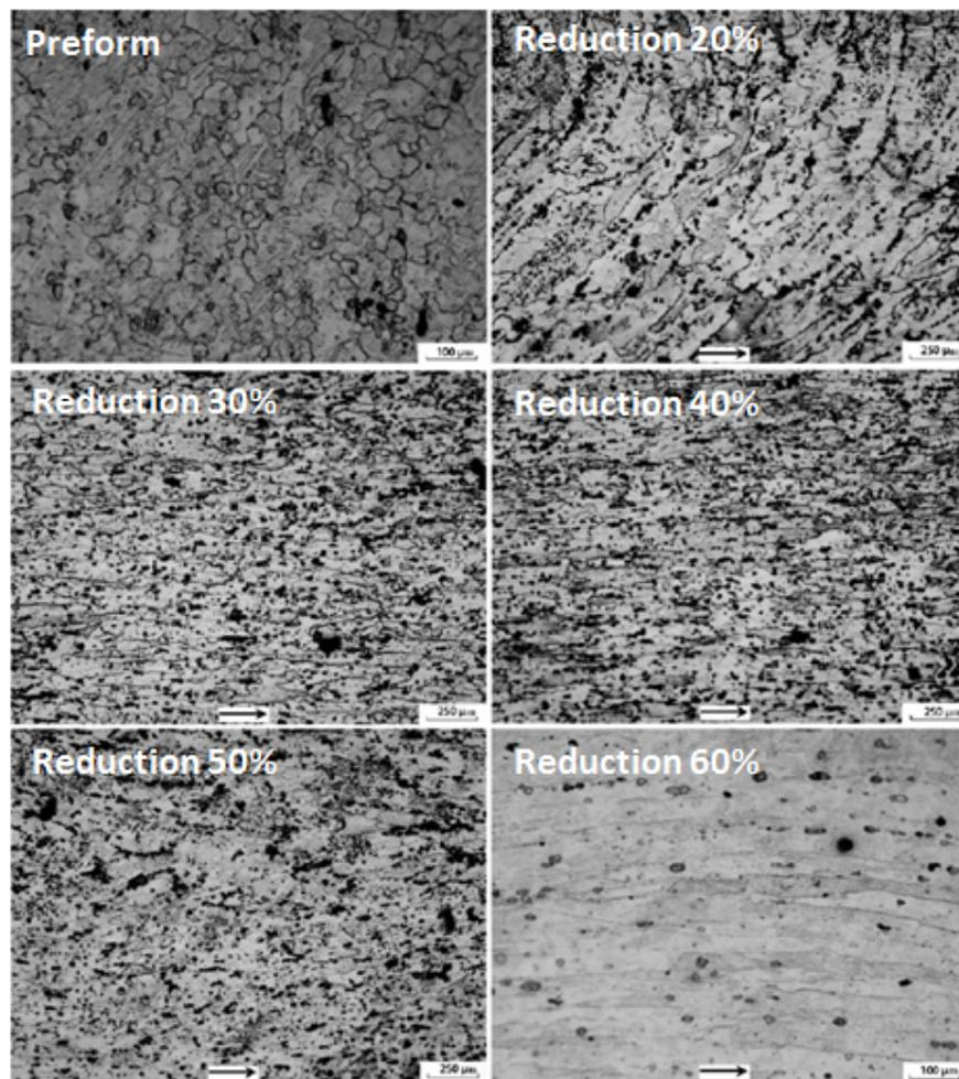
Figure D.2: Microstructure of full annealed 7075 aluminium alloy, 0.2 thickness reduction, 0.3 thickness reduction, 0.4 thickness reduction, 0.5 thickness reduction, 0.6 thickness reduction [Molladavoudi and Djavanroodi, 2010].
