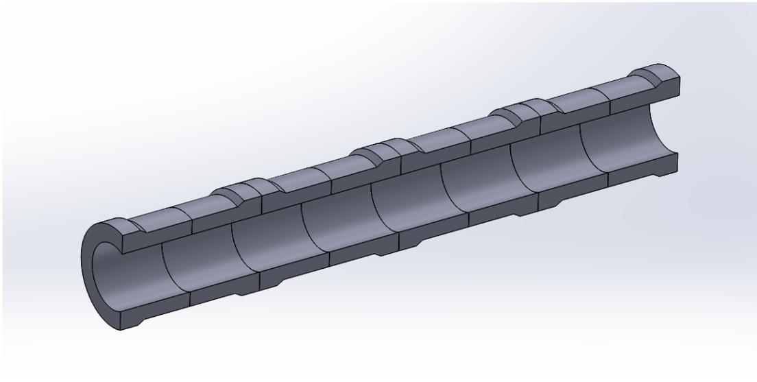
Figure 5.11: NNS design for stacked production (multiple valve seats configuration) using flow forming
