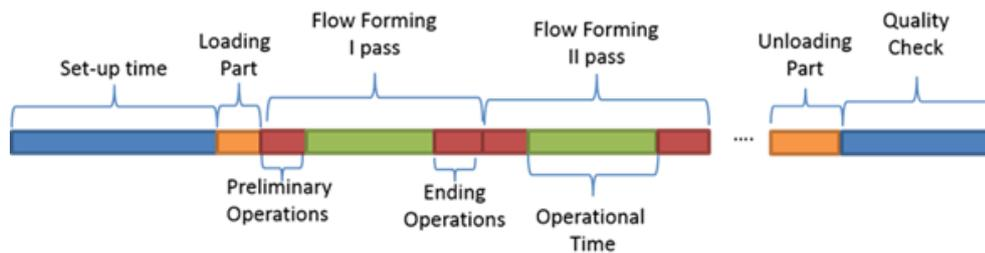
Figure 5.14: Flow forming time model schematization for hollow tube (up) and flanged pipe (down).
