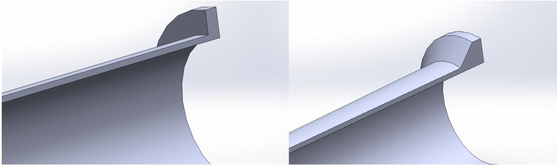
Figure 5.6: Difference between current design (welded flange) and NNS design (flow formed chamfer).
