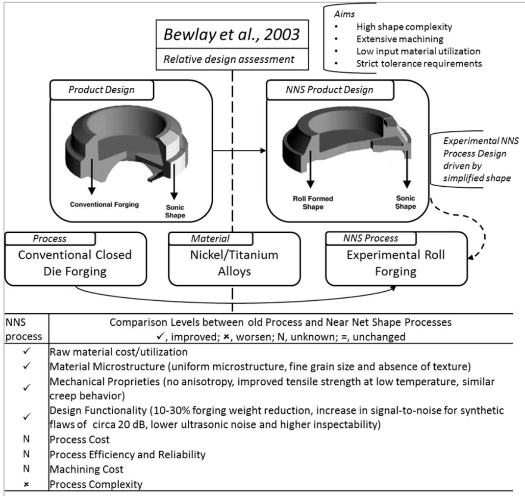
Figure A.7: Schematic representation of Bewlay et al. [2003] experimental paper on engine disk roll forging (old process, material, product design and new NNS tested process and product designs, investigation motives and Targets, NNS variables developments, comparison levels between old and NNS process).
