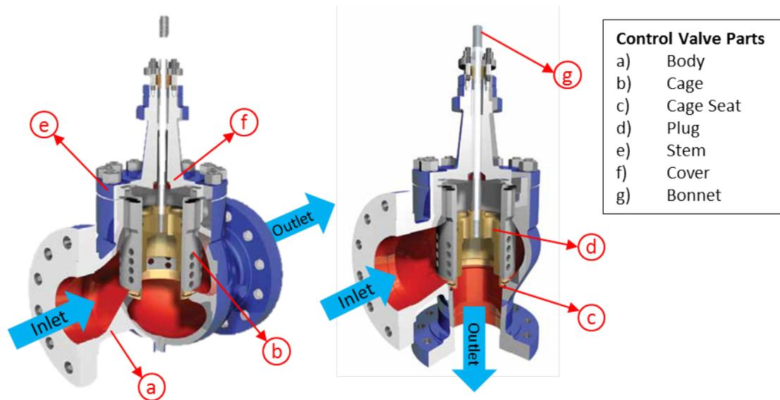
Figure 6.3: Control valve schematic showing the valve cage (Case Study II).
