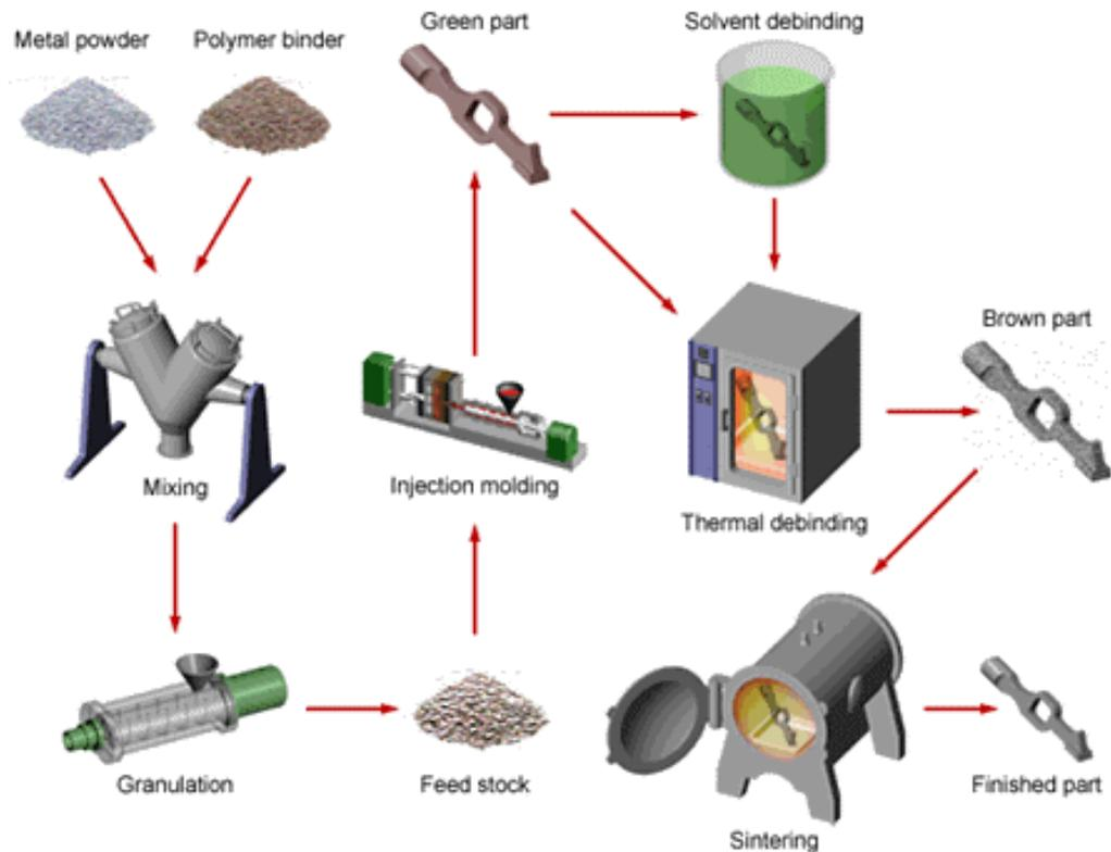
Figure B.4: Schematic of a Metal Injection Molding process [Swift and Booker, 2013].
