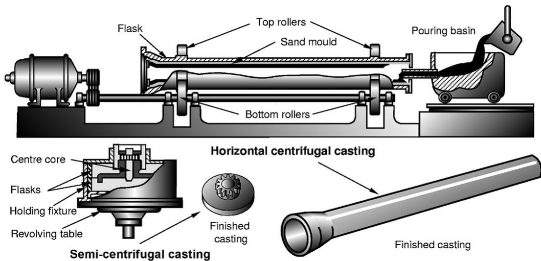
Figure B.1: Schematic of True Centrifugal Casting and Semi-Centrifugal Casting processes [Swift and Booker, 2013].
