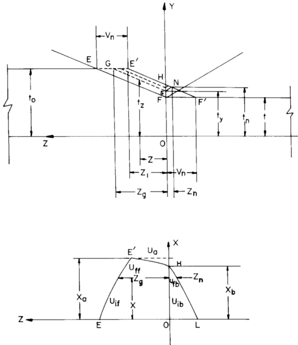
Figure E.3: Energy method, contact zone model for flow forming [Hayama and Kudo, 1979b]
