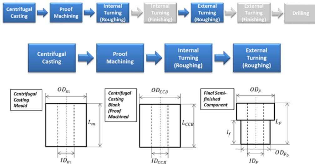
Figure 6.11: Valve cage manufacturing process chain model for optimization.
