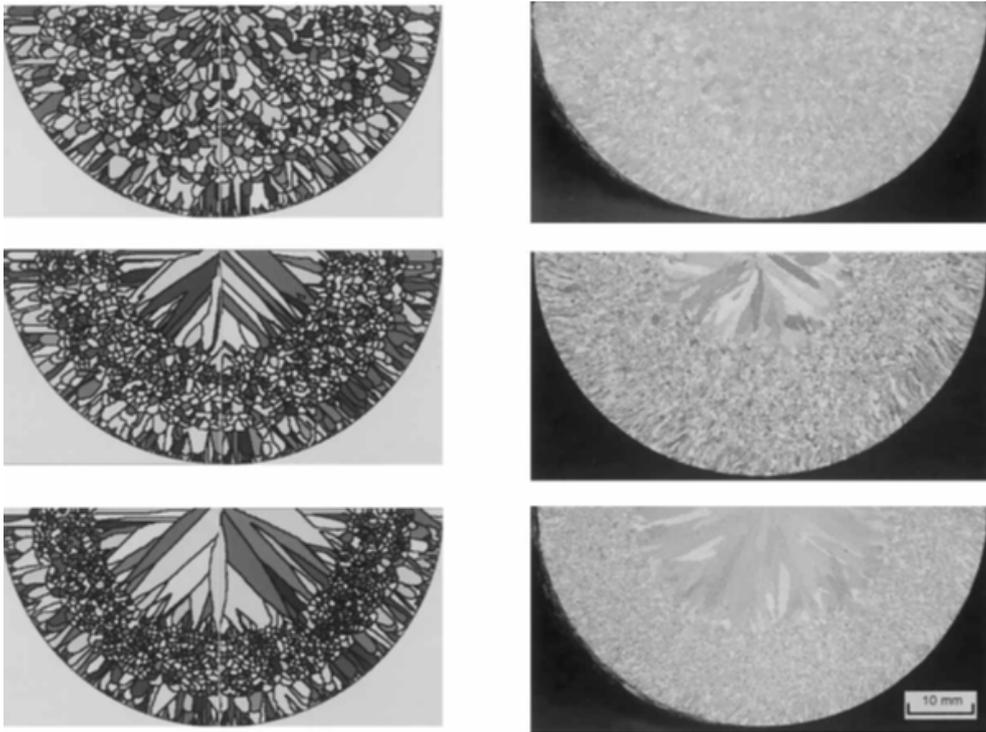
Figure D.4: Comparison of the simulated and experimental macrostructures of an AlSi alloy for various mould preheat temperatures: a) 10°C, b) 70°C, and c) 150°C [Chang et al., 2001]
