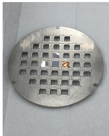
Figure 3.5: 37 position sample holder utilised for physical vapour deposition studies with the QBox 450 system.
