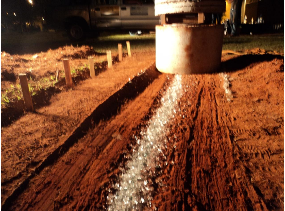
Figure 7.5: View of the cylinder after it has been dragged along the corridor and the trench filled with glass shards. It is evident that the glass shards are clean, free from soil particles and the soil corridor free from glass shards. This means that during the experiment minimal mixing between glass shards and soil took place. The glass shards visible on the sides of the cylinder (at the corridor borders) are glass shards from the trench that were above the ground level and were scrapped off from the front of the cylinder during its displacement.
