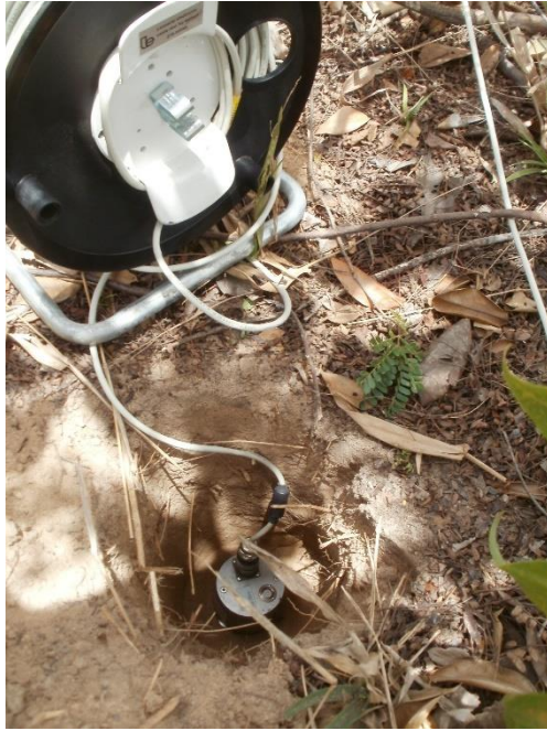
Figure 5.3: All seismometers were placed into ~50cm deep holes and were then covered with soil. This was done to increase their coupling with the surrounding soil and decrease the effect of ambient noise.
