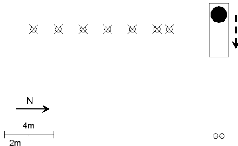
Figure 6.3: Plan view of experimental set up. Solid Black Circle; cylinder with confined soil block, Rectangle surrounding the cylinder; Surficial corridor free from vegetation, Circles marked with X; Location of seismometers, Two circles connected with a line; Position of reel. The dashed arrow shows the direction of the movement of the cylinder.
