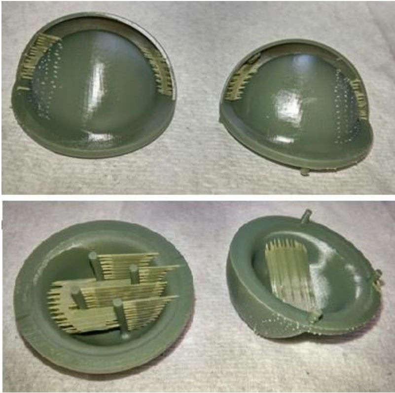
Figure 69: Photos of re-printed prototypes with vertical supports (iteration #3)
