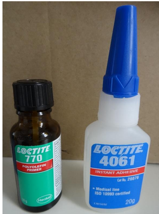
Epoxy glue and primer used to attach sparger pieces
