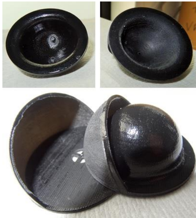
Figure 57: Photos of printed sparger pieces missing connecting post (iteration #1)
