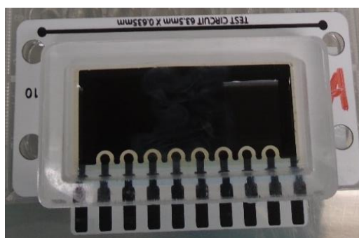
Figure 6.14. Image of a WBM chamber. Some central gel detachment is visible as lighter colouring.
