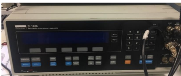
Figure 3.7. Image of the Solartron SI1260 impedance gain/phase analyser used for impedance measurements.
