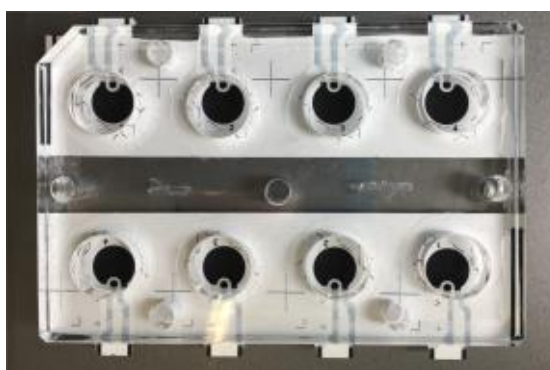
Figure 3.16. Carbon electrodes assembled into an array of 8 sensor wells.
