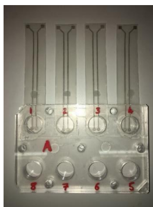
Figure 3.11. Ag/AgCl sensor plate assembly. Here 4 sensors have been secured between the acrylic plates, which have the potential to house up to 8 sensors.
