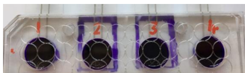
Figure 3.12. Image of crystal violet leakage from chamber after 24 hours (during sealant pattern testing).
