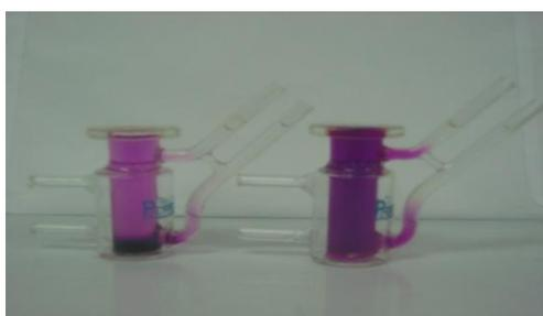
**Figure 8.2:** Effect of stirring factors on the mixing of  $\text{KMnO}_4$  dye in the receptor cell (left) no stirring and (right) stirring using stirrer bar (12.5 x 3.2 mm).
