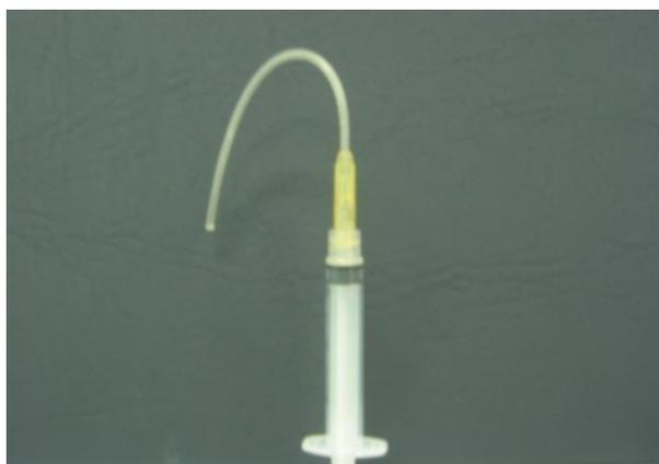
**Figure 8.1:** Plastic syringe with latex tubing used for sampling
