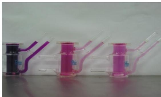
**Figure 8.4:** Effect of weight of the dye on the time required to distribute throughout the receptor cell including the two arms (left) 10mg– time taken 2.5 hours (centre) 5mg– time taken 30 minutes and (right) 1mg– time taken 22 minutes.
