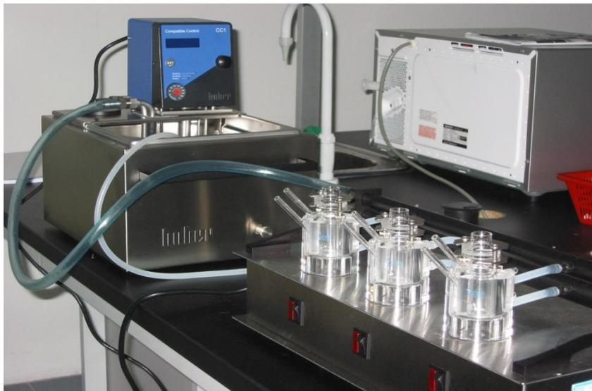
**Figure 2.17:** Franz cell experiment set up showing receiver, donor, stirring and heating glass blocks in addition to the circulating water bath.
