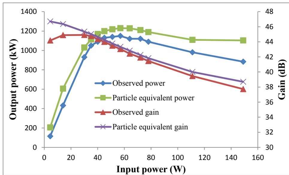
*Figure 5.5.2.5: Observed power/gain and particle equivalent power/gain as a function of input power for a gyro-TWA including a 14cm long helical down taper to an output mean radius and corrugation amplitude of  $\sim 0.80[r_0, l]$ , at 10.0GHz. The uniform helical waveguide section measured 56cm.*
