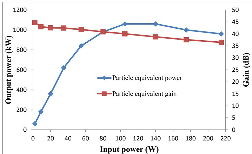
*Figure 4.3.6.2: Particle equivalent power and gain of the simulated gyro-TWA as a function of input power at 9.4GHz.*
