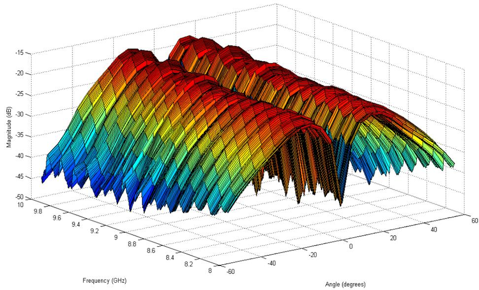
Figure 6.4.4: 3D plot of the azimuthal polarisation component with the mesh present, measured with an SNA over the entire optimised 2.0GHz frequency bandwidth of the converter.
