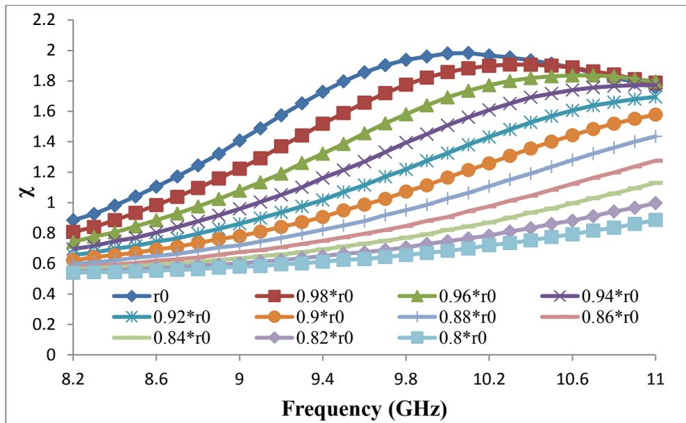
Figure 5.4.10: The content of the  $TE_{21}$  mode,  $\chi$ , in the operating eigenwave as a function of frequency for helical waveguides with varying mean radii and corrugation amplitudes.
