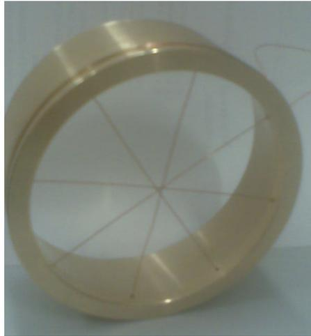
*Figure 6.4.1: Cathode mesh with eight spoke copper wire structure.*
