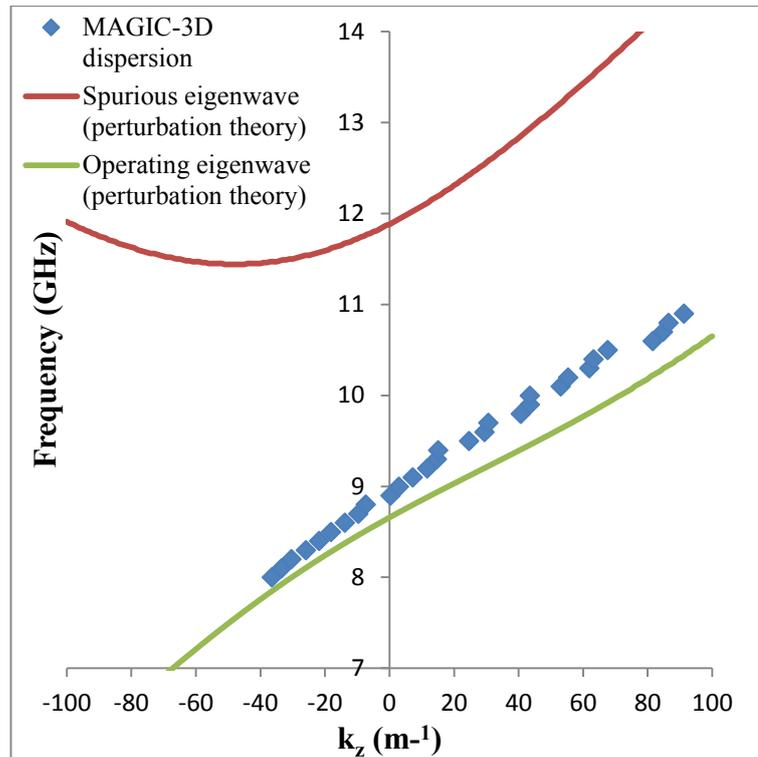
Figure 4.4.5: MAGIC-3D dispersion calculation of the helical waveguide minus contributions from the cylindrical to helical converters.
