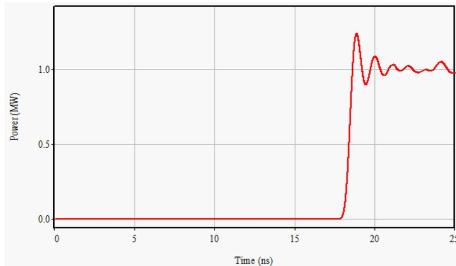
*Figure 4.3.3.1: An example of the observed power of a simulated gyro-TWA predicted by a Poynting flux diagnostic for an input power of  $\sim 105\text{W}$  at  $9.4\text{GHz}$ , taken from MAGIC-3D.*
