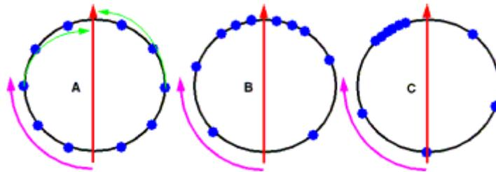
*Figure 2.5.1.1: Azimuthal electron phase bunch formation associated with the CRM instability.*
