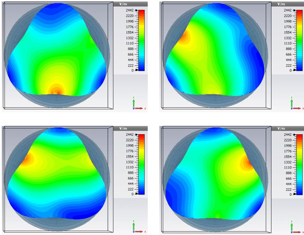
*Figure 5.4.4: Evolution of the electric field (phase angle  $0^\circ$ ,  $45^\circ$ ,  $90^\circ$ ,  $135^\circ$ ) for a drive frequency of 8.2GHz, taken from CST Microwave Studio. Here the field diagnostic was positioned midway along the length of the uniform helical waveguide section (see *figure 5.4.2*) and indicates a predominantly dipole ( $TE_{11}$ ) structure.*
