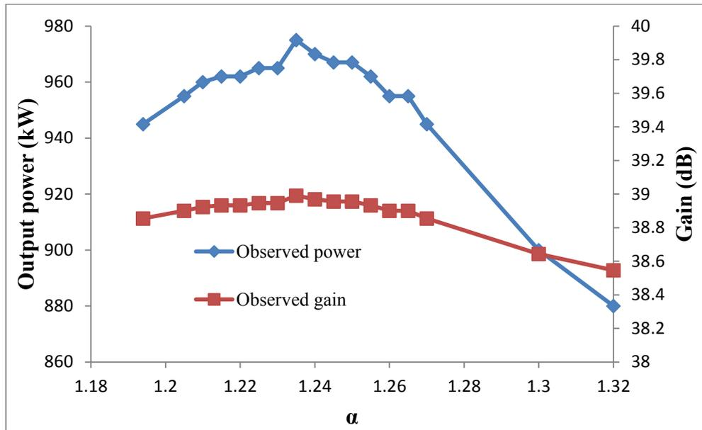
Figure 4.3.5.3: Observed power and gain of the simulated gyro-TWA for varying  $\alpha$ , with a magnetic field strength of  $\sim 0.2124\text{T}$  at  $9.4\text{GHz}$ .
