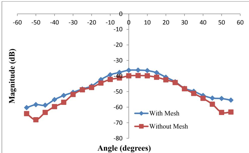
Figure 6.4.3: Comparison of the radial polarisation component of the electric field distribution at 9.0GHz centre frequency, with and without the plasma confinement mesh.
