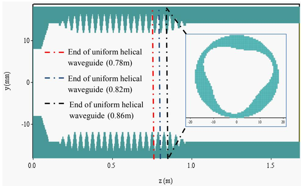
*Figure 5.2.2.4: Original simulation geometry as detailed in chapter 4 showing the original end to the uniform helical waveguide section at 0.86m and the new proposed end range of 0.78m to 0.82m to facilitate the start of the down taper, taken from MAGIC-3D.*
