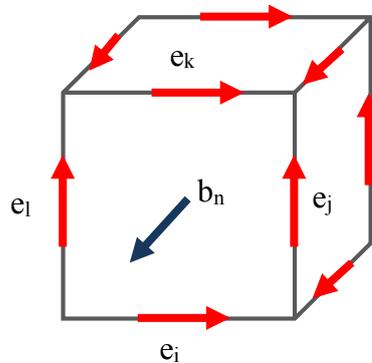
*Figure 3.3.1(b): Allocation of voltages along edges and fluxes through surfaces in the FIT.*
