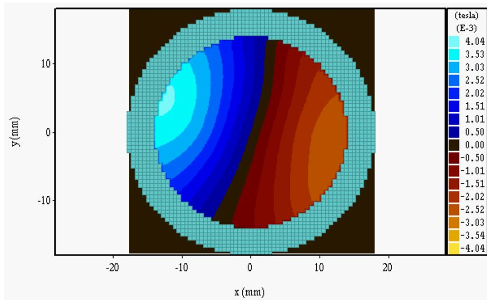
Figure 4.3.3.3: Contour plot in  $B_z$  showing the cylindrical  $TE_{11}$  mode at the output of the gyro-TWA, taken from MAGIC-3D.
