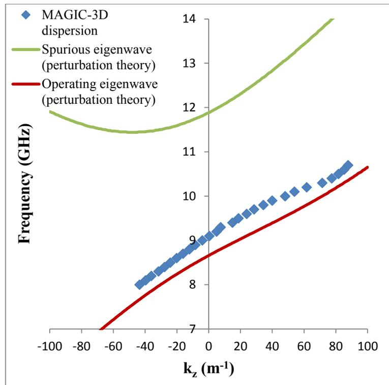
Figure 4.4.2: MAGIC-3D dispersion calculation for a 7.5cm section of helix plotted alongside the dispersion calculated from perturbation theory (cubic approximation).
