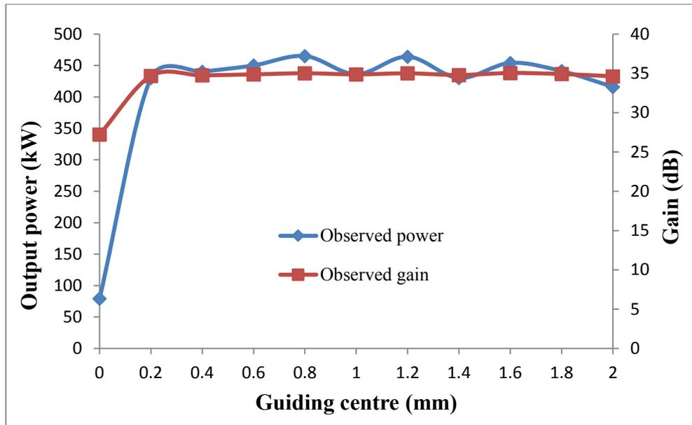
Figure 4.3.4.1: Observed power and saturated gain as a function of beam guiding centre radii for the simulated X-band 2<sup>nd</sup> harmonic gyro-TWA, operating with a magnetic field strength of 0.21T and an  $\alpha$  of 1.2 at 9.4GHz.
