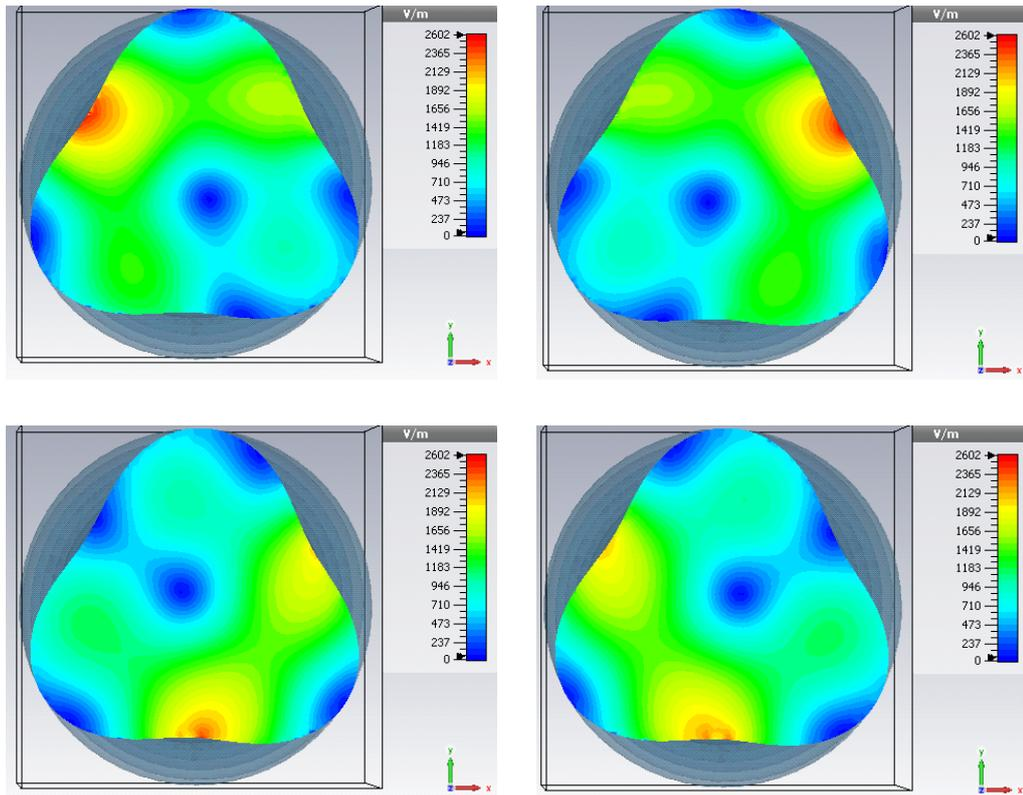
Figure 5.4.6: Evolution of the electric field (phase angle  $0^\circ$ ,  $45^\circ$ ,  $90^\circ$ ,  $135^\circ$ ) for a drive frequency of 10.8GHz, taken from CST Microwave Studio. Here the field diagnostic was positioned midway along the length of the uniform helical waveguide section (see figure 5.4.2) and indicates a predominantly quadrupole ( $TE_{21}$ ) structure.
