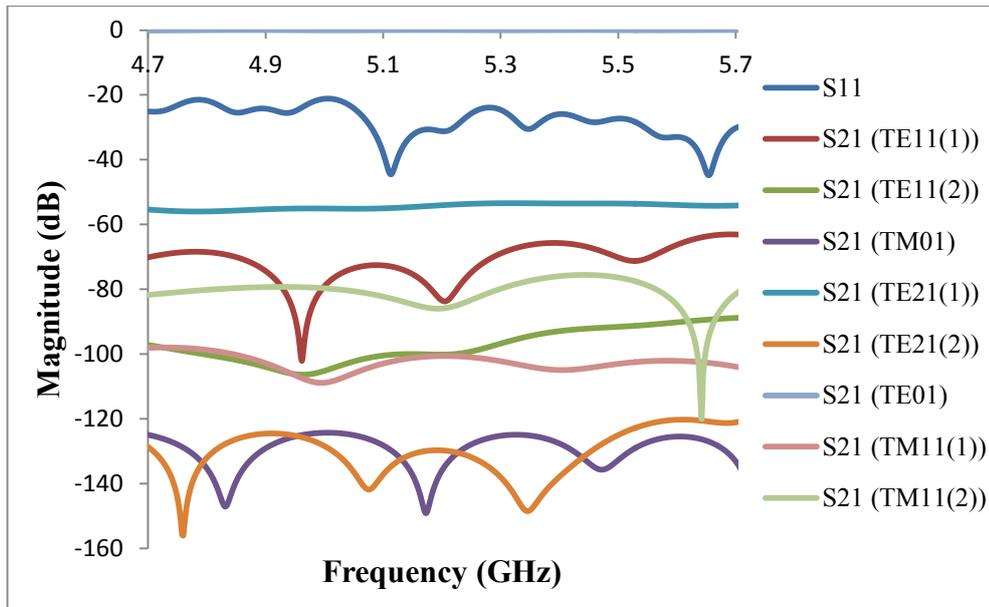
Figure 6.2.8: S-parameter plot for the 5.2GHz Marie-type converter.
