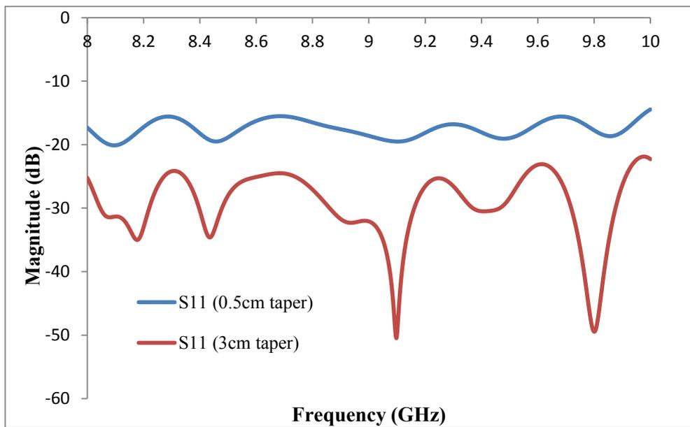
*Figure 6.2.2: S-parameter plots for the 9.0GHz Marie-type converter with a 0.5cm taper and a 3cm taper transition between the output of section 1 and the input of section 2.*
