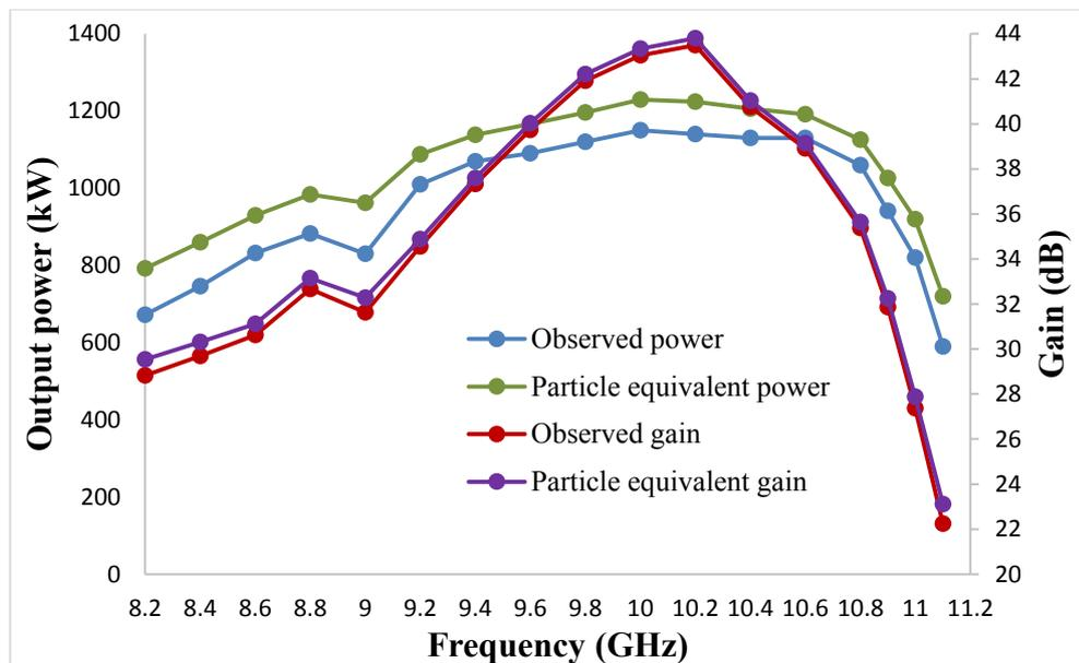
*Figure 5.6.2: Observed power/gain and particle equivalent power/gain as a function of frequency (with optimised input power) for the gyro-TWA which included a 14cm long helical down taper to an output mean radius and corrugation amplitude of  $\sim 0.80[r_0, l]$  positioned towards the output of the interaction region of the device. In all simulations the uniform helical waveguide section measured 56cm.*
