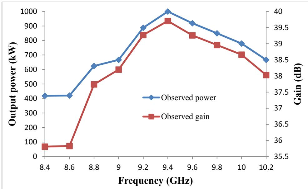
Figure 4.3.5.7: Observed power and gain of the gyro-TWA as a function of frequency for input powers of  $\sim 105W$  to  $\sim 110W$  with a magnetic field strength of  $\sim 0.2123T$  and an  $\alpha \sim 1.27$ .
