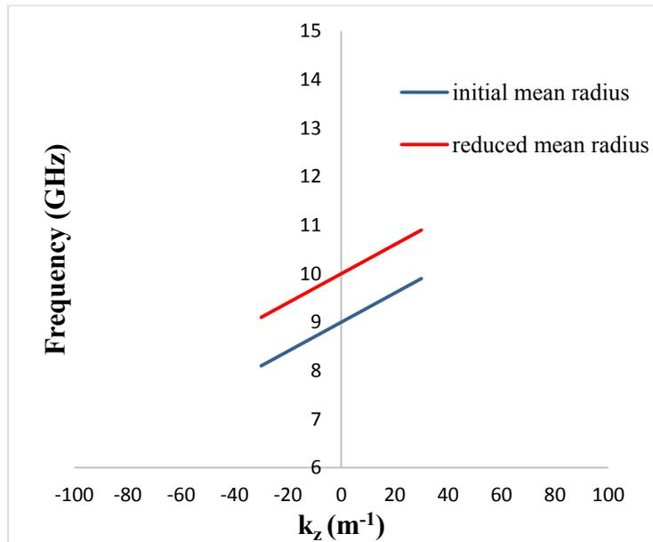
*Figure 2.5.7.2: Idealised dispersion of the operating eigenwave in a helically corrugated waveguide of different mean radii.*
