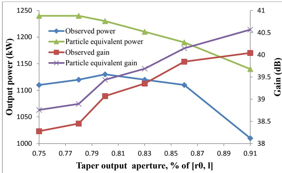
Figure 5.5.2.1: Observed output power/gain and particle equivalent power/gain as a function of output circuit aperture and input power at 10.0GHz. In each instance the gyro-TWA included a 10cm long helical taper and had a uniform helical waveguide measuring 52cm.
