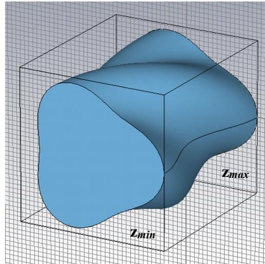
*Figure 4.4.6: A one period section (37.5mm) of helical waveguide used in the gyro-TWA dispersion simulations, taken from CST Microwave Studio.*
