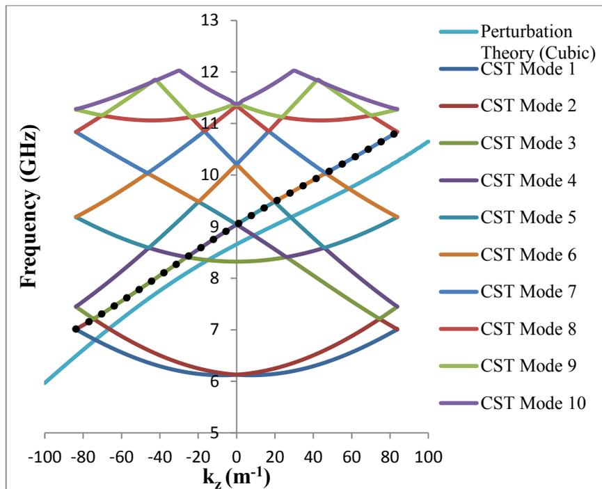
Figure 4.4.7: Dispersion calculation from CST Microwave Studio with the dotted line indicating the operating eigenwave.
