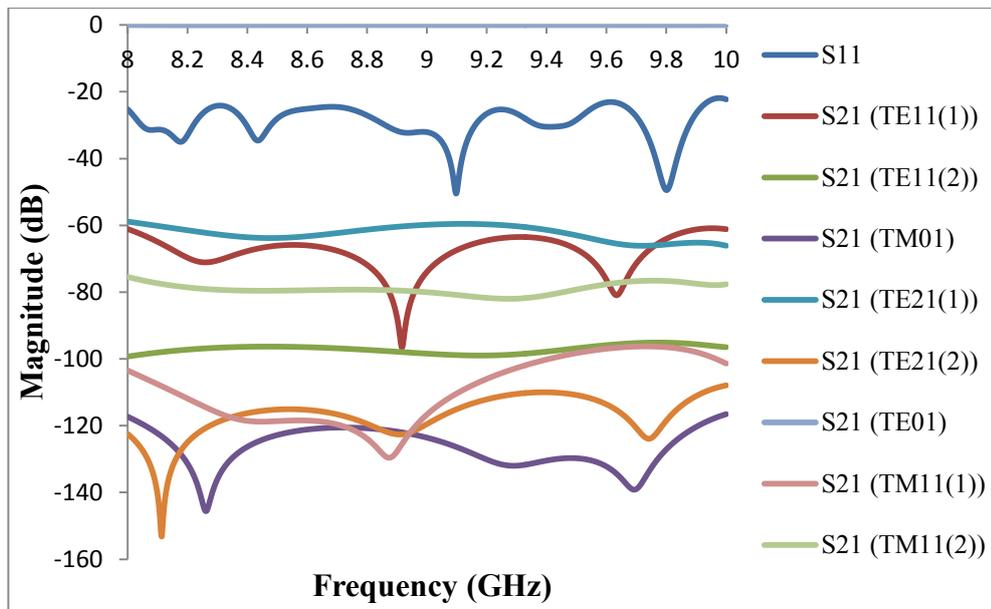
Figure 6.2.7: *S*-parameter plot for the 9.0GHz Marie-type converter.
