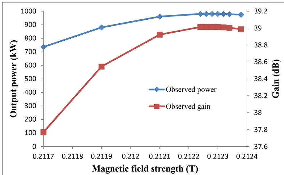
Figure 4.3.5.4: Observed power and gain of the simulated gyro-TWA for varying magnetic field strengths, with an  $\alpha$  of  $\sim 1.24$  at 9.4GHz.
