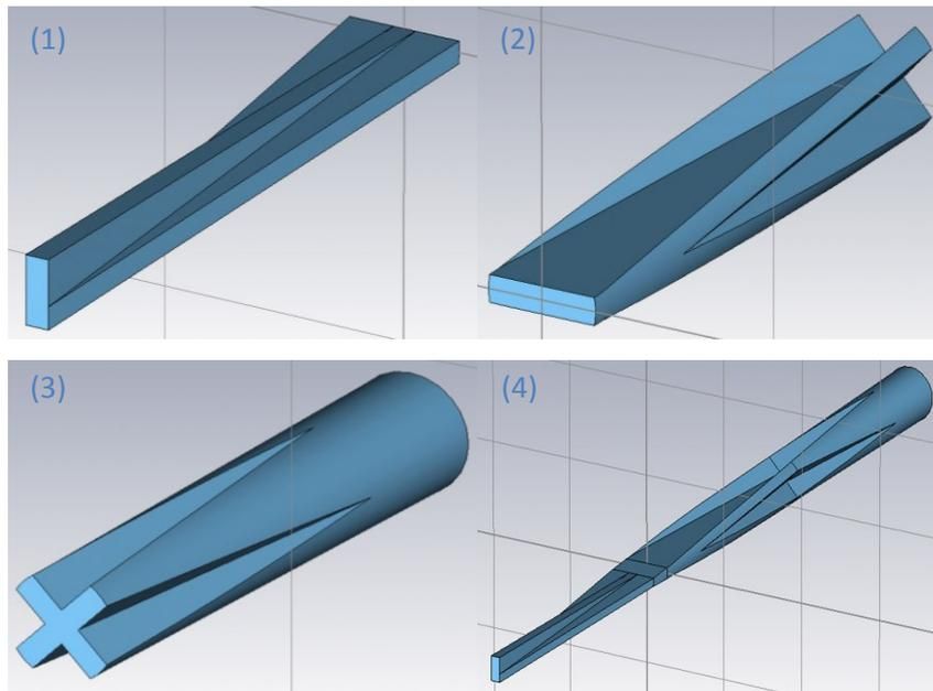
*Figure 6.2.1: The three main sections ((1), (2) and (3)) and the full 3D representation (4) of the Marie-type converter which includes a 3cm taper between the output of section 1 and the input of section 2, taken from CST Microwave Studio.*
