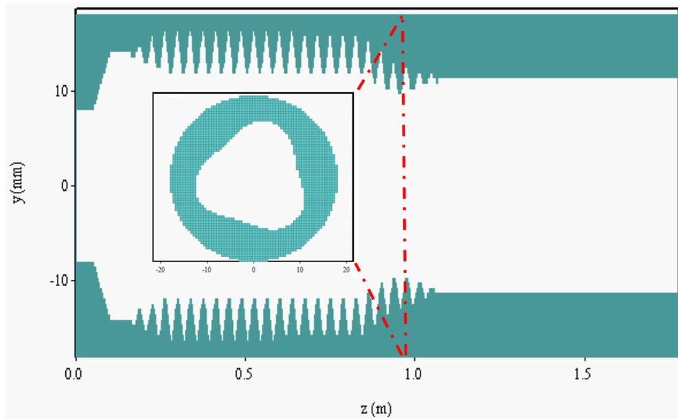
*Figure 5.2.2.5: An example of a proposed simulation geometry taken from MAGIC-3D. Here the gyro-TWA geometry includes a 14cm long helical down taper starting at an axial position of 0.82m. The output mean radius and corrugation amplitude of the taper have been reduced by ~20% from initial values of 14.1mm and 2.2mm respectively. In this instance the uniform helical waveguide section measures 56cm in length.*
