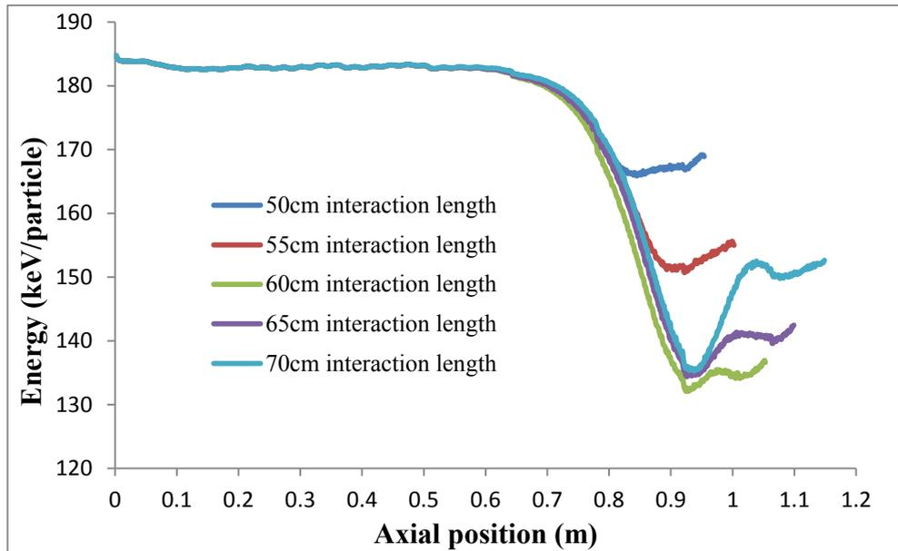
*Figure 4.3.7.2: Predicted average kinetic energy of the beam electrons as a function of axial position taken at 9.4GHz, for varying lengths of helical interaction waveguide.*
