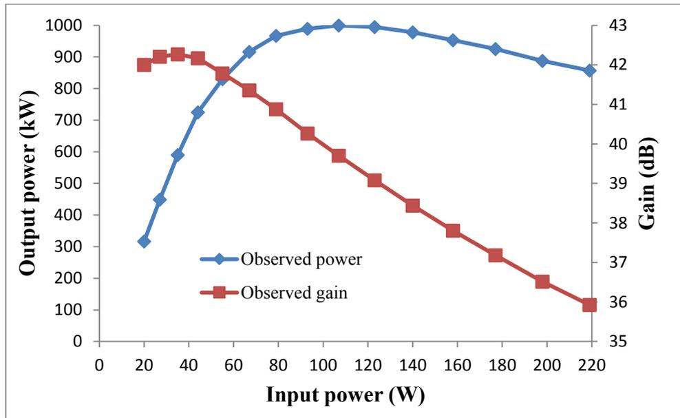
Figure 4.3.5.6: Transfer curve for the simulated gyro-TWA with a magnetic field strength  $\sim 0.2123T$  and an  $\alpha$  of  $\sim 1.27$  at 9.4GHz.
