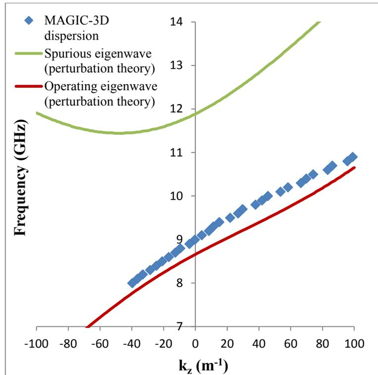
Figure 4.4.4: MAGIC-3D dispersion calculation for a 30cm long section of helix plotted alongside the dispersion calculated from perturbation theory (cubic approximation).
