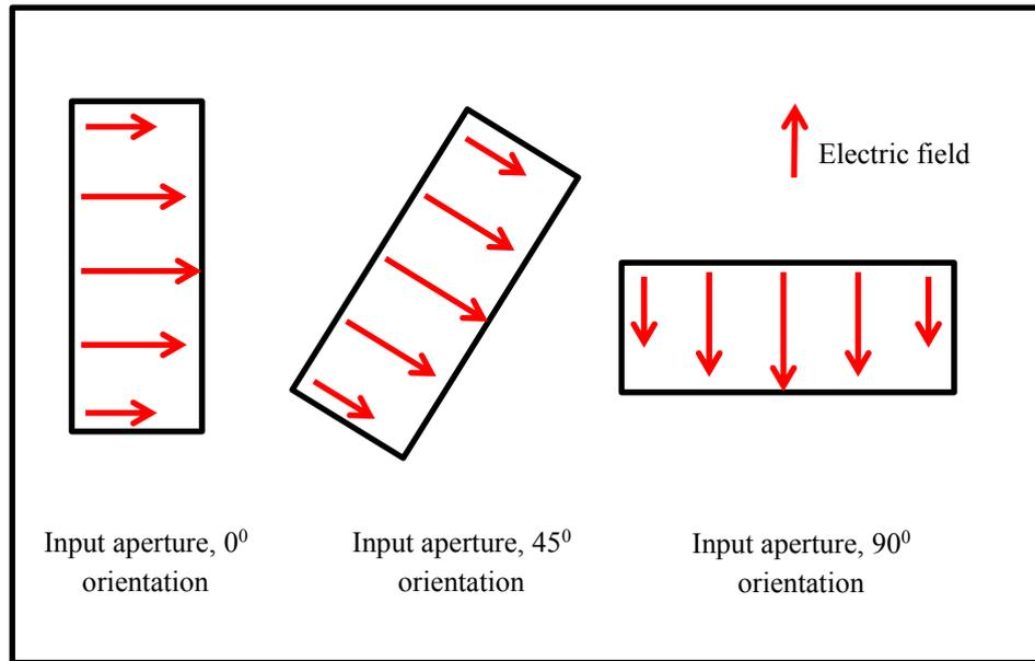
Figure 3.5.3: Orientation of the rectangular waveguide input of the Marie-type converter.
