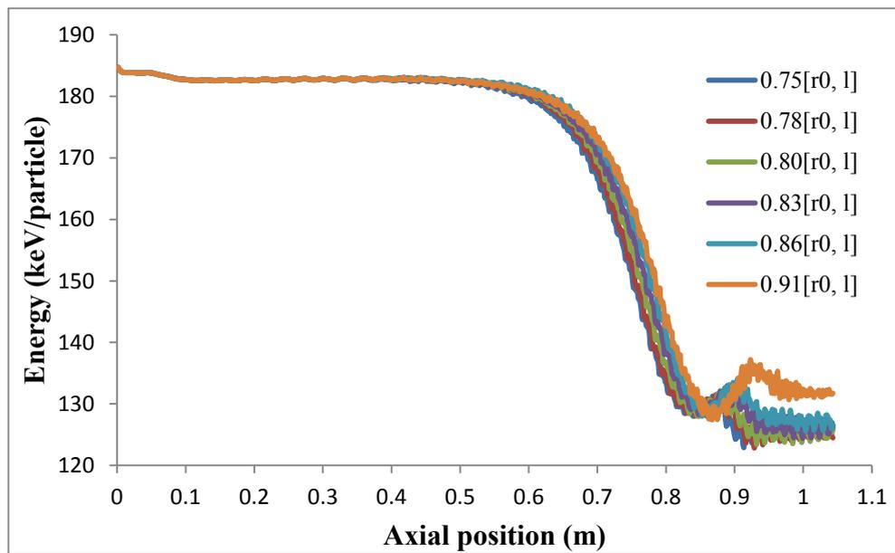
*Figure 5.5.2.2: Predicted average kinetic energy of the beam electrons as a function of axial position for gyro-TWAs including 10cm long helical tapers with output mean radii and corrugation amplitudes of  $\sim 75\%$  to  $\sim 91\%$  of the original values (i.e. from an initial  $r_0$  of 14.1mm and  $l$  of 2.2mm). In all instances the uniform helical waveguide measured 52cm with the amplifier operating at 10.0GHz.*
