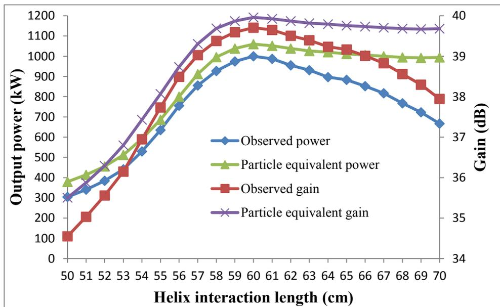
*Figure 4.3.7.1: Observed power/gain and particle equivalent power/gain of the simulated gyro-TWA as a function of interaction length, at 9.4GHz for an input drive power of ~105W.*
