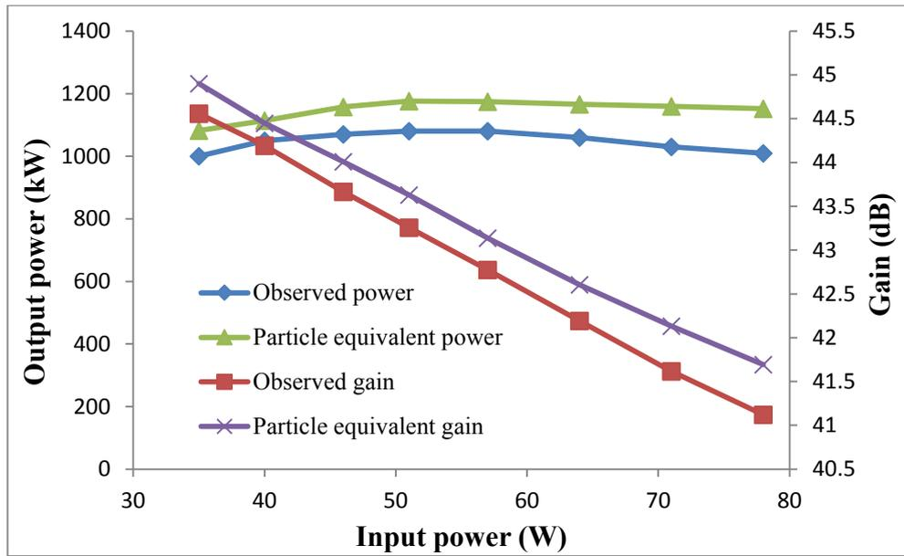
Figure 5.7.2: Observed power/gain and particle equivalent power/gain as a function of input power for a gyro-TWA including a 26cm long tapered helical to cylindrical converter with an output radius of  $\sim 0.80 \cdot r_0$ , at 10.0GHz. Here the uniform helical waveguide section of the amplifier measured 56cm.
