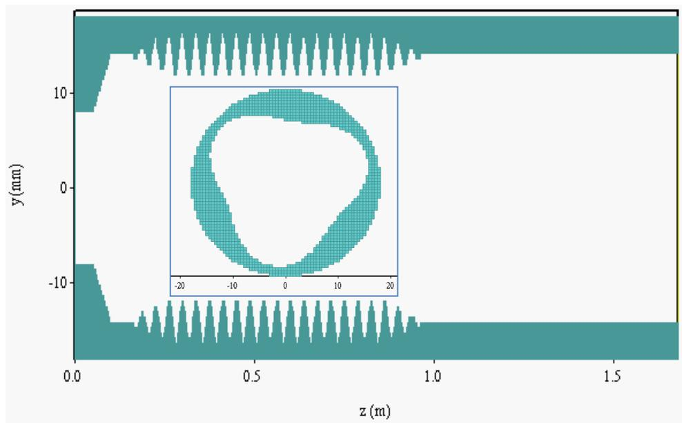
*Figure 4.3.1.1: Simulation geometry taken from MAGIC-3D of the X-band 2<sup>nd</sup> harmonic gyro-TWA, programmed using the Cartesian co-ordinate system.*
