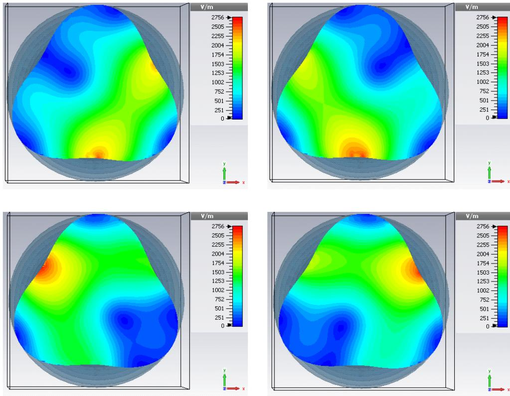
*Figure 5.4.5: Evolution of the electric field (phase angle  $0^\circ$ ,  $45^\circ$ ,  $90^\circ$ ,  $135^\circ$ ) for a drive frequency of 9.4GHz, taken from CST Microwave Studio. Here the field diagnostic was positioned midway along the length of the uniform helical waveguide section (see figure 5.4.2) and indicates a predominantly dipole ( $TE_{11}$ ) structure.*
