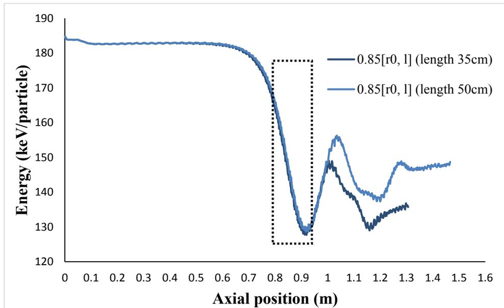
*Figure 5.5.1.3: Predicted average kinetic energy of the beam electrons as a function of axial position for gyro-TWAs including helical tapers of lengths 35cm and 50cm with output mean radii and corrugation amplitudes of  $\sim 0.85[r_0, l]$ , at  $10.0\text{GHz}$ . In both instances the length of the uniform helical waveguide section measured  $52\text{cm}$ .*
