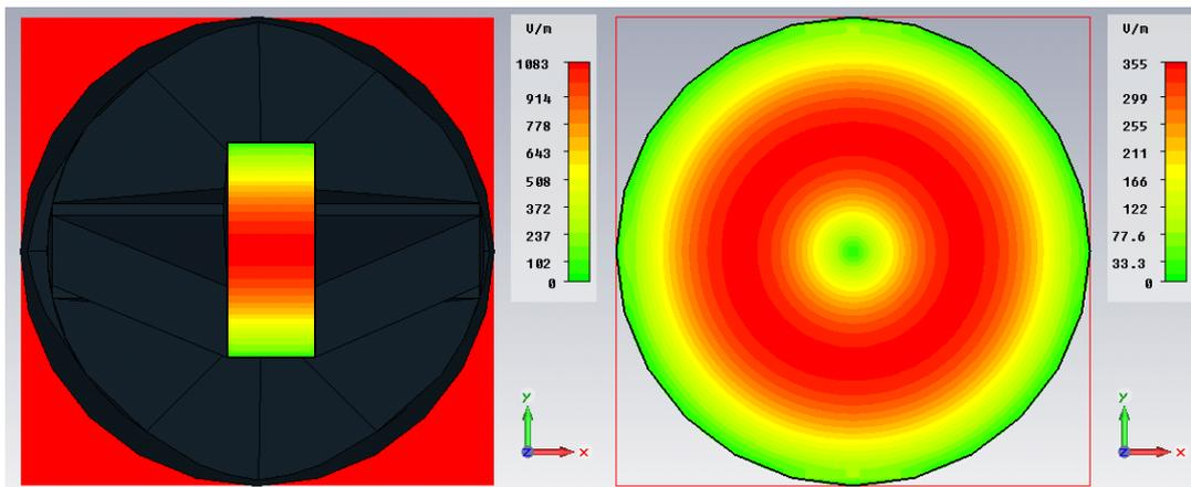
*Figure 6.2.5: Contour electric field distribution patterns (modes) at the input and output of the 5.2GHz Marie-type converter respectively, taken from CST Microwave Studio.*
