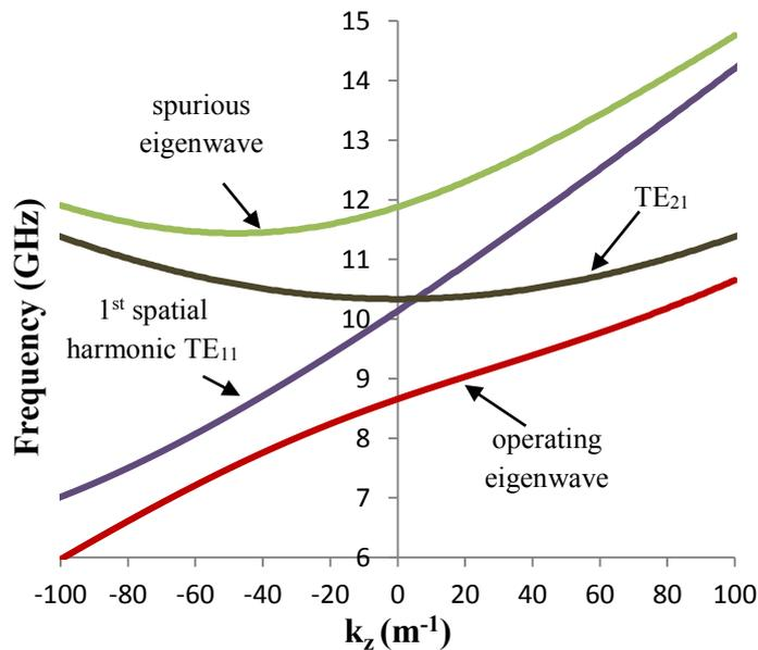
Figure 1.3.3: Dispersion diagram for a 3-fold helically corrugated waveguide.
