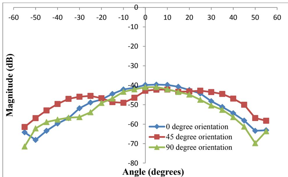
Figure 6.3.5: Radial polarisation component of the electric field distribution at the centre frequency of 9.0GHz, with the Marie-type converter at 0°, 45° and 90° orientations.
