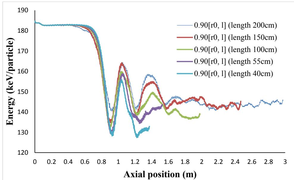
Figure 5.5.1.2: Predicted average kinetic energy of the beam electrons as a function of axial position for gyro-TWA geometries including helical tapers of lengths between 40cm and 200cm, with output mean radii and corrugation amplitudes of  $\sim 0.90[r_0, l]$ , at 10.0GHz. In all instances the length of the uniform helical waveguide section measured 52cm.
