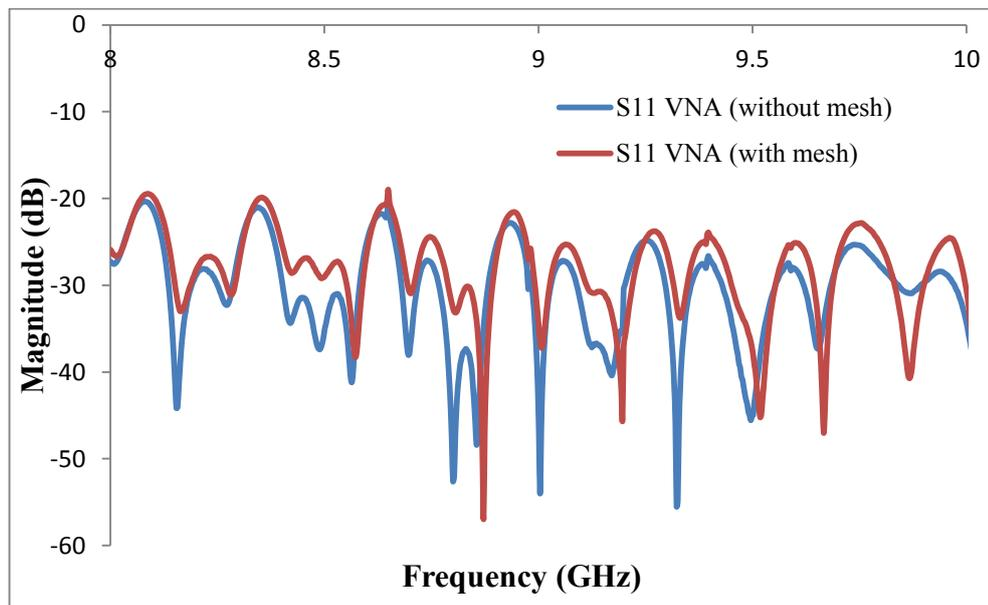
*Figure 6.4.6: Forward reflection coefficient (S<sub>11</sub>) with the presence of the 8 spoke cathode mesh compared to the same measurement taken when the mesh was not present, measured using a VNA.*
