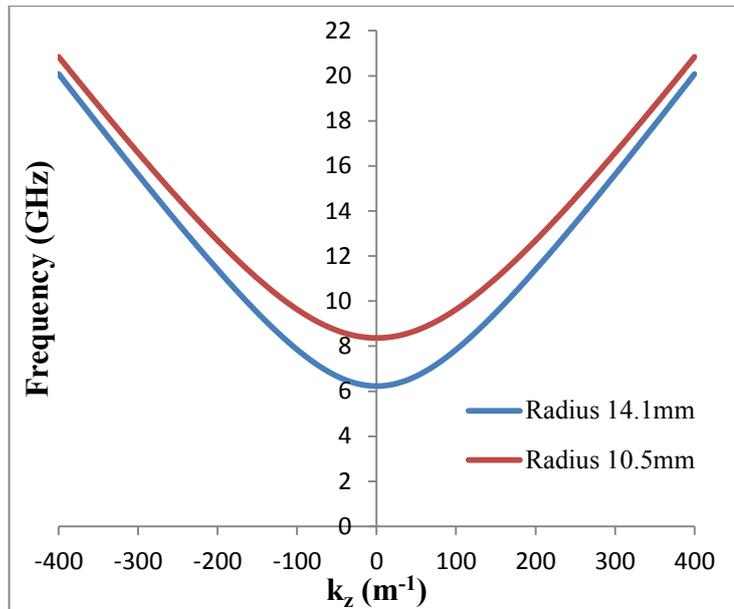
Figure 2.5.7.1: Cylindrical waveguide dispersion of the  $TE_{11}$  mode for two waveguide radii.
