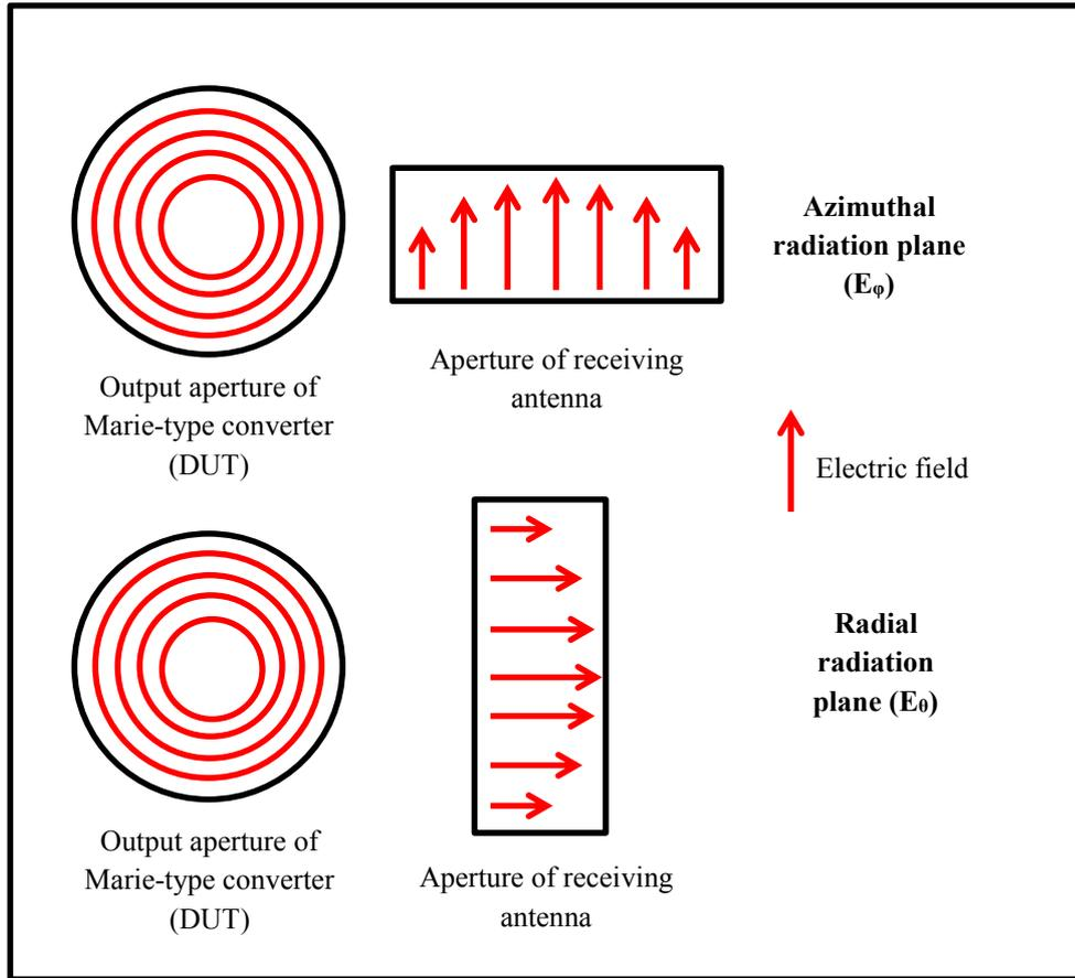
Figure 3.5.2: Orientation of the receiving antenna with respect to the output aperture of the Marie-type converter.
