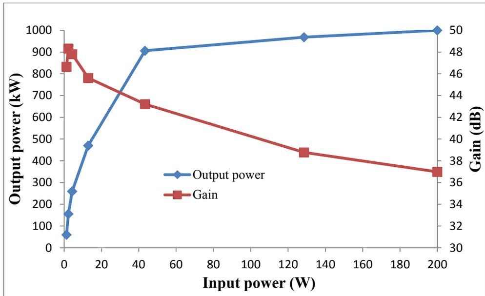
Figure 4.2.2.1: Measured output power and gain for given input powers of the experimental X-band 2<sup>nd</sup> harmonic gyro-TWA at 9.2GHz [Bratman, 2000].
