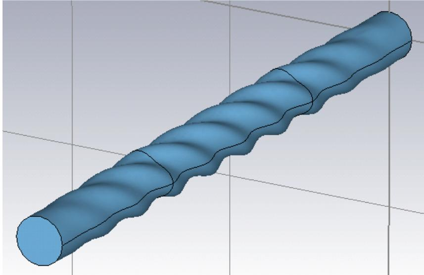
*Figure 5.4.1: 3D representation of a section of helical waveguide with a mean radius and corrugation amplitude of  $r_0$  and  $l$  respectively bracketed by two cylindrical to helical converters, taken from CST Microwave Studio. The cylindrical to helical converter has a constant mean radius of  $r_0$  and a corrugation amplitude which varies from 0 to  $l$  along the transition length. The helical to cylindrical converter is the inverse of the cylindrical to helical converter.*
