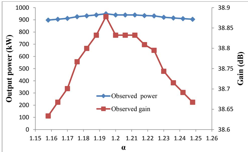
Figure 4.3.5.2: Observed power and gain of the simulated gyro-TWA for varying  $\alpha$ , with a magnetic field strength of  $\sim 0.2126\text{T}$  at  $9.4\text{GHz}$ .
