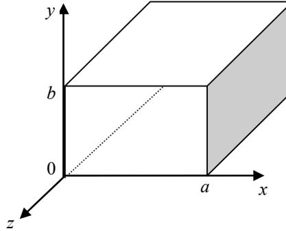
*Figure 2.3.3.1: Rectangular waveguide geometry.*
