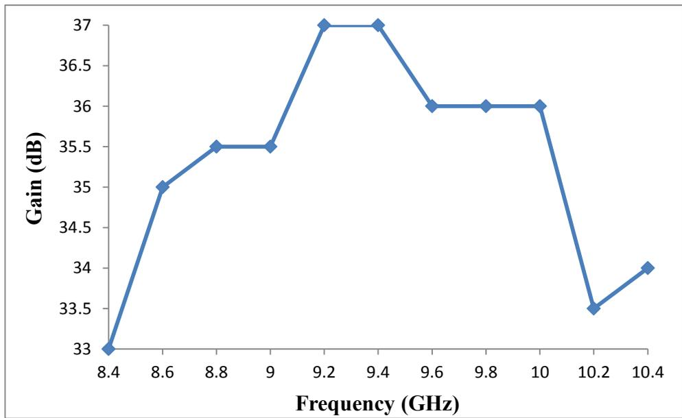
Figure 4.2.2.2: Measured saturated gain as a function of frequency for the experimental X-band 2<sup>nd</sup> harmonic gyro-TWA [Bratman, 2000].
