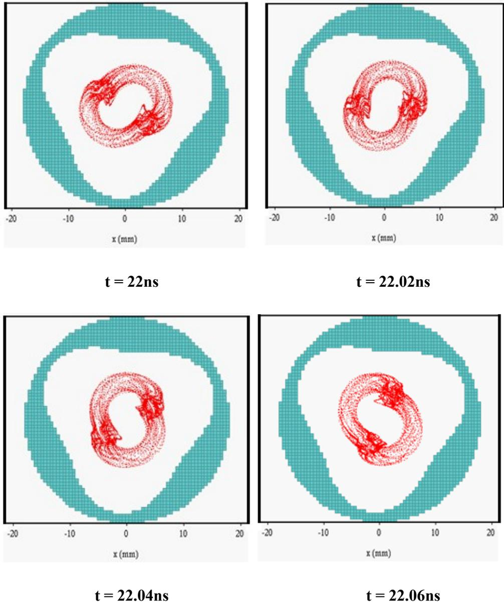
*Figure 4.3.3.5: Transverse phase-space plots depicting the evolution of the electron beam as a function of time, taken from MAGIC-3D. The axial window these plots were recorded in corresponds to  $1/10^{\text{th}}$  of the axial periodicity of the helical waveguide i.e. 3.75mm with the start position of this window at 84cm i.e. close to the end of the uniform helical waveguide section.*
