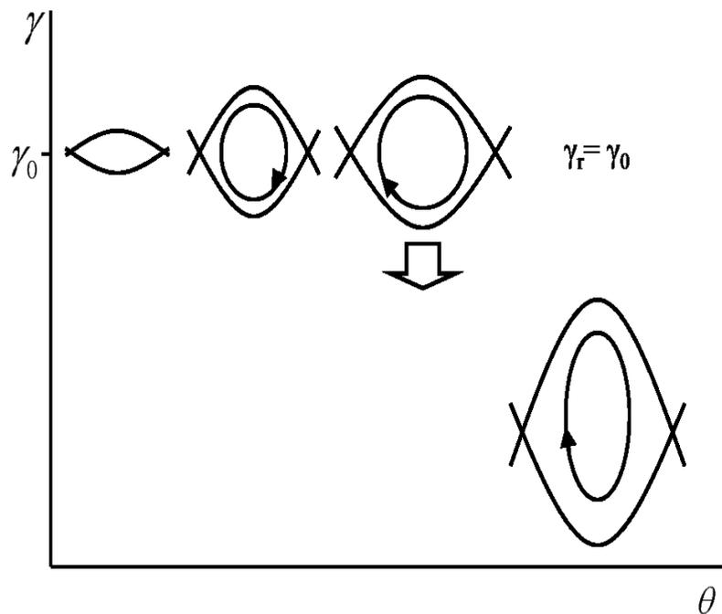
*Figure 2.5.5.1: Motion of separatrix with beam-wave resonance.*
