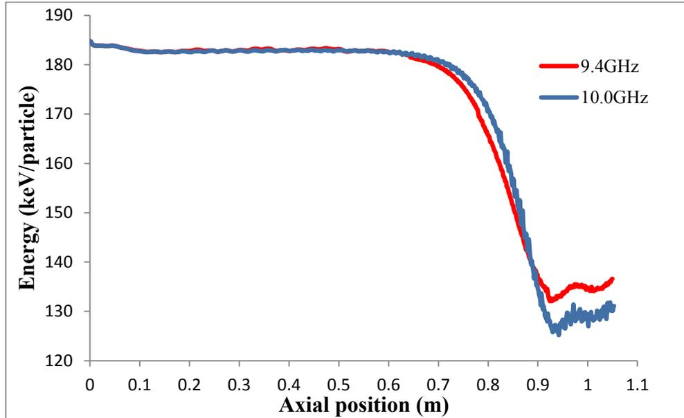
Figure 5.2.2.3: Predicted average kinetic energy of the beam electrons as a function of axial position for an input power of  $\sim 105\text{W}$  at  $9.4\text{GHz}$  and for an input power of  $\sim 30\text{W}$  at  $10.0\text{GHz}$ . These results are based on the original gyro-TWA geometry as detailed in chapter 4.
