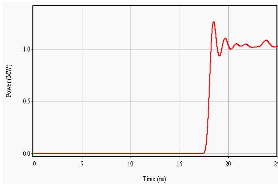
*Figure 4.3.6.3: Revised output power (particle equivalent power) for an input power of  $\sim 105\text{W}$  at 9.4GHz, taken from MAGIC-3D with the magnetic field spanning the axial range  $0\text{m}$  to  $\sim 0.91\text{m}$ .*
