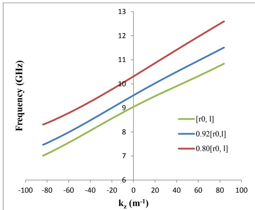
*Figure 5.3.1: Dispersion calculations for one period sections of helical waveguide with varying output mean radii and corrugation amplitudes, simulated in CST Microwave Studio. This plot highlights the frequency shift of the operating eigenwave for sections of helical waveguide with  $r_0$  and  $l$  decreasing from initial values of 14.1mm and 2.2mm respectively to  $\sim 80\%$  ( $\sim 0.80[r_0, l]$ ) and  $\sim 92\%$  ( $\sim 0.92[r_0, l]$ ) of these values.*
