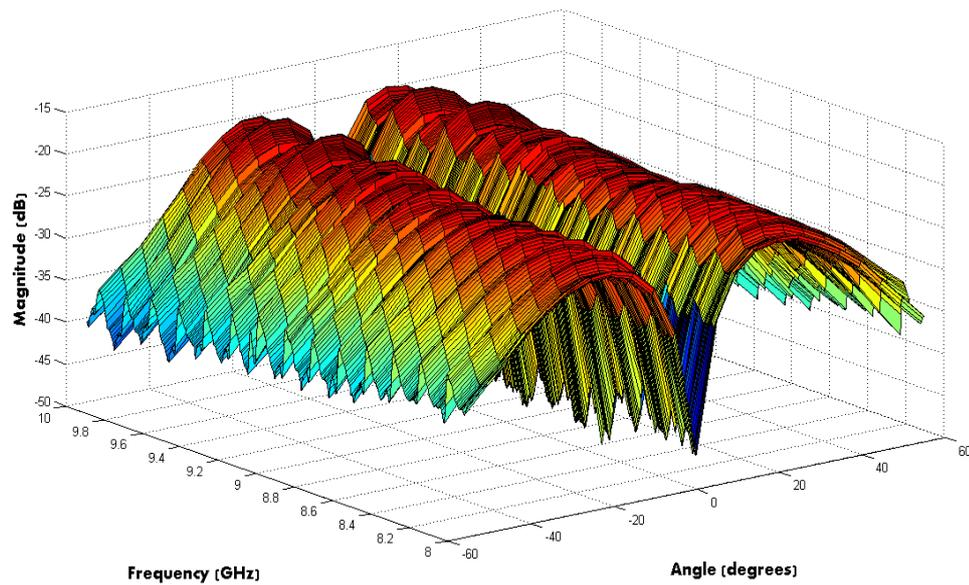
Figure 6.3.2: 3D plot of the far field azimuthal polarisation component across the entire frequency bandwidth, measured with the SNA.
