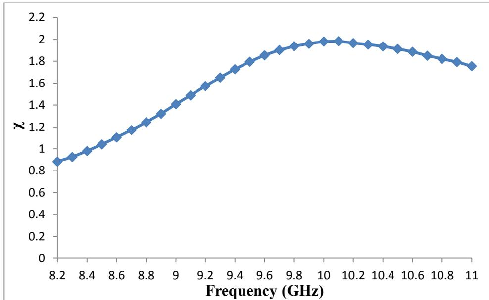
Figure 5.4.9: The content of the TE<sub>21</sub> mode,  $\chi$ , in the operating eigenwave as a function of frequency for a section of uniform helical waveguide with a mean radius and corrugation amplitude of  $r_0$  (14.1mm) and  $l$  (2.2mm).
