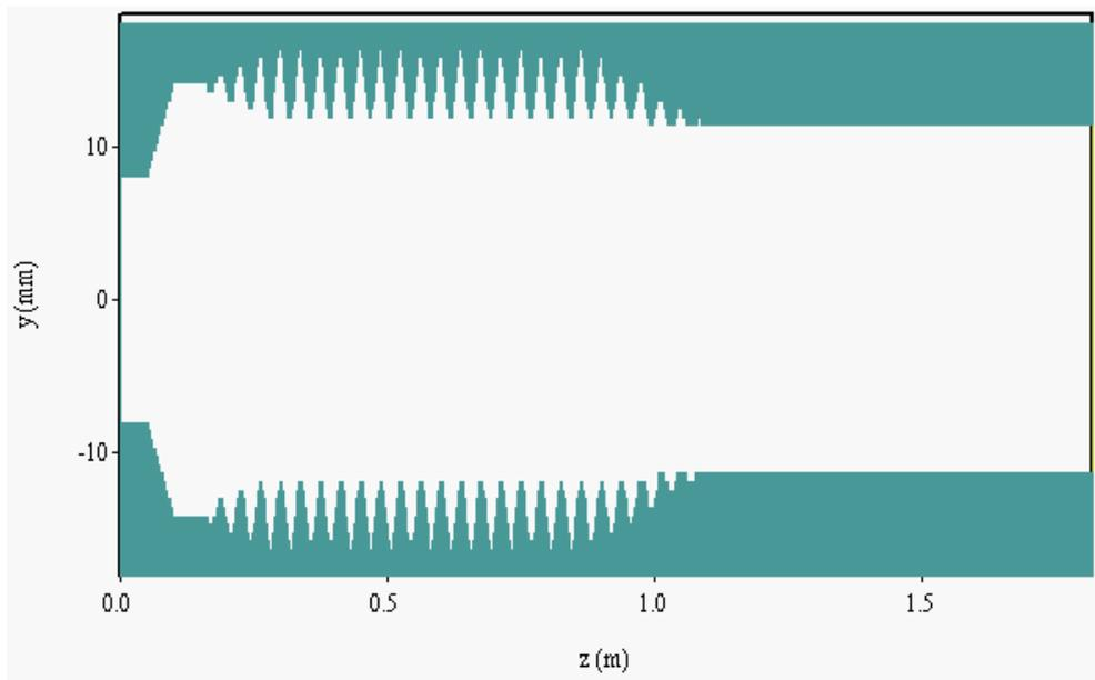
*Figure 5.7.1: Simulation geometry taken from MAGIC-3D showing a 26cm long tapered helical to cylindrical converter towards the output of the interaction region of the gyro-TWA with an output radius of  $\sim 0.80 \cdot r_0$ . In this geometry the uniform helical waveguide section measured 56cm in length.*
