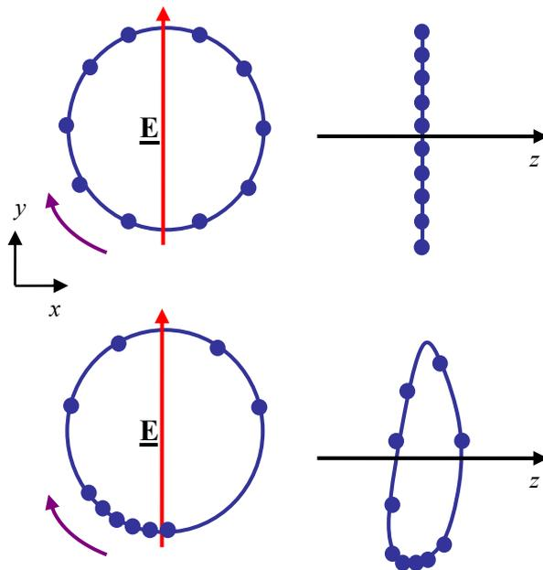
Figure 2.5.3.1: Axial electron movement associated with the Weibel instability.
