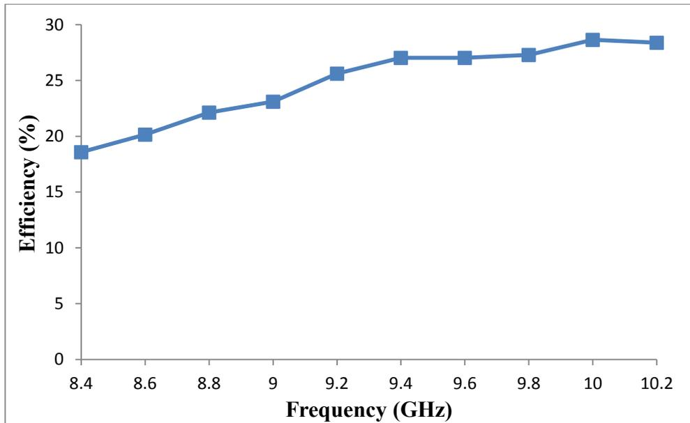
Figure 4.3.5.10: Predicted saturated efficiency of the simulated gyro-TWA as a function of frequency, with varying drive power at each frequency.
