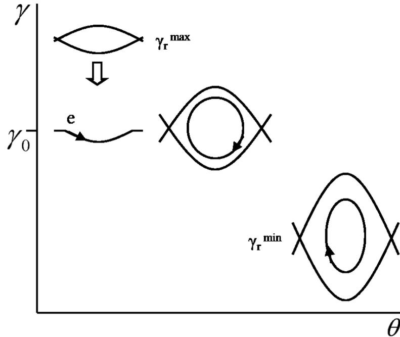
Figure 2.5.6.1: Separatrix motion with electron-wave resonance.
