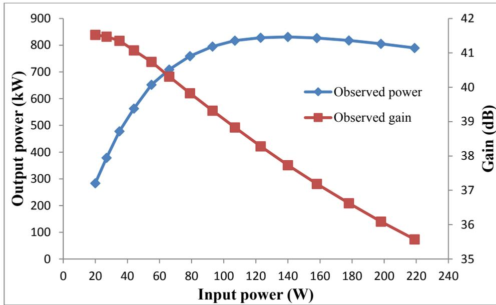
Figure 4.3.8.1: Observed power and gain as a function of input power for the simulated gyro-TWA with a helical interaction waveguide of axial period 39mm, with a magnetic field strength of  $\sim 0.2112T$  and an  $\alpha \sim 1.09$  at 9.4GHz.
