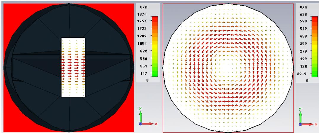
*Figure 6.2.4: Vector electric field distribution patterns (modes) at the input and output of the 9.0GHz Marie-type converter respectively, taken from CST Microwave Studio.*
