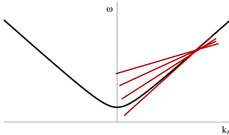
Figure 1.3.4: Generic dispersion diagram for a CARM showing autoresonance.
