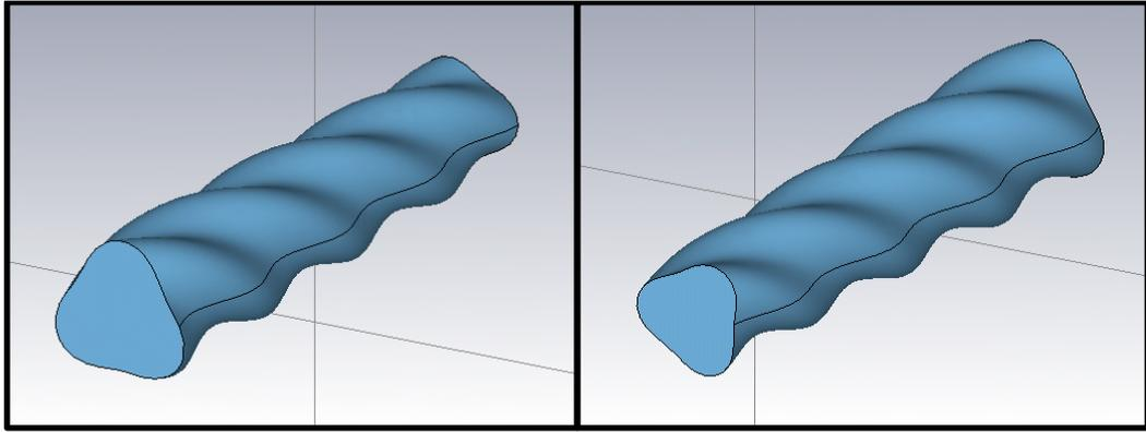
Figure 5.2.2.1: An example of a helical down taper and a helical up taper which maintain the ratio of  $l$  to  $r_0$  along the transition length, taken from CST Microwave Studio. The down taper has an initial mean radius and corrugation amplitude of  $r_0$  and  $l$  respectively with a final mean radius and corrugation amplitude of  $\sim 0.80 \cdot r_0$  and  $\sim 0.80 \cdot l$  respectively. The up taper is the inverse of the down taper.
