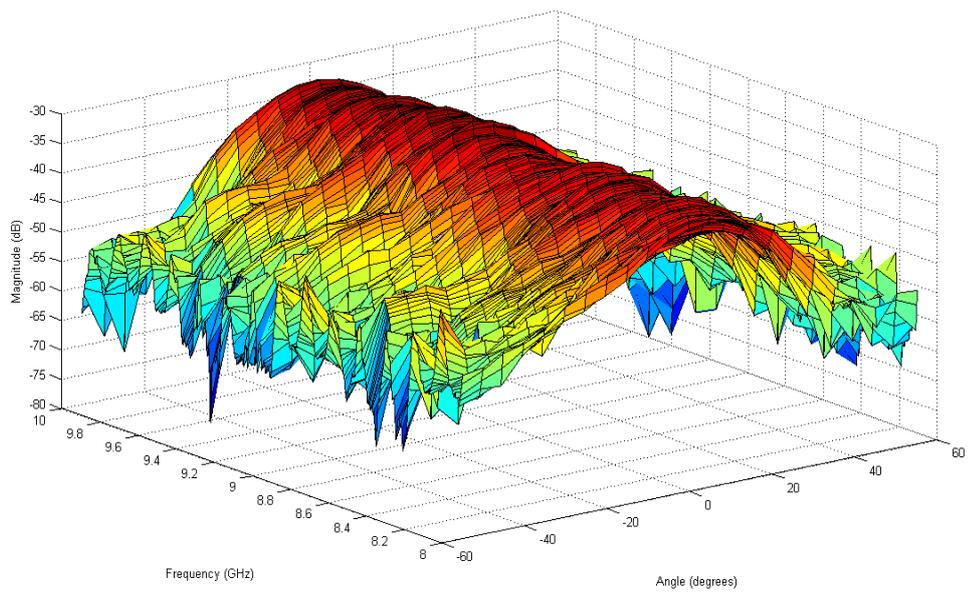
Figure 6.4.5: 3D plot of the radial polarisation component with the mesh present, measured with an SNA over the entire optimised 2.0GHz frequency bandwidth of the converter.
