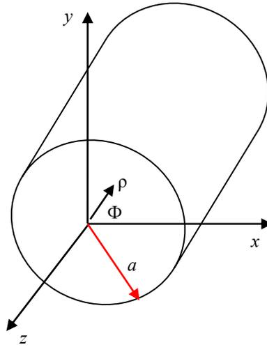
Figure 2.3.4.1: Cylindrical waveguide geometry.
