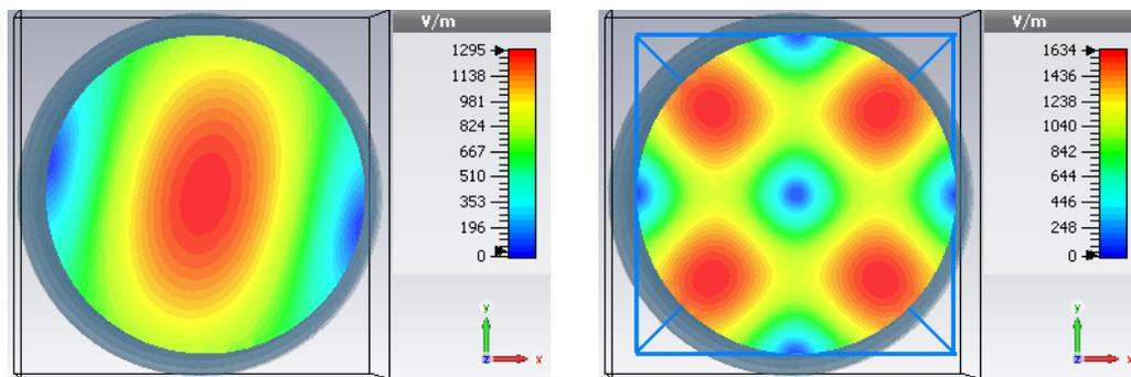
*Figure 5.4.3: Example of a cylindrical  $TE_{11}$  mode and a  $TE_{21}$  mode, taken from CST Microwave Studio.*
