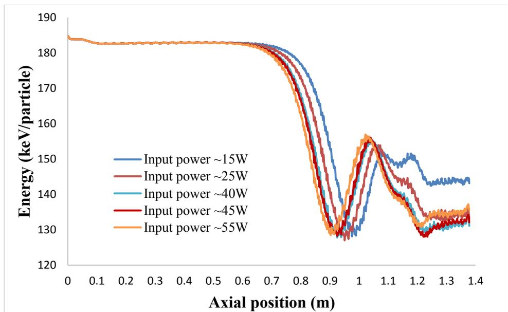
*Figure 5.5.1.1: Predicted average kinetic energy of the beam electrons as a function of axial position and input power at 10.0GHz, for a gyro-TWA including a helical down taper of length 40cm to an output mean radius and corrugation amplitude of  $\sim 0.90[r_0, l]$ . Here the uniform helical waveguide section measured 52cm in length.*
