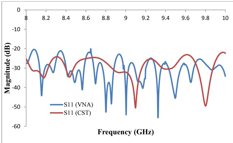
Figure 6.3.1: Plot showing the forward reflection coefficient ( $S_{11}$ ) measured with the VNA alongside that predicted by CST Microwave Studio for the 9.0GHz Marie-type converter.
