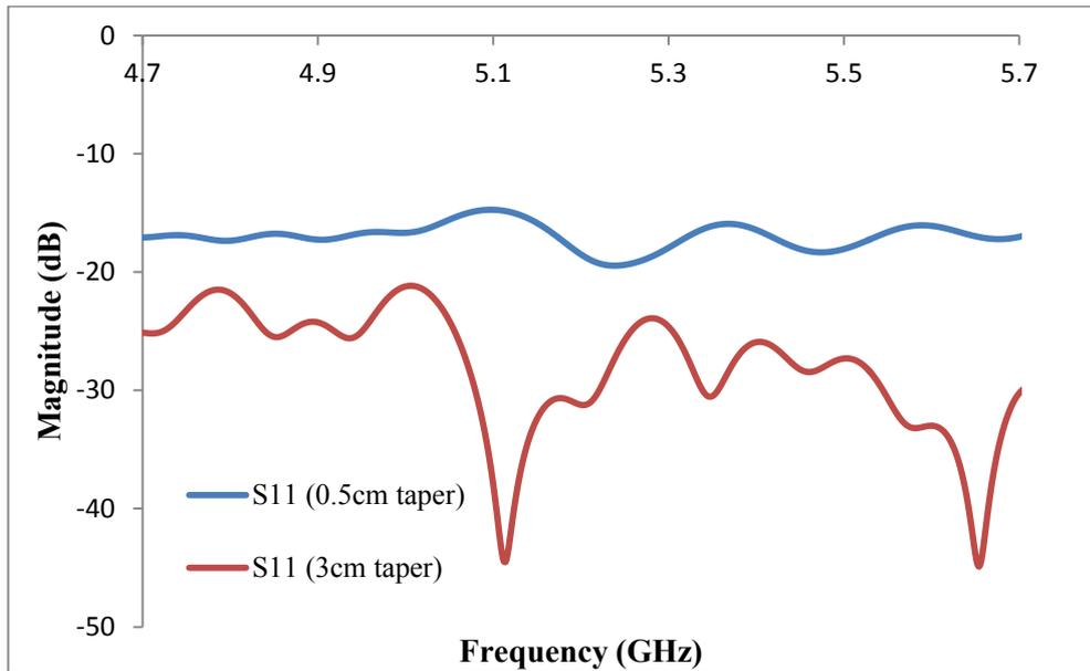
*Figure 6.2.3: S-parameter plots for the 5.2GHz Marie-type converter with a 0.5cm taper and a 3cm taper transition between the output of section 1 and the input of section 2.*
