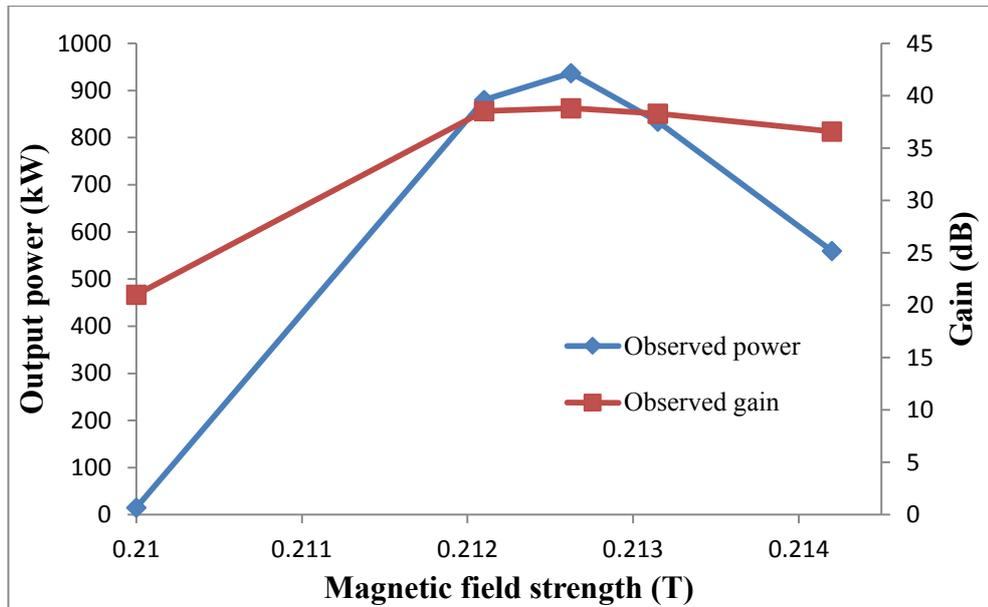
Figure 4.3.5.1: Observed power and gain of the simulated gyro-TWA for varying magnetic field strengths, with an  $\alpha$  of 1.2 at 9.4GHz.
