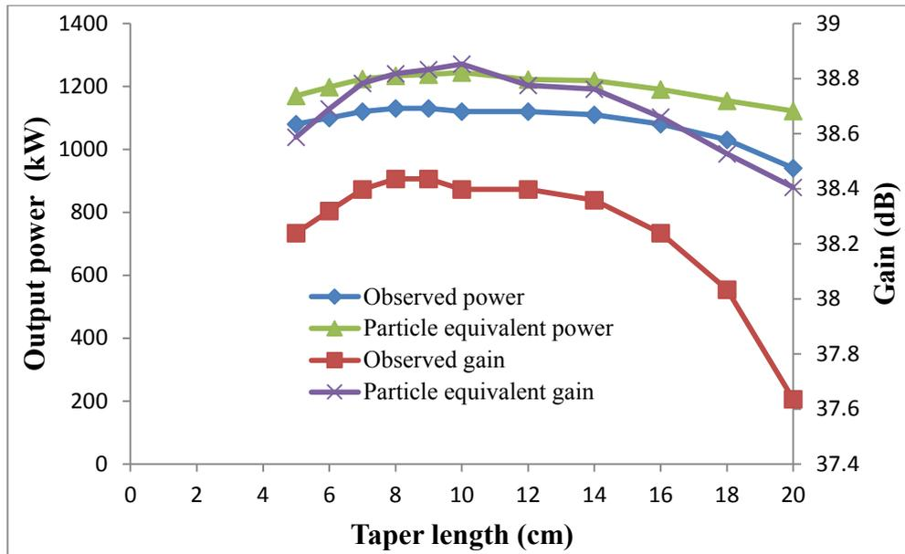
Figure 5.5.2.3: Observed power/gain and particle equivalent power/gain as a function of taper length for a gyro-TWA including a helical down taper with an output mean radius and corrugation amplitude of  $\sim 0.78[r_0, l]$ , taken at 10.0GHz for a drive power of  $\sim 160W$ .
