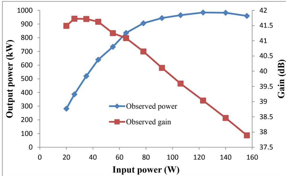
*Figure 4.3.8.2: Observed power and gain as a function of input power for the simulated gyro-TWA with a helical interaction waveguide of axial period  $36\text{mm}$ , with a magnetic field strength of  $\sim 0.2149\text{T}$  and an  $\alpha \sim 1.27$  at  $9.4\text{GHz}$ .*
