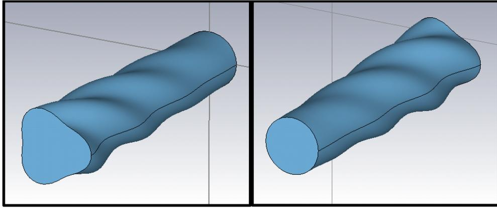
*Figure 5.2.2.2: An example of a helical to cylindrical converter and a cylindrical to helical converter taken from CST Microwave Studio. The helical to cylindrical converter has an initial mean radius and corrugation amplitude of  $r_0$  and  $l$  respectively with a final mean radius and corrugation amplitude of  $\sim 0.80 \cdot r_0$  and  $0$  respectively. The cylindrical to helical converter is the inverse of the helical to cylindrical converter.*
