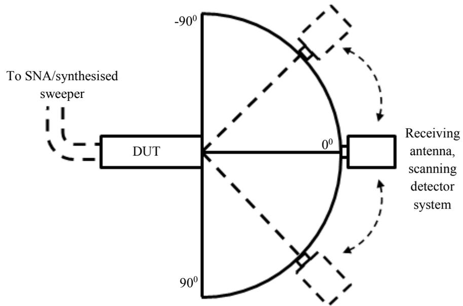
Figure 3.5.1: Scanning apparatus set up. Here the DUT was the Marie-type converter.
