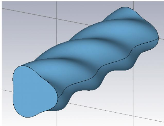
Figure 2.3.6.1: Inner 3-fold helical waveguide geometry, taken from CST Microwave Studio.
