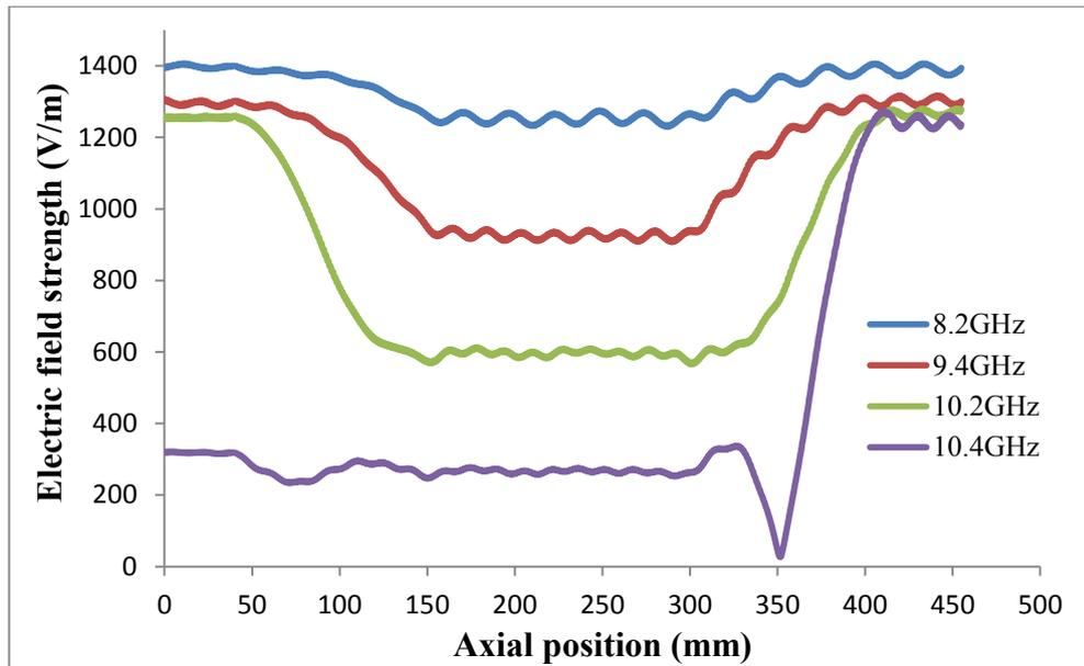
Figure 5.4.7: Absolute electric field strength monitored axially through the centre of the helical structure which did not include helical tapers (figure 5.4.1) for varying drive frequencies.
