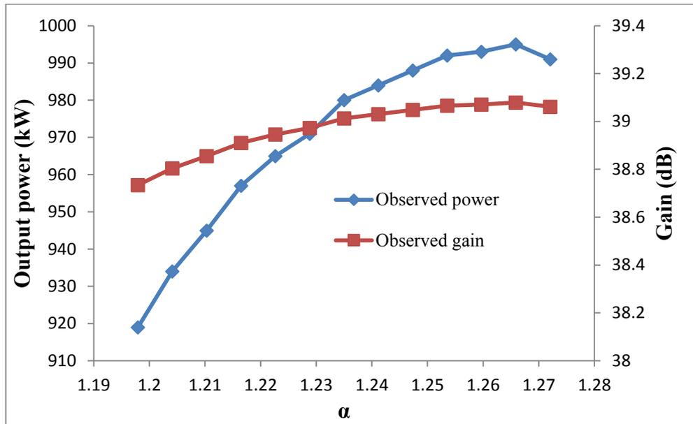
Figure 4.3.5.5: Observed power and gain of the simulated gyro-TWA for varying  $\alpha$ , with a magnetic field strength of  $\sim 0.2123T$  at  $9.4GHz$ .
