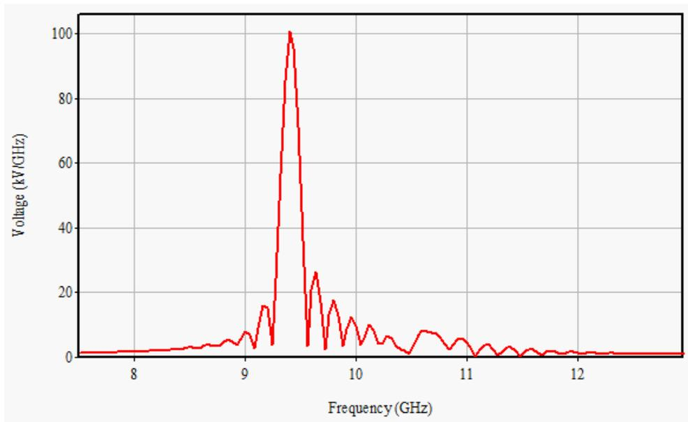
*Figure 4.3.3.2: FFT showing the gyro-TWA operating at the desired frequency, in this instance 9.4GHz, taken from MAGIC-3D.*
