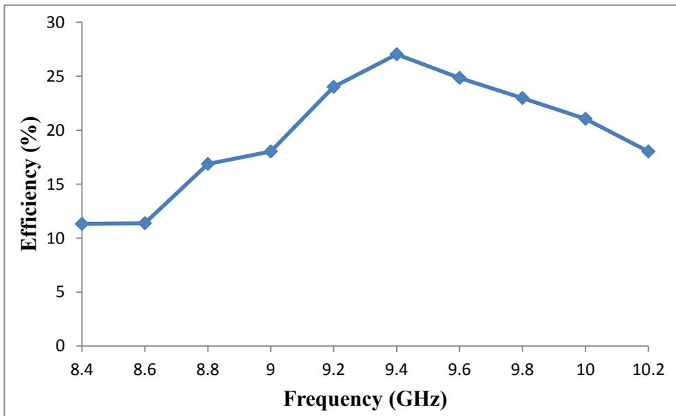
Figure 4.3.5.8: Predicted efficiency of the gyro-TWA as a function of frequency for input powers of  $\sim 105W$  to  $\sim 110W$  with a magnetic field strength and an  $\alpha$  of  $\sim 0.2123T$  and  $\sim 1.27$  respectively.
