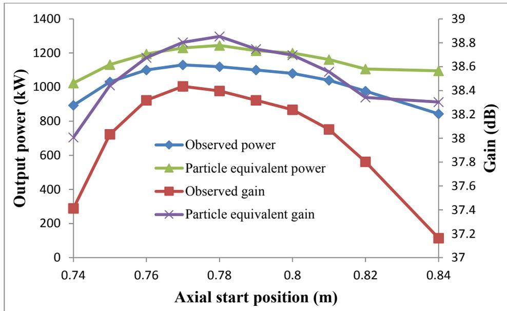
Figure 5.5.2.4: Observed power/gain and particle equivalent power/gain as a function of taper start position for a gyro-TWA including a helical down taper of length 10cm to an output mean radius and corrugation amplitude of  $\sim 0.78[r_0, l]$ , taken at 10.0GHz for a drive power of  $\sim 160W$ .
