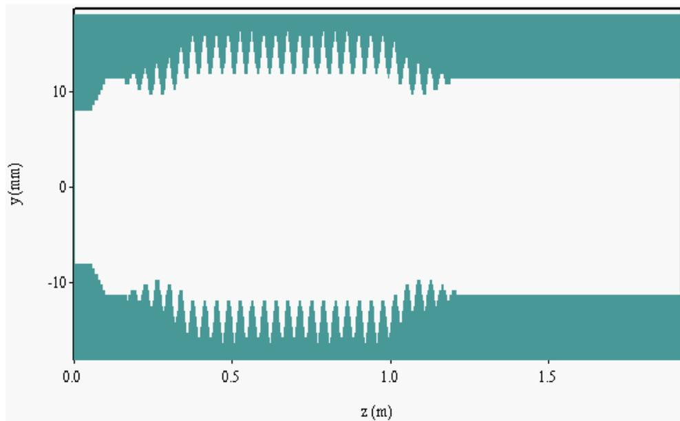
Figure 5.6.1: A gyro-TWA geometry with a 14cm long helical up taper with an initial mean radius and corrugation amplitude of  $0.80[r_0, l]$  to final values of  $[r_0, l]$ , taken from MAGIC-3D. The up taper is the inverse of the helical down taper which features towards the output of the interaction region of the amplifier. This geometry is primarily that of figure 5.2.2.5, but with the addition of a helical up taper positioned immediately before the uniform helical waveguide section.
