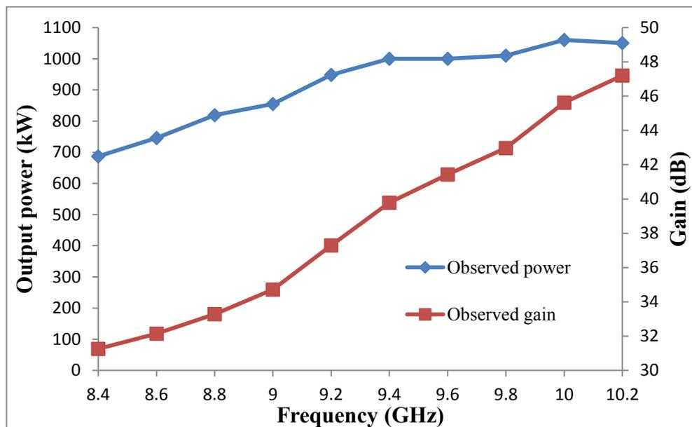
*Figure 4.3.5.9: Maximum observed power and saturated gain of the simulated gyro-TWA as a function of frequency, with varying drive power at each frequency.*
