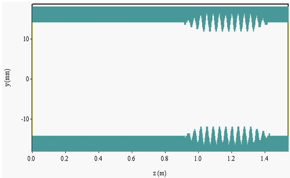
*Figure 4.4.3: Simulation geometry including a 30cm long helically corrugated waveguide section used to calculate the dispersion of the helix.*
