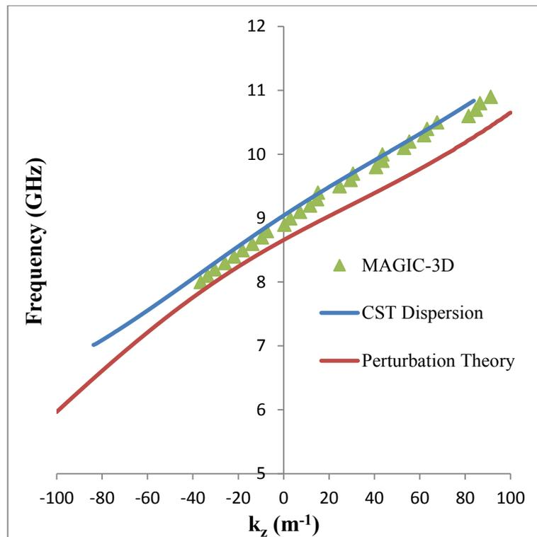
Figure 4.4.8: Dispersion calculation from CST Microwave Studio plotted alongside the dispersion predictions from perturbation theory and MAGIC-3D.
