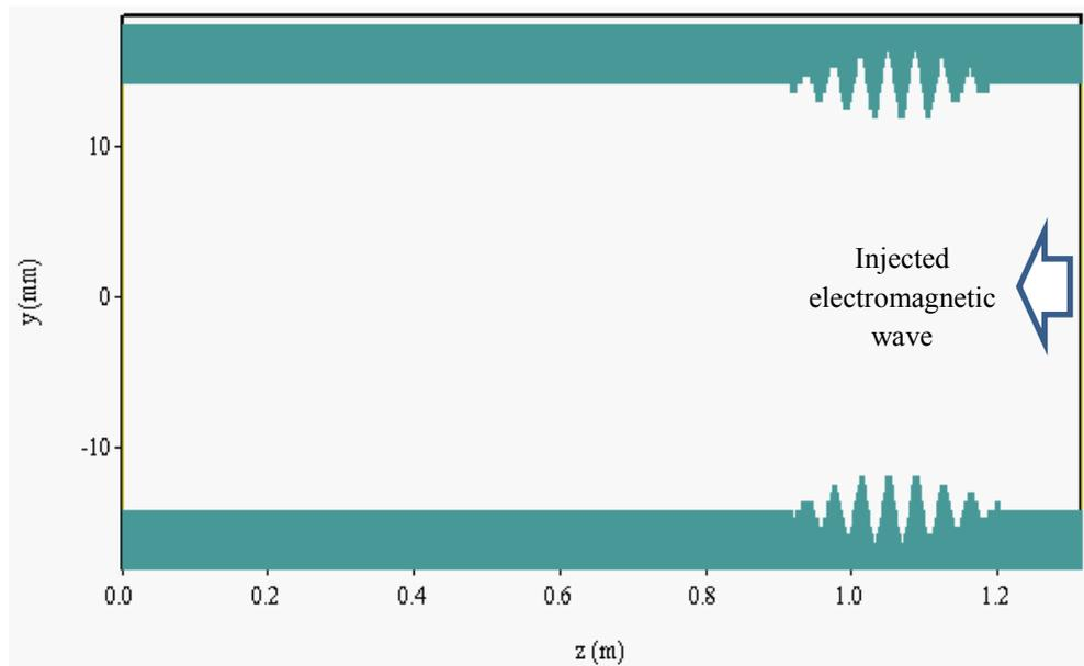
Figure 4.4.1: Simulation geometry including a 7.5cm long helically corrugated waveguide section used to calculate the dispersion of the helix.
