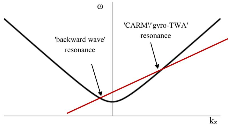
Figure 1.3.5: Generic dispersion diagram for a gyro-BWO.
