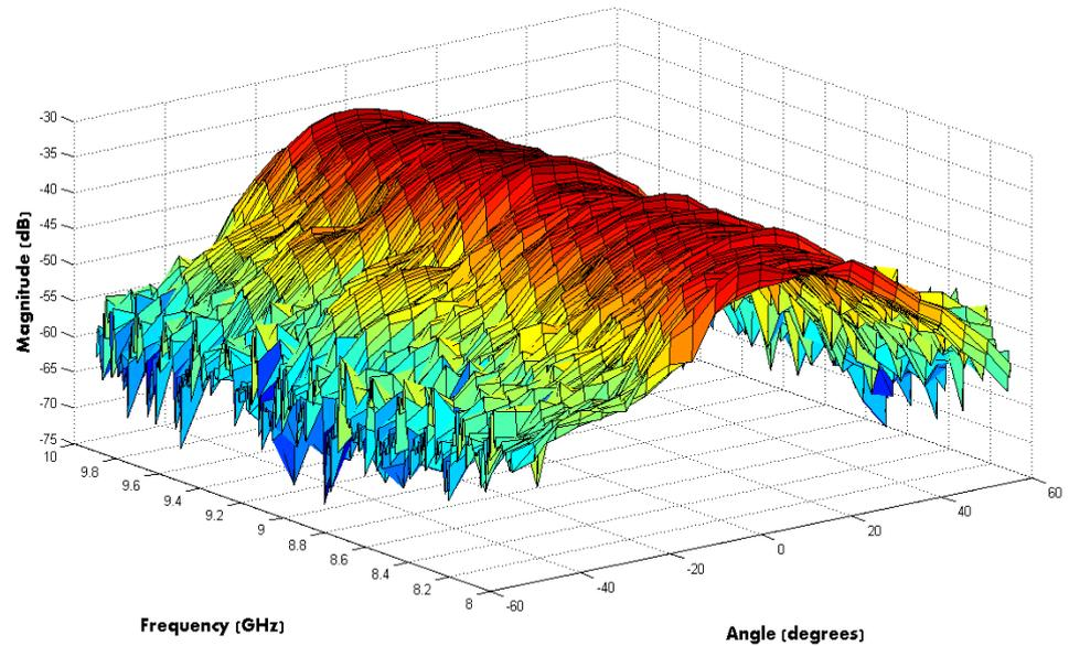
Figure 6.3.3: 3D plot of the far field radial polarisation component across the entire frequency bandwidth, measured with the SNA.
