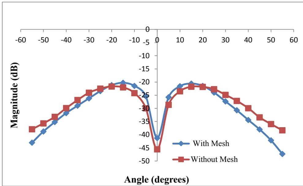
Figure 6.4.2: Comparison of the azimuthal polarisation component of the electric field distribution at 9.0GHz centre frequency, with and without the plasma confinement mesh.
