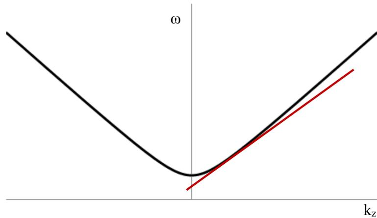
*Figure 1.3.2: Generic dispersion diagram for a gyro-TWT.*
