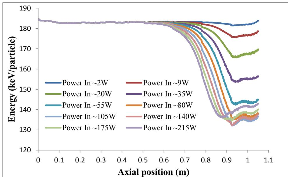
Figure 4.3.6.1: Predicted average kinetic energy of the beam electrons in the simulated gyro-TWA as a function of axial position and drive power, taken at 9.4GHz.
