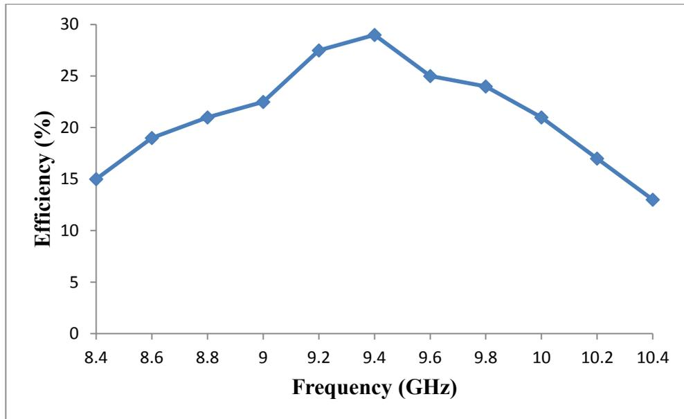
Figure 4.2.2.3: Measured saturated efficiency as a function of frequency for the experimental X-band 2<sup>nd</sup> harmonic gyro-TWA [Bratman, 2000].
