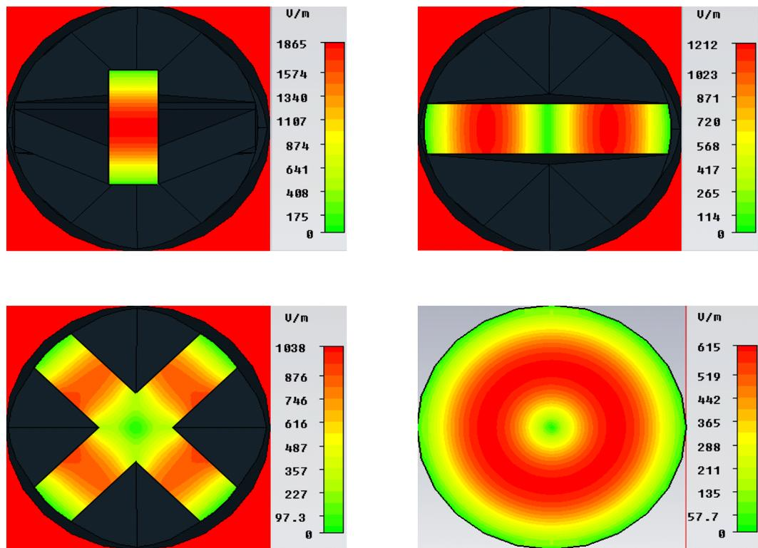
Figure 6.2.6: Mode patterns at the input and output for each main section of the Marie-type converter with operating centre frequency of 9.0GHz.
