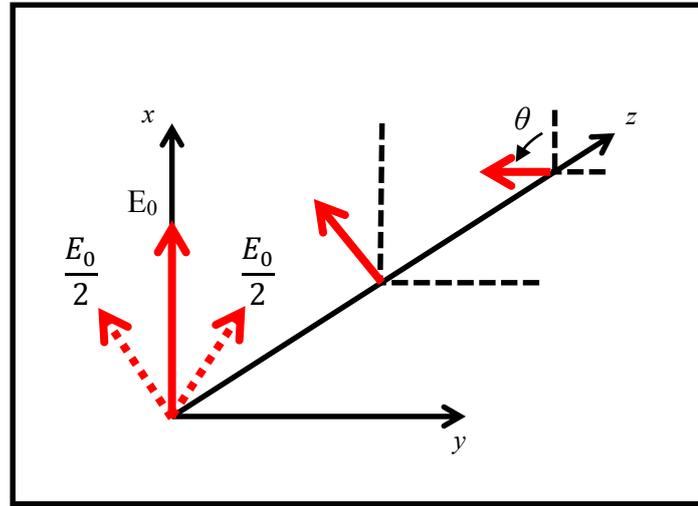
*Figure 3.6.1: Illustration of linearly polarised wave rotation.*
