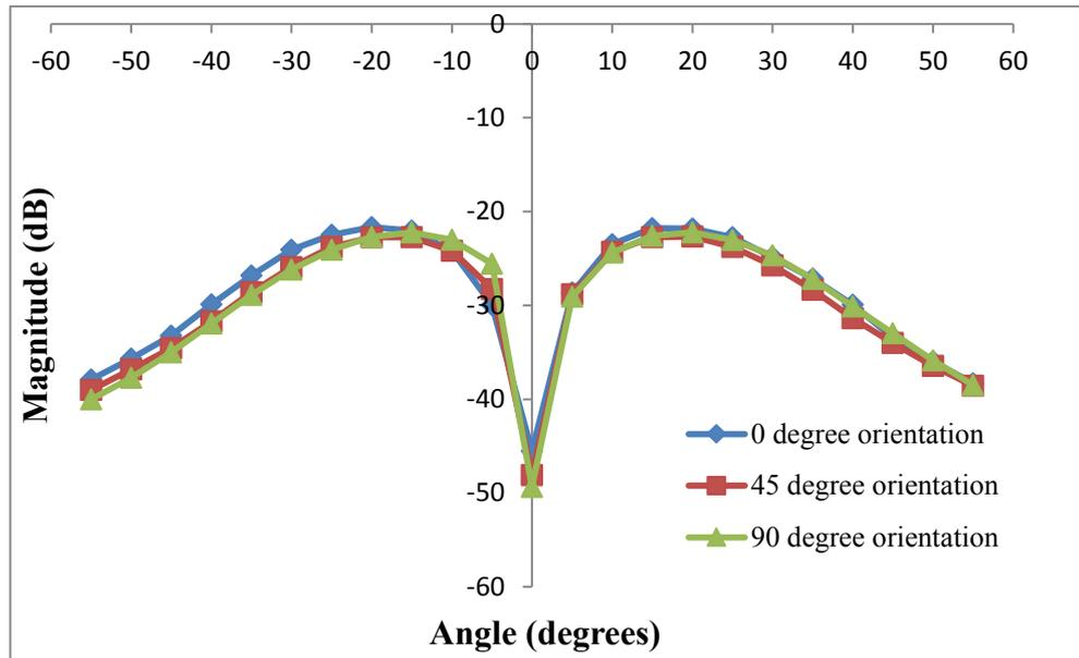
Figure 6.3.4: Azimuthal polarisation component of the electric field distribution at the centre frequency of 9.0GHz, with the Marie-type converter at 0°, 45° and 90° orientations.
